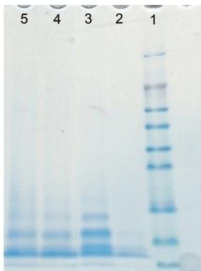
**Fig. S14** SDS-PAGE images for visible observing the inhibition effect of F-SLOH. Lane 1, the molecular weight markers; Lane 2, HFIP-treated monomeric  $A\beta_{1-42}$ ; Lane 3, oligomeric  $A\beta_{1-42}$  by incubating monomer at 4 °C for 24 h; Lane 4 and 5, in the presence of F-SLOH, at 1:1 and 5:1 molar ratio of F-SLOH to monomers, respectively.
