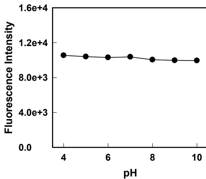
**Fig. S7** The effect of pH on the fluorescence property of F-SLOH (1.0 μM).
