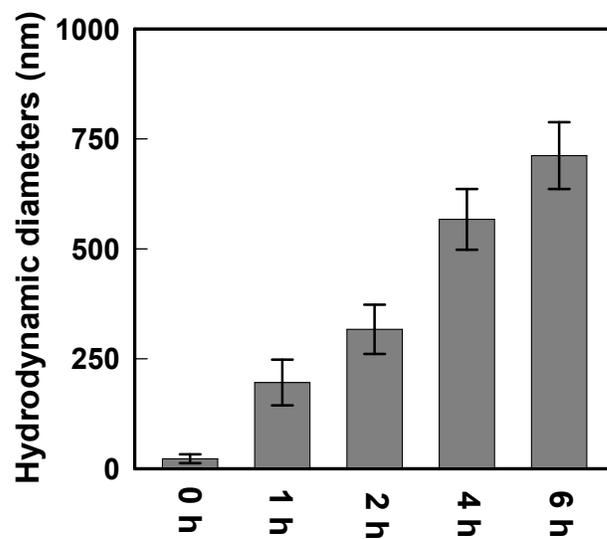
**Fig. S9** Hydrodynamic diameters of  $A\beta$  during the growth process as measured by DLS.
