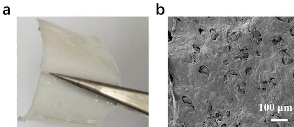
**Fig. S6.** Photo image (a) and SEM image (b) of methylcellulose modified PVA membrane.
