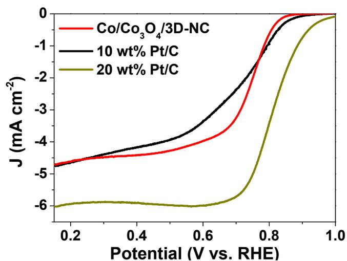
**Fig. S4.** Comparison of ORR polarization curves of Co/Co<sub>3</sub>O<sub>4</sub>/3D-NC with commercial 10 wt.% and 20 wt.% Pt/C.
