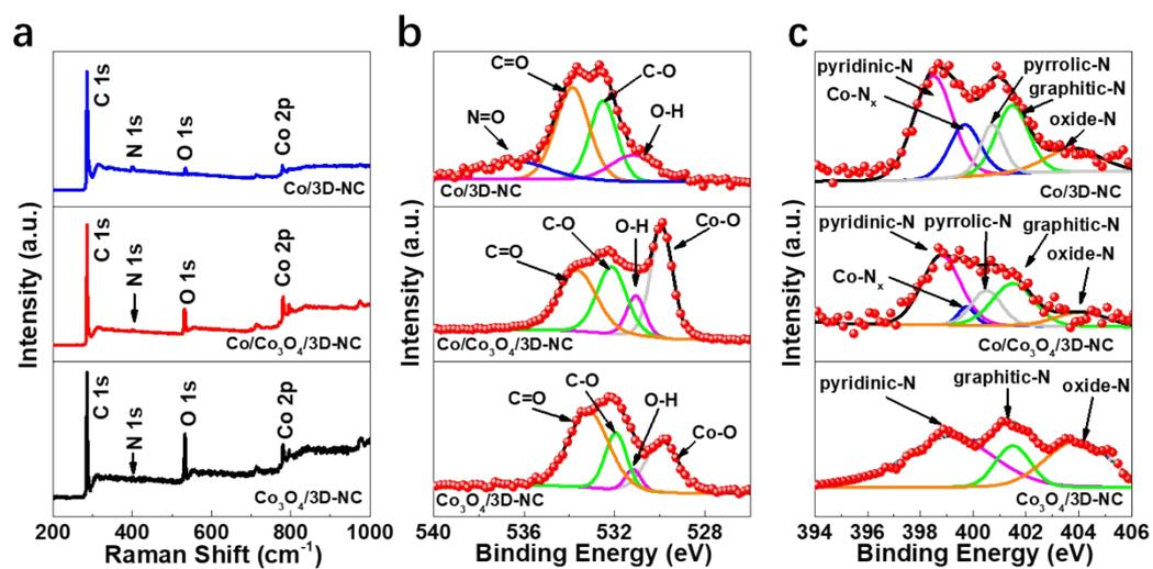
**Fig. S3.** (a) XPS survey spectra, high-resolution (b) O 1s and (c) N 1s XPS spectra of Co/3D-NC, Co/Co<sub>3</sub>O<sub>4</sub>/3D-NC and Co<sub>3</sub>O<sub>4</sub>/3D-NC.
