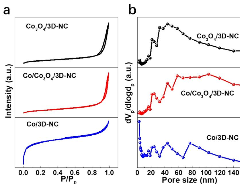
**Fig. S2.** (a)  $N_2$  adsorption-desorption isotherms and (b) Pore size distribution curves of Co/3D-NC, Co/Co<sub>3</sub>O<sub>4</sub>/3D-NC and Co<sub>3</sub>O<sub>4</sub>/3D-NC.
