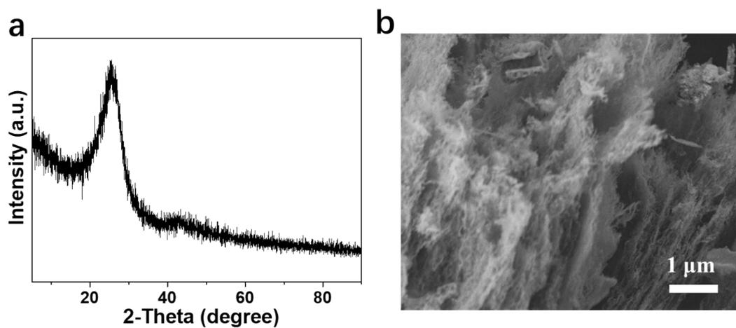
**Fig. S1.** (a) XRD spectrum and (b) SEM image of 3D-NC. The XRD pattern displays a diffraction peak at  $26.1^\circ$ , which matches well with the graphitic carbon phase (JCPDS No. 41-1487).
