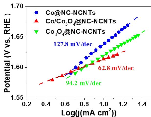
**Fig. S5.** The Tafel slop of Co/3D-NC, Co/Co<sub>3</sub>O<sub>4</sub>/3D-NC and Co<sub>3</sub>O<sub>4</sub>/3D-NC for OER process.
