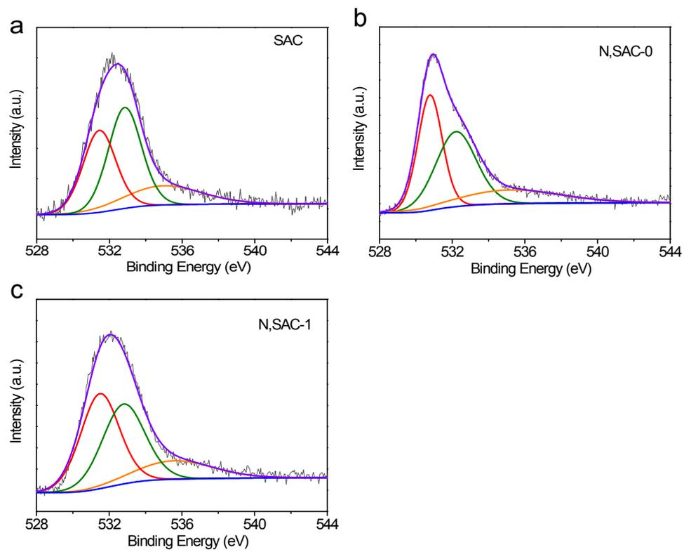
**Figure S6.** The high-resolution XPS O1s spectra of (a) SAC, (b) N,SAC-0, and (c) N,SAC-1.
