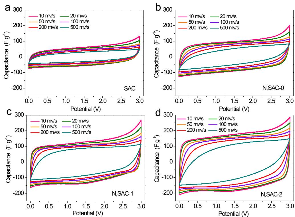
**Figure S8.** The CV curves of all the specimens for different scan rates in ionic liquid electrolyte.
