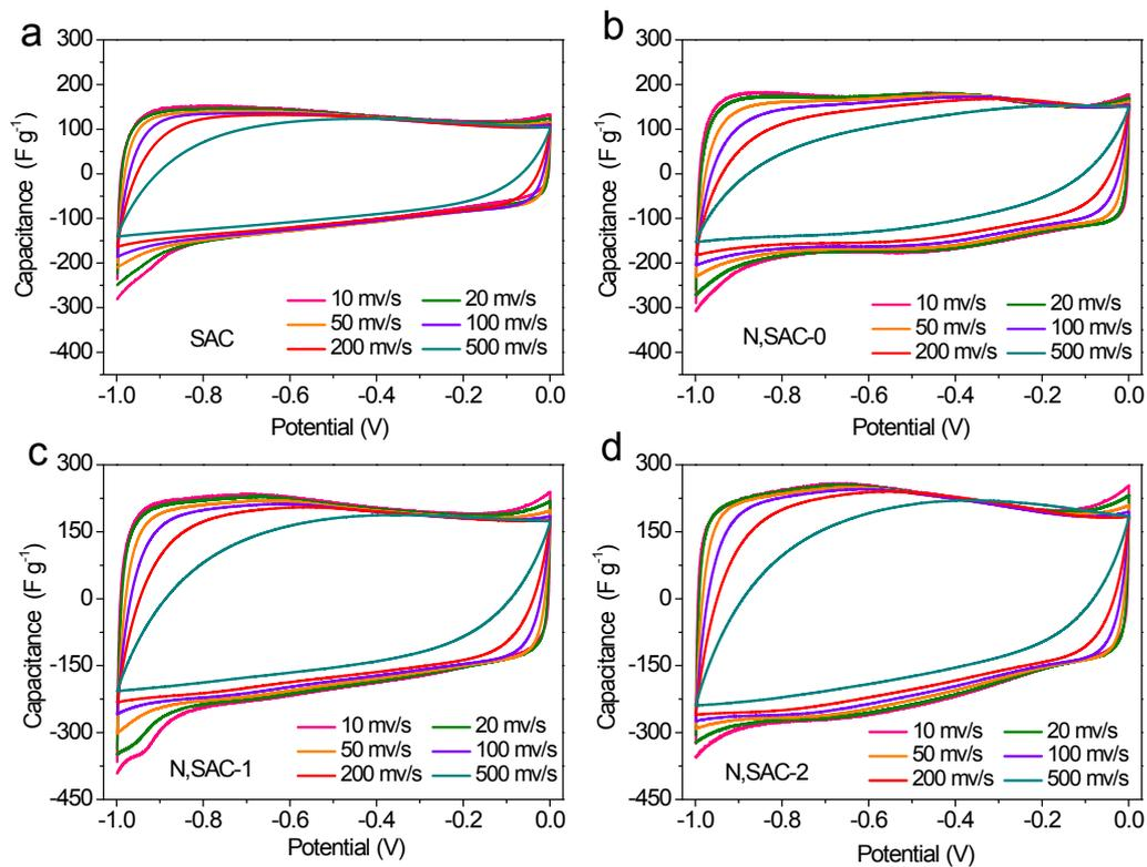
**Figure S7.** The CV curves of all the specimens for different scan rates in 2M KOH electrolyte.
