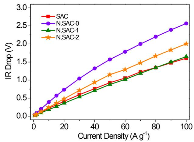
**Figure S10.** Potential IR drop vs. current density in ionic liquid electrolyte.
