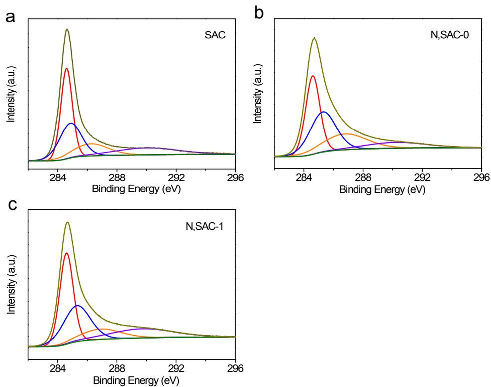
**Figure S4.** The high-resolution XPS C1s spectra of (a) SAC, (b) N,SAC-0, and (c) N,SAC-1.
