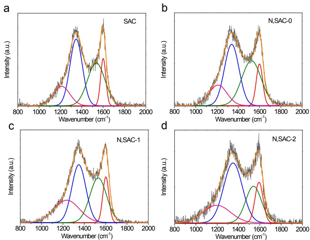
**Figure S2.** The fitted Raman spectra of all carbon specimens by using Voigt function.
