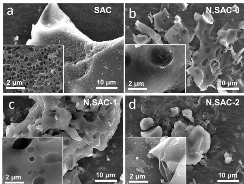
**Figure S1.** SEM micrographs of sodium alginate derived carbons: (a) SAC, (b) N,SAC-0, (c) N,SAC-1, and (d) N,SAC-2.
