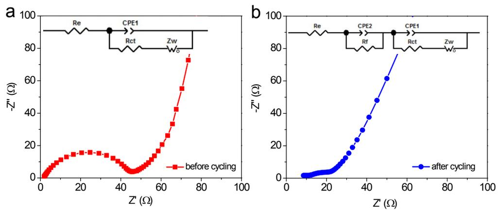
**Figure S13.** The Nyquist plots for N,SAC-2 (a) before cycling and (b) after 500 cycles.
