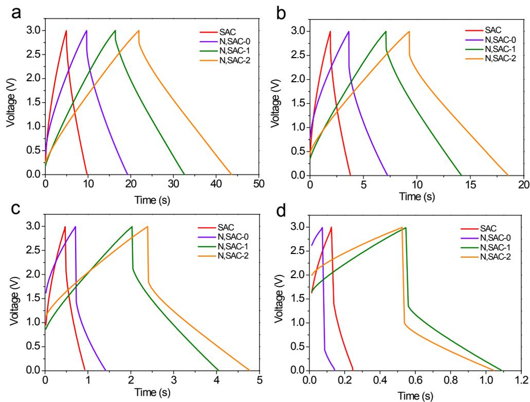
**Figure S9.** The galvanostatic charge-discharge curves of all samples measured at 10, 20, 50, and 100 A g<sup>-1</sup> in ionic liquid electrolyte.
