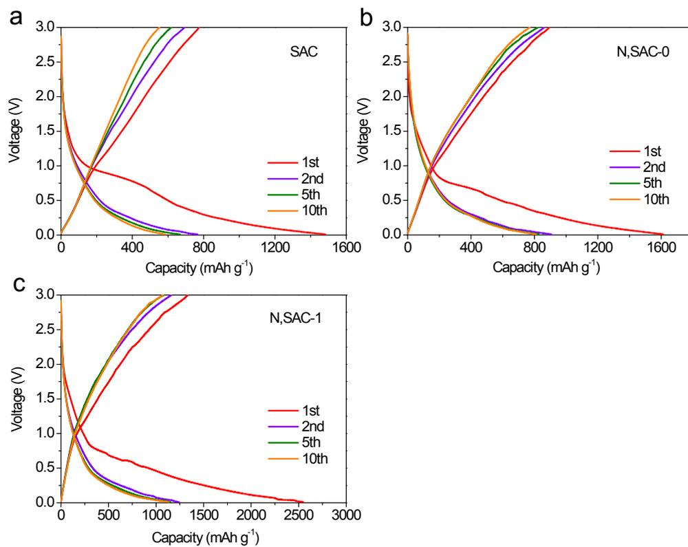
**Figure S12.** The galvanostatic charge-discharge curves of (a) SAC, (b) N,SAC-0, and (c) N,SAC-1 for lithium ion batteries.
