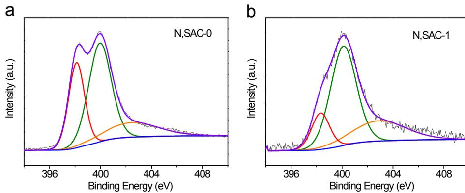
**Figure S5.** The high-resolution XPS N1s spectra of (a) N,SAC-0, and (b) N,SAC-1.
