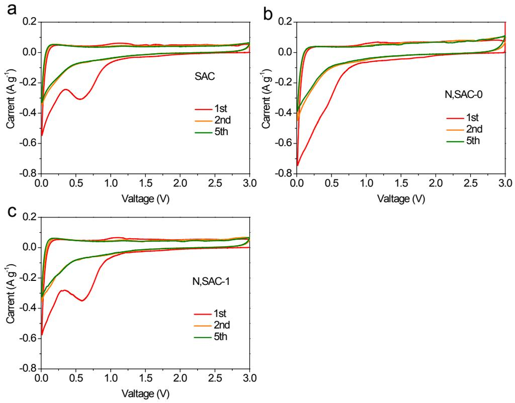
**Figure S11.** The CV curves of (a) SAC, (b) N,SAC-0, and (c) N,SAC-1 for lithium ion batteries.
