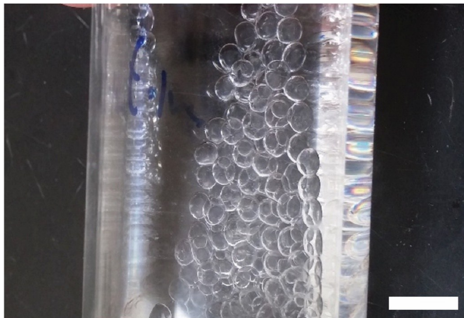
Figure S2. (a) Stable millimeter size CNF composite microcapsules suspended in toluene. The capsules are prepared by dripping an aqueous solution of 0.16 wt% CNF into a toluene solution containing 0.3 wt% MADQUAT-co-BTA. Scale bar is 10 mm.
