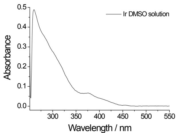
**Figure S3** UV-Vis absorption spectra of complex **Ir** in DMSO solution with the concentration of  $10^{-5}$  M.
