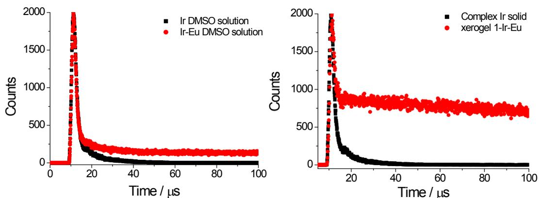
**Figure S4** Lifetime decay profiles of **Ir** and **Ir-Eu** in DMSO solution and solid state. ( $\lambda_{ex} = 370$  nm, monitored at 494 nm for **Ir** DMSO solution and solid state, monitored at 613 nm for **Ir-Eu** DMSO solution and xerogel **Ir-Eu** solid)
