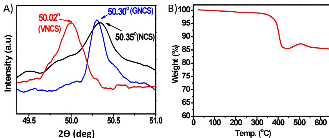
Figure S 1. A) XRD shift of plane (511), B) TGA of VNCS
