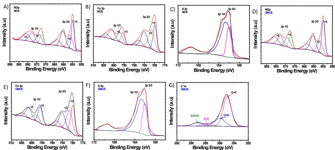
Figure S3. XPS results, A-C) Ni 2p, Co 2p and S2p XPS spectra, respectively for NCS sample, and D-G) Ni 2p, Co 2p, S2p and C 1s XPS spectra, respectively for GNCS
