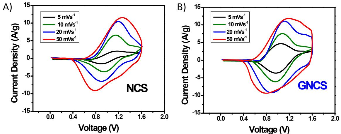
Figure S 9 CV test at different scan rates of A) NCS samples, and B) GNCS sample
