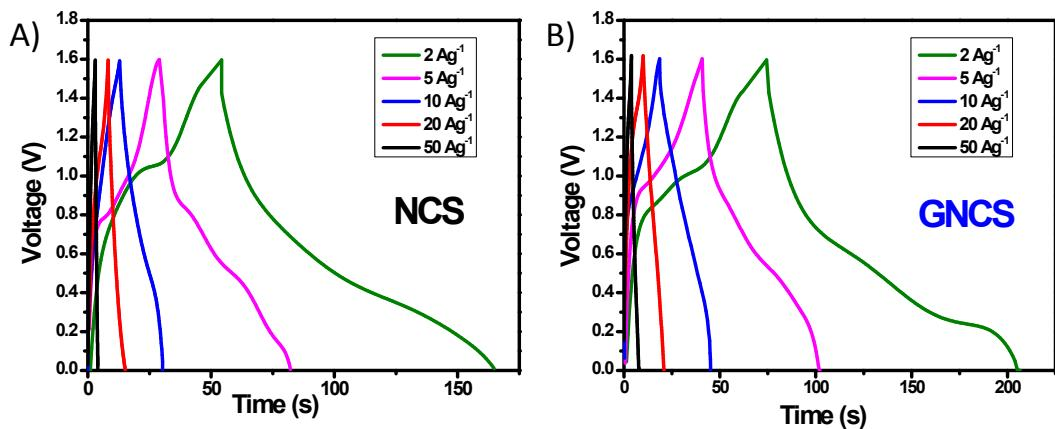
Figure S 10 Charge-Discharge at different current densities of A) P HSC, and B) G HSC
