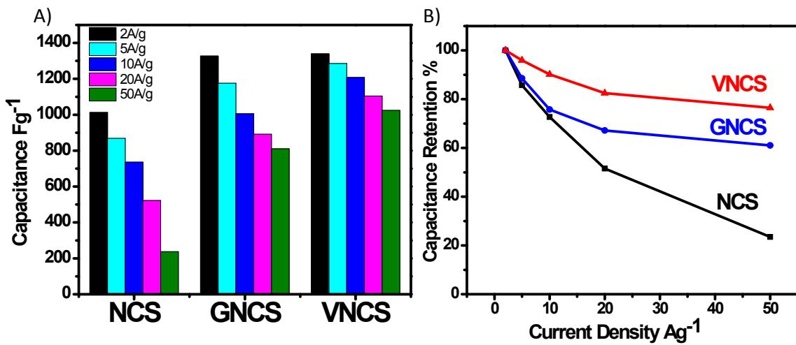
Figure S6. A) Specific capacitance values of all samples at different current rates, and B) Capacitance retention of all samples at all current densities.
