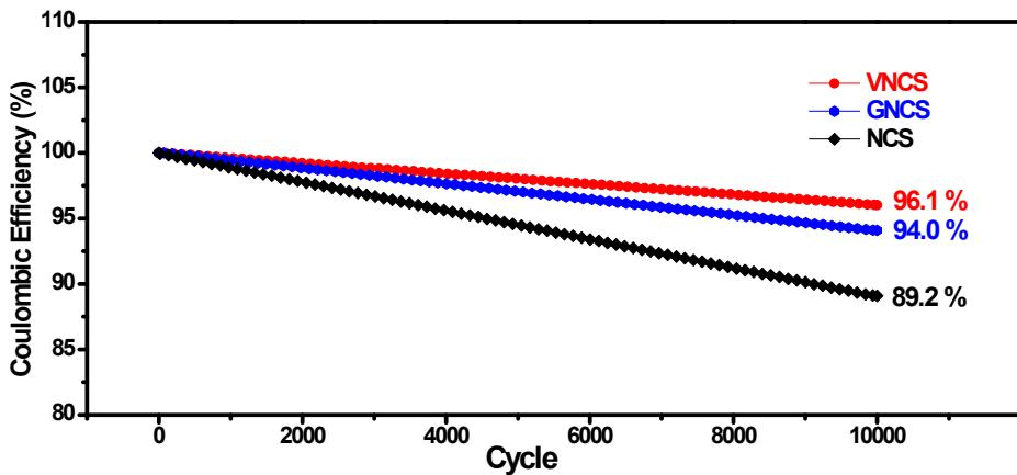
Figure S7. Columbic efficiency throughout the testing cycles
