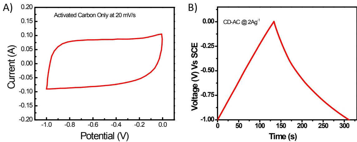
Figure S 8 A) CV, and B) Charge-discharge tests of tests of AC/G electrode
