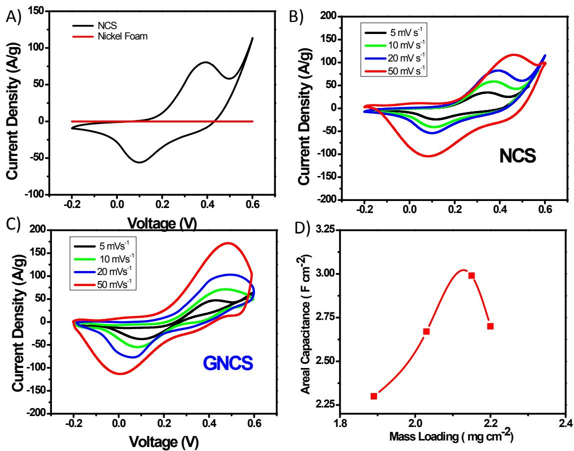
Figure S4. A) CV test of the nickel foam compared to NCS, B-C) CV test of NCS and GNCS at different scan rates, and D) Areal capacitance variation with mass loading of VNCS
