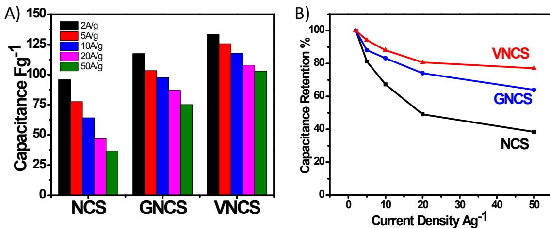
Figure S 11. A) Capacitance values of all samples at different current densities, and B) Capacitance retention of all samples compared to the capacitance value of each sample at  $2 \text{ Ag}^{-1}$
