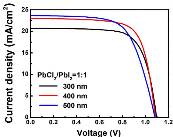
**Fig. S2**  $J$ - $V$  curves of devices with different thickness of perovskite absorption layer.
