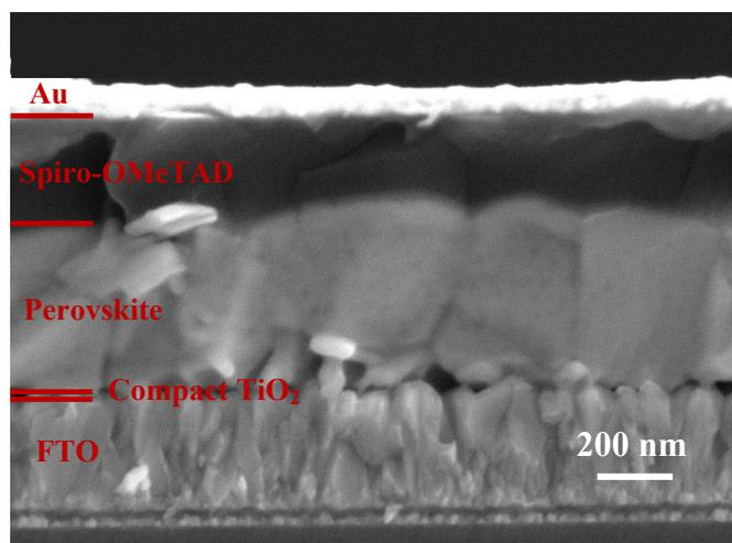
**Fig. S5** Typical cross-sectional SEM image of device.
