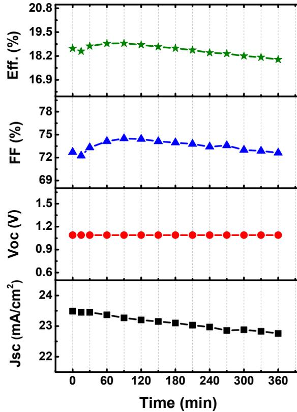
**Fig. S6** Device parameters evolution under continuous AM 1.5G light illumination.
