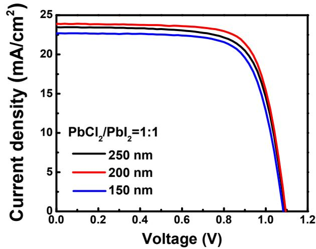
**Fig. S3**  $J$ - $V$  curves of devices with different thickness of Spiro-OMeTAD.
