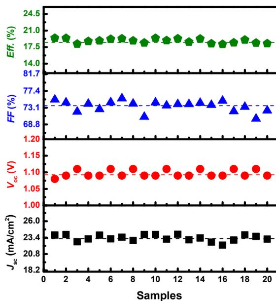
**Fig. S4** Statistical distributions of the device parameters obtained in 20 devices fabricated with optimized conditions.
