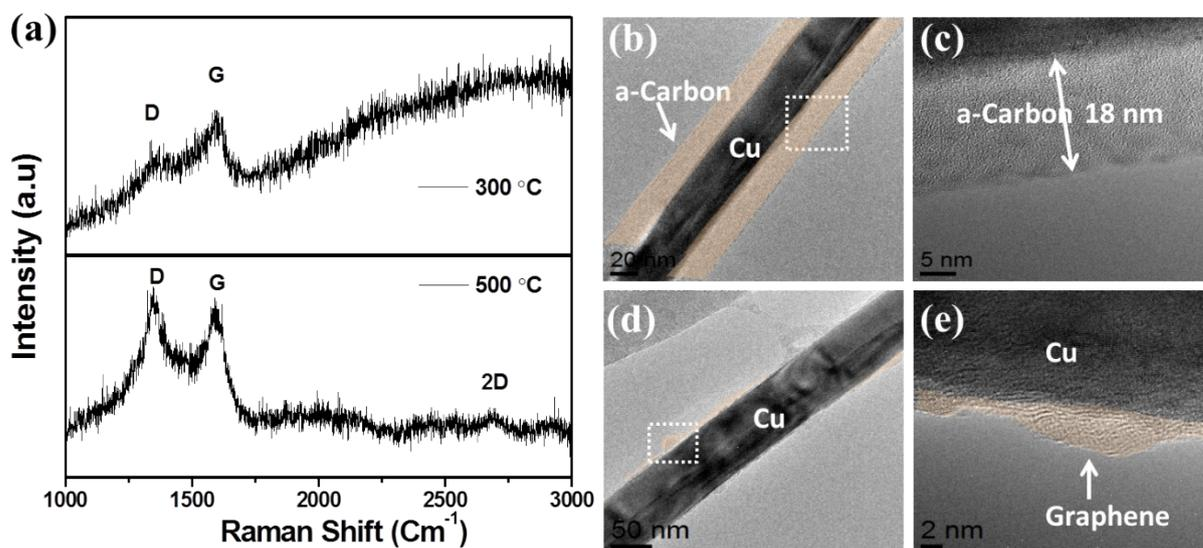
Fig. S2 (a) RAMAN spectra of a-carbon-coated Cu NWs grown at 300 °C (top) and graphene-coated Cu NWs grown at 500 °C (bottom), (b and c) HRTEM images of a-carbon coated Cu NW and (d and e) HRTEM image of graphene-coated Cu NW grown at 300 and 500 °C.
