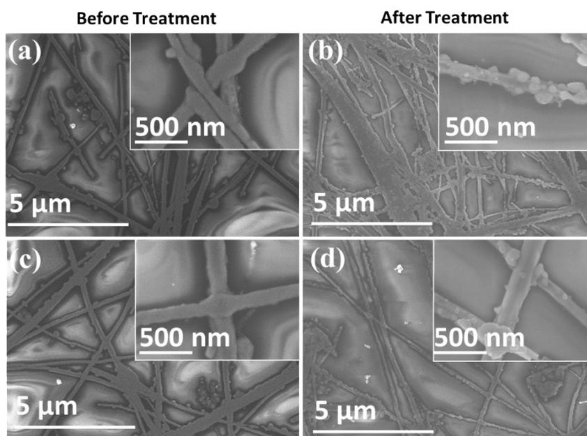
**Fig. S6** SEM images of Cu NWs TCE (a and b) before and after basic tests in the presence of 0.5 M NaCl (c and d) before and after acidic tests in the presence of 0.5 M H<sub>2</sub>SO<sub>4</sub>, respectively.
