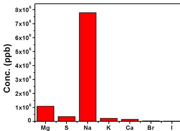
**Fig. S8** ICPMS results of the sea water collected from Penghu Island, Taiwan (concentration of element in ppb)
