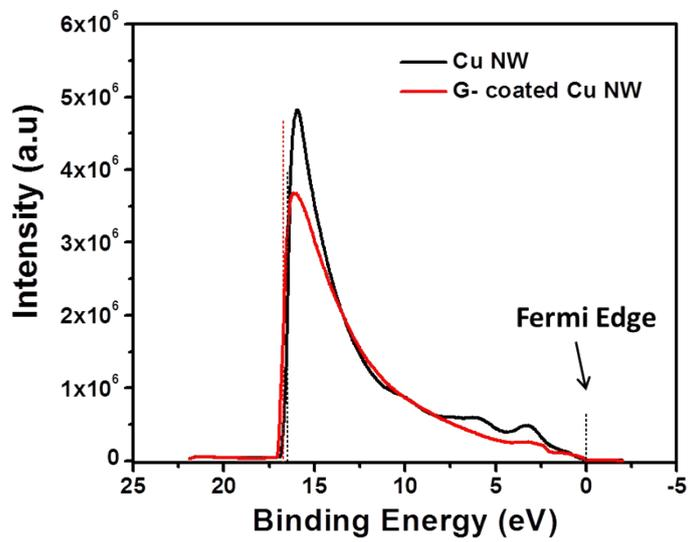
**Fig. S12** UPS plots of pure Cu NWs and graphene-coated Cu NWs.
