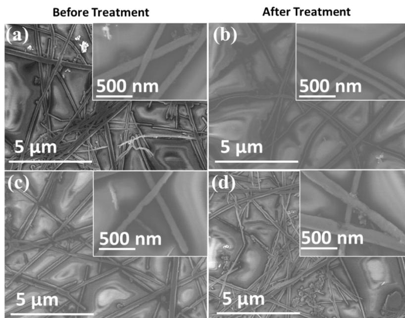
**Fig. S7** SEM images of graphene-coated Cu NW TCE (a and b) before and after basic tests in the presence of 0.5 M NaCl (c and d) before and after acidic tests in the presence of 0.5 M H<sub>2</sub>SO<sub>4</sub>.
