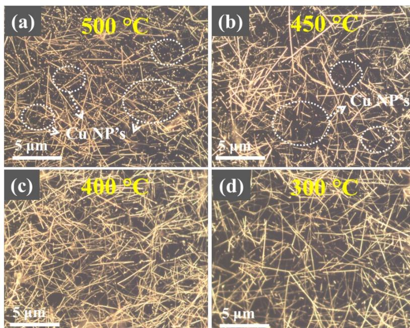
Fig.S1 (a-d) OM images of graphene-coated Cu NWs at different growth temperatures.
