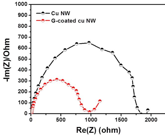
**Fig. S11** Electrode kinetics of Cu NWs and graphene- coated Cu NWs by Nyquist plots.
