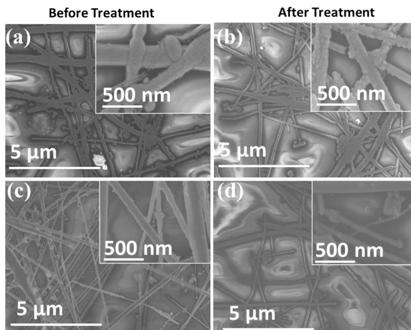
**Fig. S9** SEM images of Cu NW TCE (a & b) and graphene-coated Cu NW TCE (c & d) before and after sea water test.
