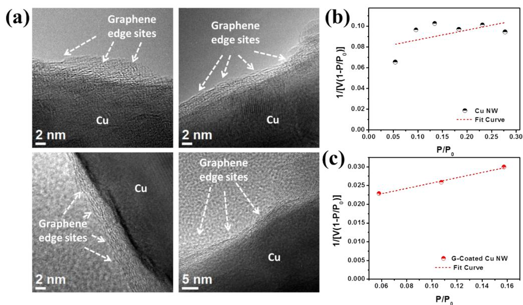
**Fig. S10** (a) HRTEM images of graphene-coated Cu NWs grown at 400 °C. (b) and (c) show brunauer–emmett–teller (BET) measurements of Cu NWs and graphene-coated Cu NWs, respectively.
