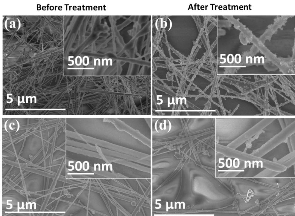
**Fig. S4** SEM images of Cu NWs TCE (a and b) and graphene-coated Cu NWs TCE (c and d) before and after oxidation tests at 240 °C in the presence  $O_2$  gas of 300 sccm.
