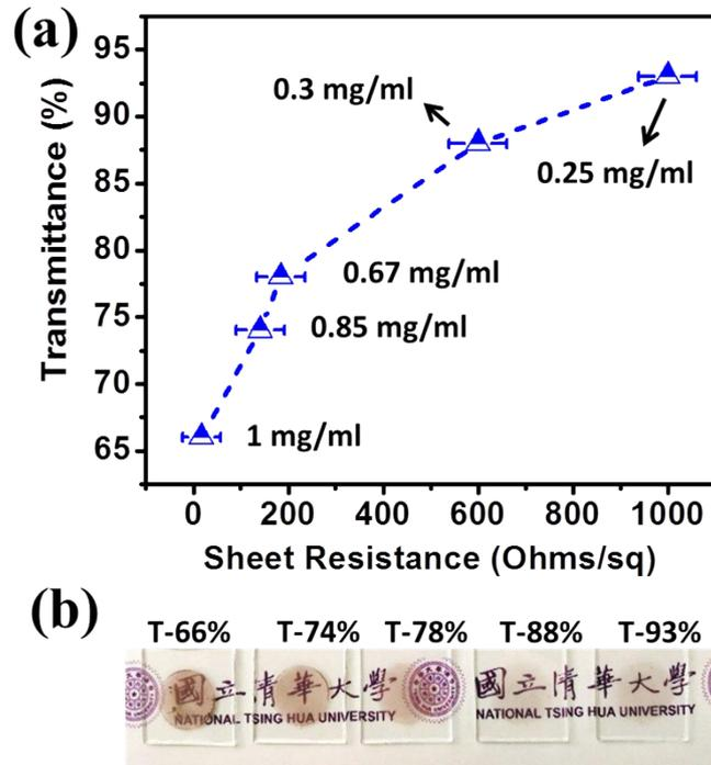
**Fig. S3** (a)  $R_s$  Vs  $T\%$  of a-carbon coated Cu NW TCE at 300 °C (b) photographic images of different concentration of samples.
