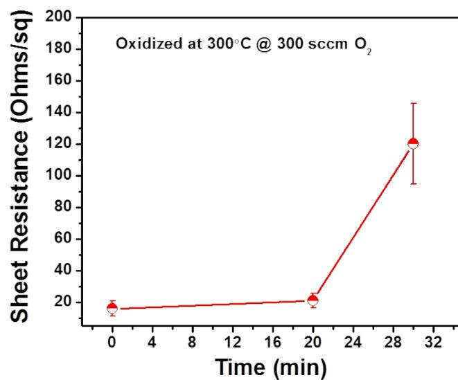
**Fig. S5** Rs vs Time plot of graphene-coated Cu NWs TCE after oxidized at 300 °C in the presence O<sub>2</sub> gas of 300 sccm.
