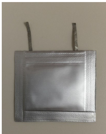
Fig. S7 Photograph of an asymmetric supercapacitor full cell.
