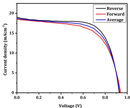
**Figure S7(c)** Photovoltaic performance of perovskite solar cells based on mp-TiO<sub>2</sub> measured by forward and reverse scans with 10mV voltage steps and 50ms delay times under AM 1.5 G illumination. Device configuration FTO/Bl-TiO<sub>2</sub>/ mp-TiO<sub>2</sub>+MAPbI<sub>3</sub>/PTAA/Au.
