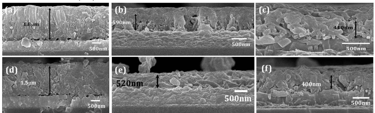
**Figure S7 (a)** Typical Cross Section micrograph of perovskite solar cell based on mp-TiO<sub>2</sub>. Device configuration FTO/Bl-TiO<sub>2</sub>/mp-TiO<sub>2</sub>+MAPbI<sub>3</sub>/PTAA/Au (Please note that Au contact is not shown in this cross section.)
