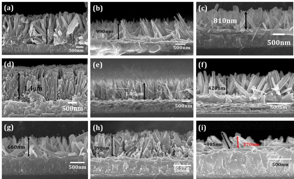
**Figure S3** Cross sectional FESEM images of TiO<sub>2</sub> nanorods deposited at 180°C and etched at 150°C. (a-c) 160 µl (d-f) 180 µl (g-i) 200 µl (j-l) 220µl TBT precursor and etched at 0, 3.0 and 3.5h respectively. (Note: Inset notation shows etching hours)
