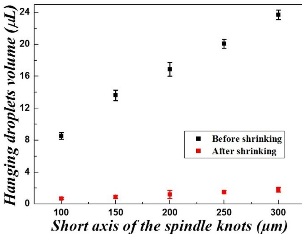
**Figure S7.** Volume of hanging droplets before and after shrinkage of the spindle knots. The long axis of the spindle knots was  $500\ \mu\text{m}$  and the distance between the spindle knots was  $1000\ \mu\text{m}$ .
