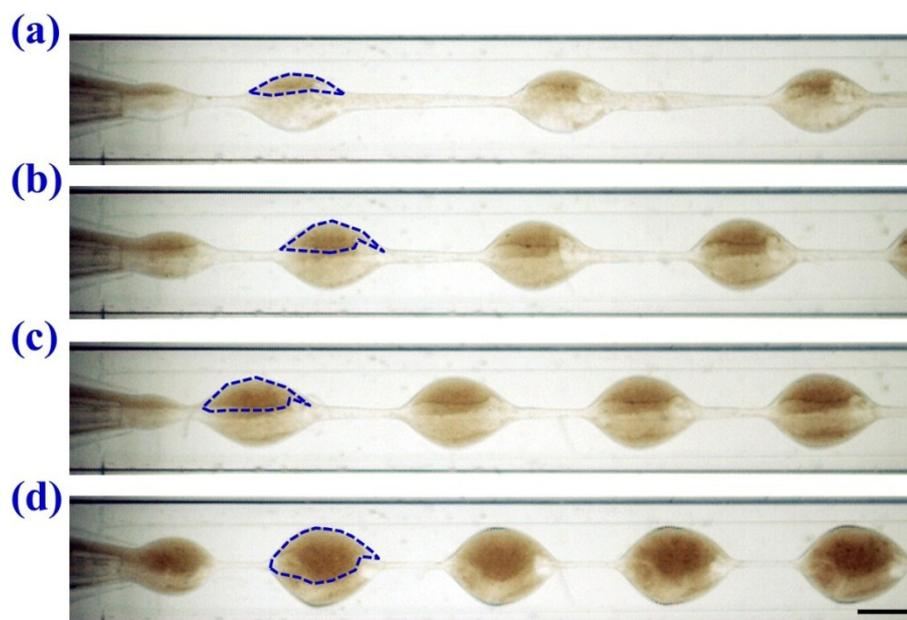
**Figure S2.** Microfluidic spinning and emulsification when  $F_1$  and  $F_2$  were too high. In these cases, the emulsification was disturbed, resulting in a nonuniform GO distribution, as marked by the blue dotted areas.
