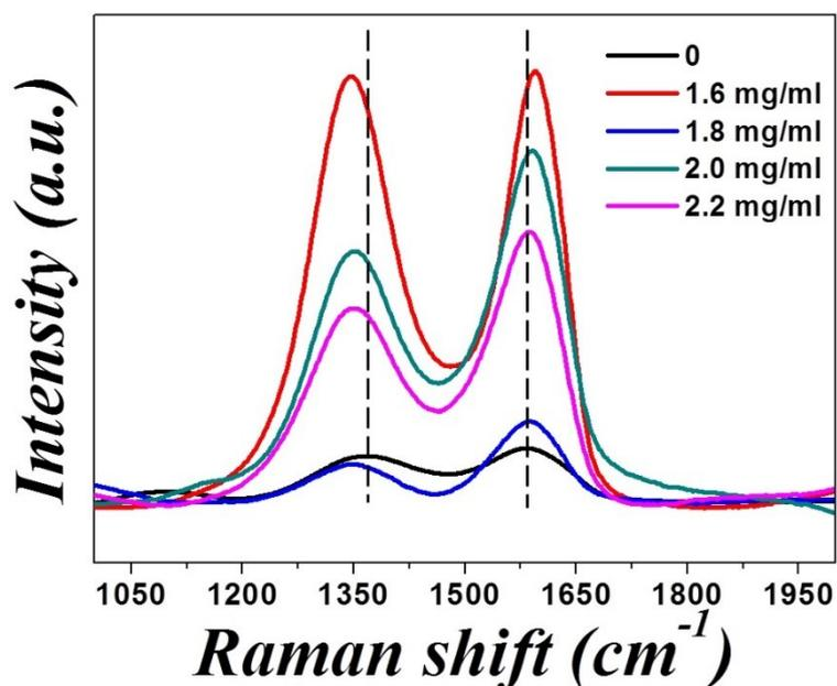
**Figure S4.** Raman spectra of the spindle knots prepared with different concentration of GO. The black dotted lines depict the peak positions. Compared with pure GO, the G peak of the GO/NIPAM composite spindle knots was blue-shifted from 1590  $\text{cm}^{-1}$  to 1602  $\text{cm}^{-1}$ , and D peak was red-shifted from 1365  $\text{cm}^{-1}$  to 1350  $\text{cm}^{-1}$ .
