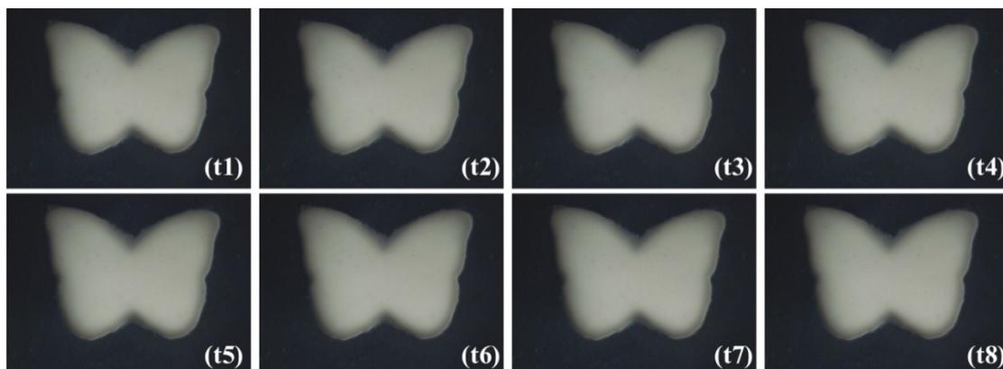
**Figure S1.** The pure NIPAM hydrogel under NIR irradiation: (t1-t5) with laser switched on; (t6-t8) with laser switched off.
