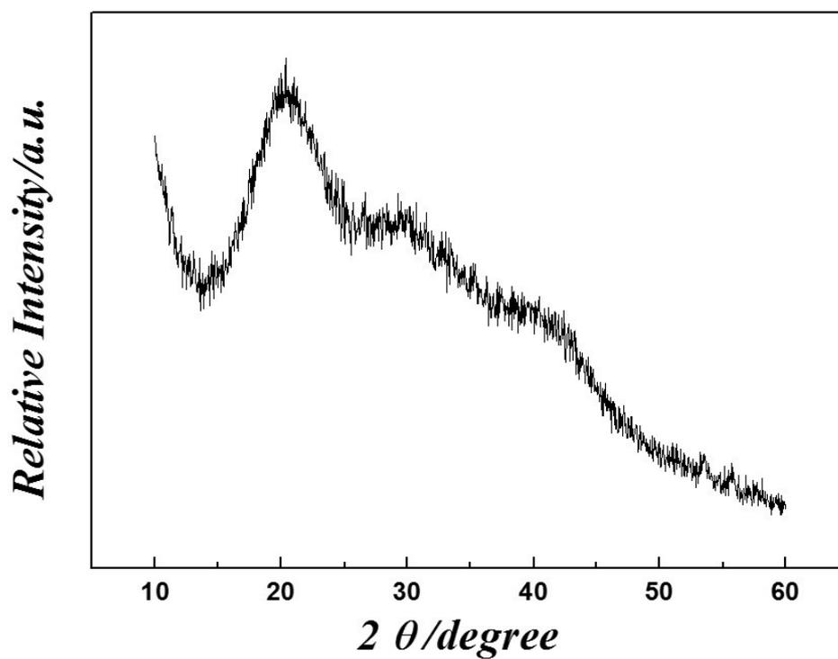
**Figure S5.** XRD pattern of spindle knots composed of GO/NIPAM composites. It showed diffraction peak of PNIPAM with diffraction peak at  $2\theta=20.36^\circ$  while no typical diffraction peak of GO, which indicated that the GO sheets were dispersed well into the polymer matrix.
