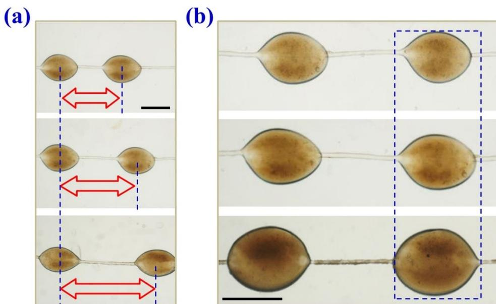
**Figure S3.** The resultant fibers with (a) different distances between the spindle knots and (b) different sizes of the spindle knots. The scale bar represents 400  $\mu\text{m}$ .
