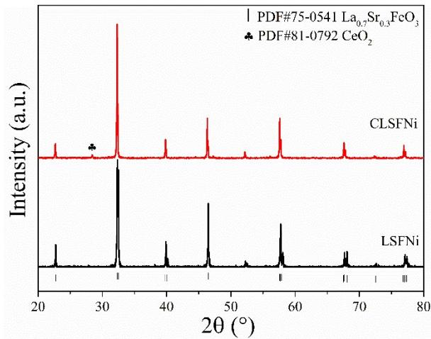
**Fig. S2** Post-mortem XRD patterns of samples after electrical conductivity measurement.
