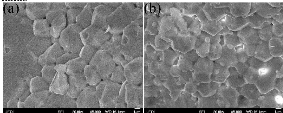
**Fig. S3** Post-mortem cross-section microstructure of samples after electrical conductivity measurement. (a) LSFNi; (b) CLSFNi.
