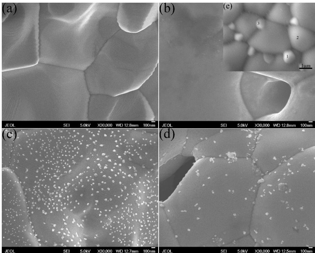
**Fig. S1** SEM images of (a, b) as-synthesized LSFNi and CLSFNi; (c, d) reduced LSFNi and CLSFNi under 10%  $\text{H}_2$  atmosphere at 800  $^{\circ}\text{C}$  for 10 h; (e) SEM image of CLSFNi at low magnification.
