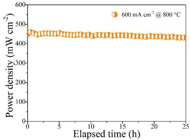
**Fig. S6** Stability of the LSFNi symmetrical cell with  $\text{H}_2$  (3%  $\text{H}_2\text{O}$ ) under a constant current density of  $600 \text{ mA cm}^{-2}$  at  $800^\circ\text{C}$ .
