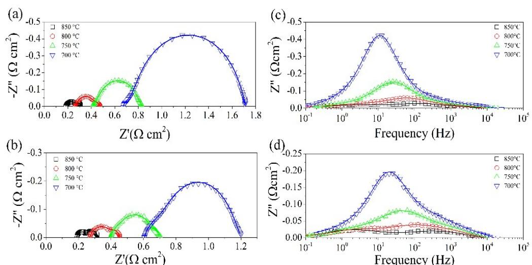
Fig. S5 Fitting results of EIS for H<sub>2</sub>-fueled symmetrical cells.(a, c) LSFNi electrode; (b, d) CLSFNi electrode.
