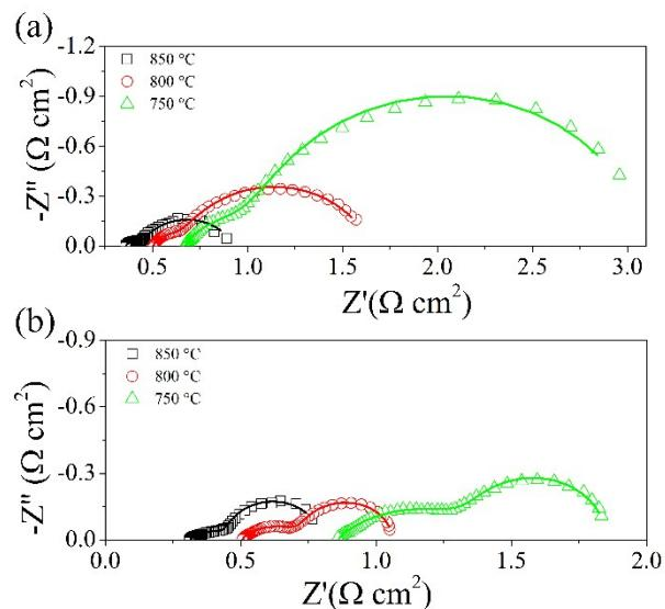
Fig. S7 Fitting results of EIS for  $\text{CH}_4$ -fueled symmetrical cells.(a) LSFNi electrode; (b) CLSFNi electrode.
