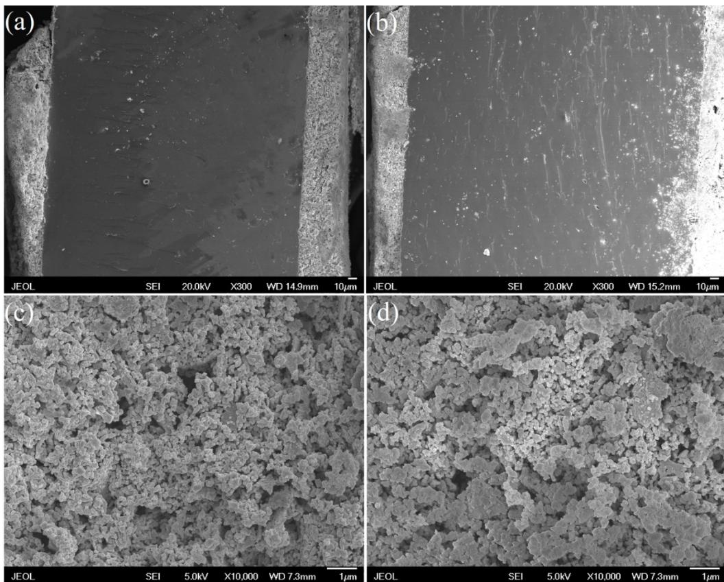
**Fig. S8** Microstructure and cross section of symmetrical cells. (a) LSFNi/LSGM/LSFNi after stability testing with H<sub>2</sub> as fuel; (b) CLSFNi/LSGM/CLSFNi after stability testing with CH<sub>4</sub> as fuel; (c) cathode section of (b); (d) anode section of (b).
