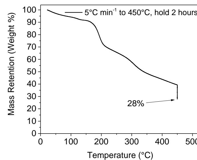
Figure S1. Thermogravimetric analysis of powdered milk.
