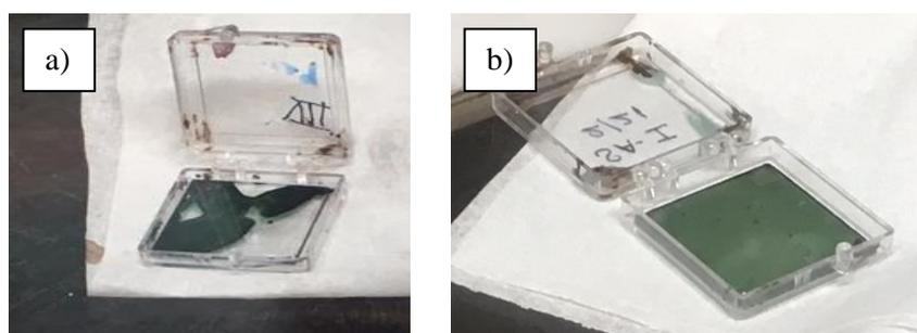
**Figure S4:** a) Example of incomplete coverage of the substrate and gelation in case of higher molecular weight PffBT4T-2OD with the initial processing set-up (commercial sample of Solarmer,  $M_n = 57.2$  kDa); b) Example of a properly spin-coated active layer, with lower molecular weight PffBT4T-2OD (Table 5, entry 5) and using the initial processing set-up.
