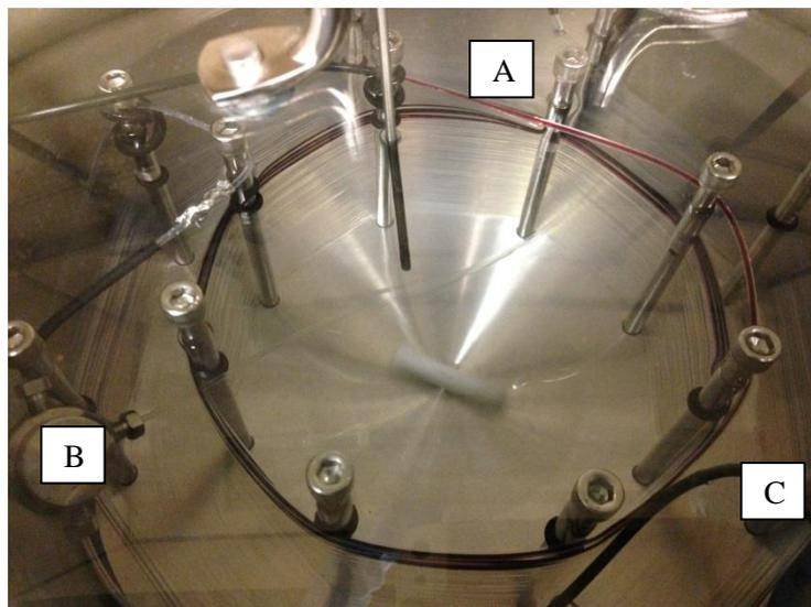
**Figure S2:** The tubular flow reactor is immersed in an oil bath. The incoming reaction mixture (A) rapidly turns deep purple. Before exiting the reactor (C), the reaction mixture is diluted (B) by a stream of fresh solvent, in which also the palladium scavenging agent is dissolved.
