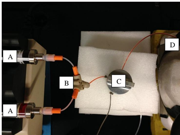
**Figure S1:** Reagents are injected into the continuous flow reactor (D) by two SGE gastight syringes (A), a T-piece mixer (B) and a 4-way valve (C).
