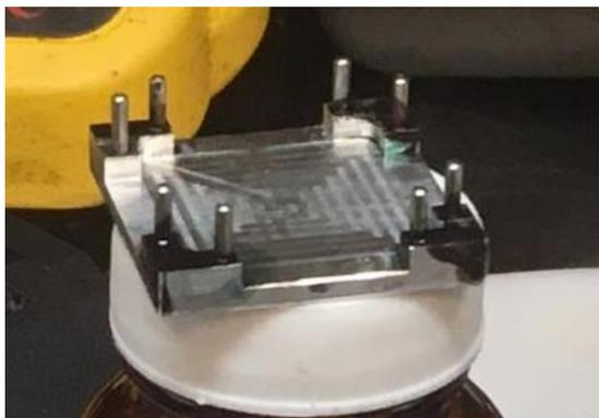
**Figure S3:** The modified processing chuck, which allows elevation of the glass substrate from the cold metal surface. The substrate rests on the four corners and is kept in place with 8 pins.
