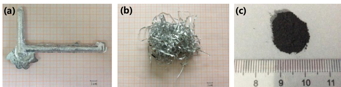
Figure S2. Photographs of (a) \text{Al}_{97.8}\text{Ni}_2\text{Pt}_{0.2} alloy ingot, (b) \text{Al}_{97.8}\text{Ni}_2\text{Pt}_{0.2} alloy ribbons, and (c) PtNi NPNWs catalyst after dealloying.
