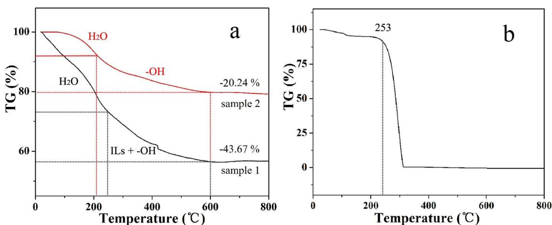
**Fig. S3.** TG curves of  $\alpha$ -Fe<sub>2</sub>O<sub>3</sub> precursors of sample 2 and sample 1 (a); TG curve of [C<sub>12</sub>mim][Br] (b).
