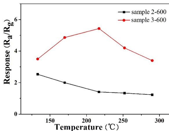
**Fig. S5.** The responses of the  $\alpha$ -Fe<sub>2</sub>O<sub>3</sub> nanorods sensors (sample 2-600 and sample 3-600) to 100 ppm TMA measured at different operating temperatures.
