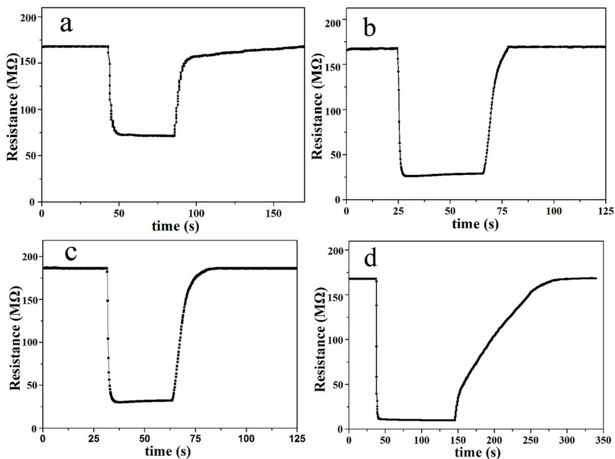
**Fig. S6.** Sensing transients of the  $\alpha$ -Fe<sub>2</sub>O<sub>3</sub> nanorod arrays sensor to volatiles (0 and 25 °C) come from fresh (a, c) and 11 h stored (b, d) fish measured at the working temperature of 217 °C.
