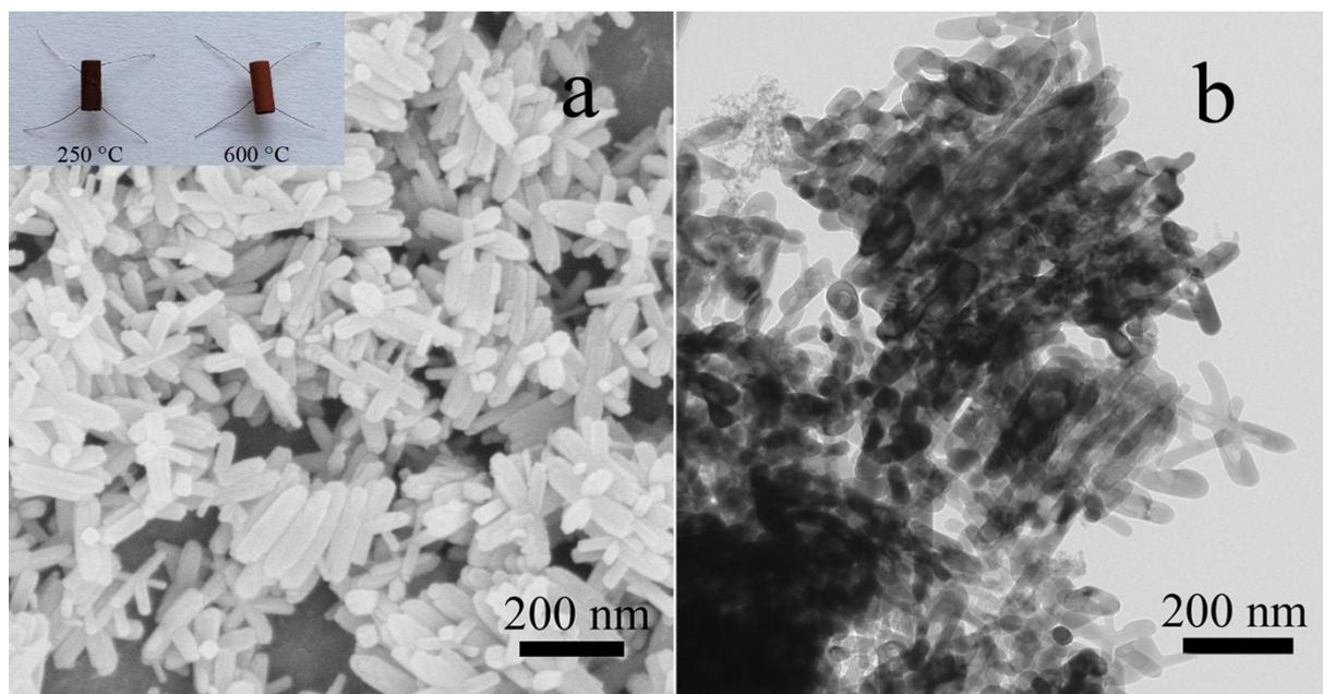
**Fig. S2.** Typical SEM, Picture (inset) (a) and TEM (b) images of sample 2 after calcined at 600 °C.
