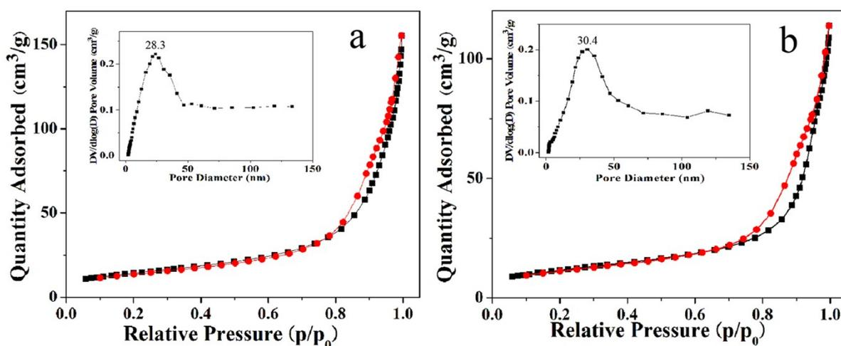
**Fig. S4.** Nitrogen adsorption-desorption isotherms and pore size distribution curve (inset) of sample 2 calcined at 250 °C (a) and 600 °C (b).
