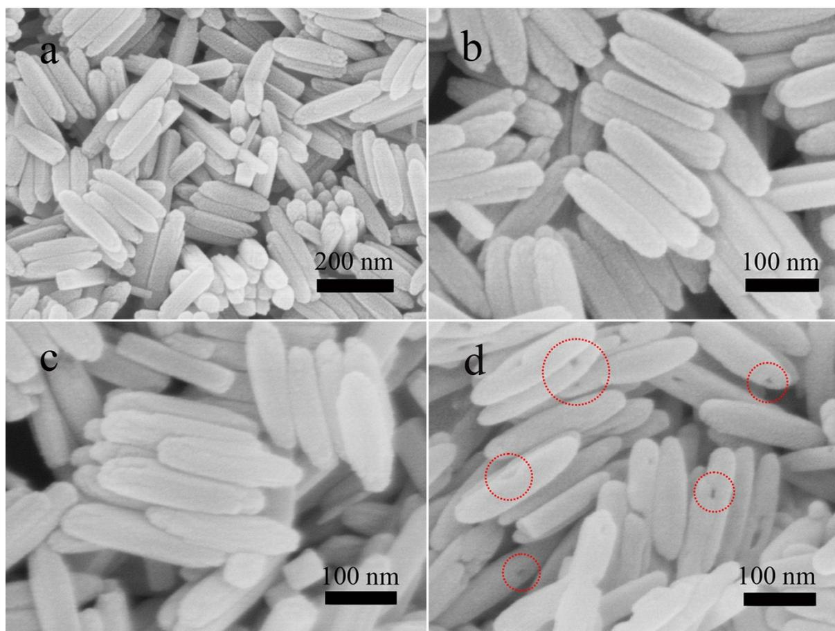
**Fig. S1.** Typical SEM images of precursor sample 1 (a), sample 1-250 (b), sample 1- 400 (c) and sample 1- 600 (d) precipitated at the bottom of the autoclave.
