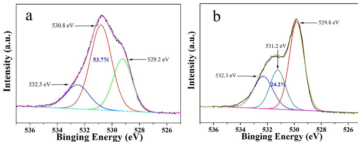
**Fig. S8.** O 1s XPS spectra of the  $\alpha$ -Fe<sub>2</sub>O<sub>3</sub> nanorod arrays (sample 1-250) sensor before (a) and after (b) exposure to 100 ppm to TMA at 217 °C.
