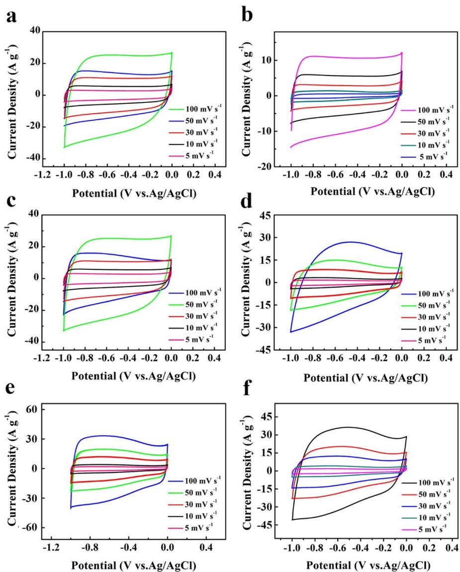
**Figure S4.** CV curves at different scan rates of 5, 10, 30, 50 and 100  $\text{mV s}^{-1}$  of the (a) PCTBs, (b) CTBs, (c) PCTBs2-1, (d) N-PCTBs, (e) B-PCTBs and (f) B/N-PCTBs.
