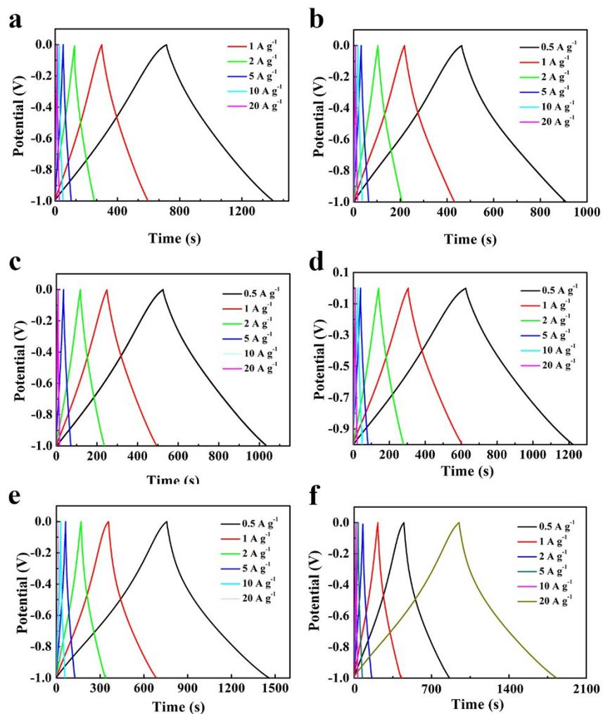
**Figure S5.** Galvanostatic charge/discharge curves versus various current densities (0.5-20 A g<sup>-1</sup>) of the (a) PCTBs, (b) CTBs, (c) PCTBs2-1, (d) N-PCTBs, (e) B-PCTBs and (f) B/N-PCTBs.
