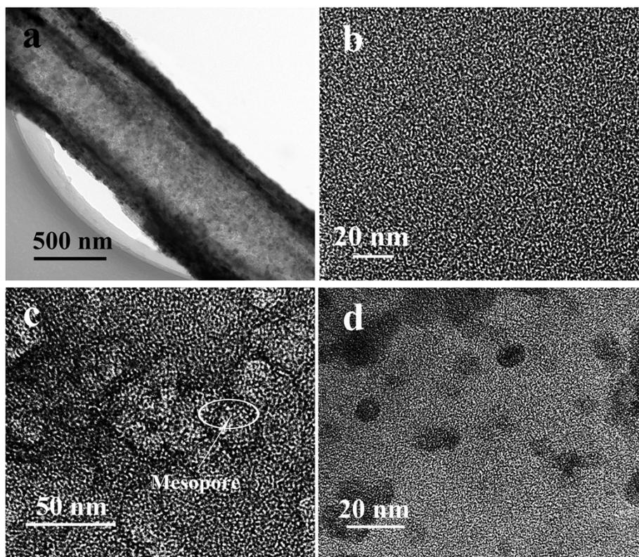
**Figure S2.** (a) TEM and (b) HRTEM images of the CTBs. (c, d) HRTEM images of the PCTBs, illustrating the abundant mesopores and micropores distribute uniformly inside the PCTBs.
