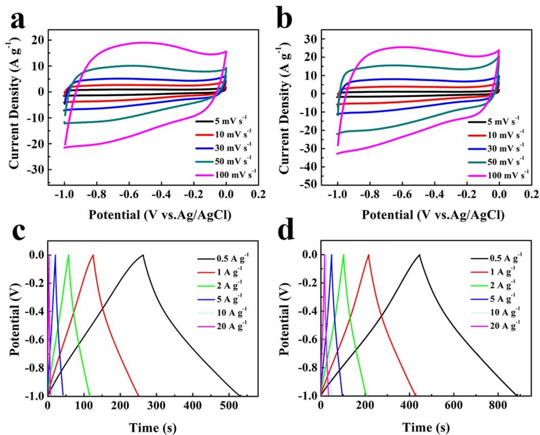
**Figure S9.** Electrochemical performance of the AC and B/N-PCTBs with a high mass loading of 40 mg cm<sup>-2</sup>. CV curves at various scan rates of 5, 10, 30, 50 and 100 mV s<sup>-1</sup> of the (a) AC and (b) B/N-PCTBs. Galvanostatic charge/discharge curves versus different current densities (0.5-20 A g<sup>-1</sup>) of the (c) AC and (d) B/N-PCTBs.
