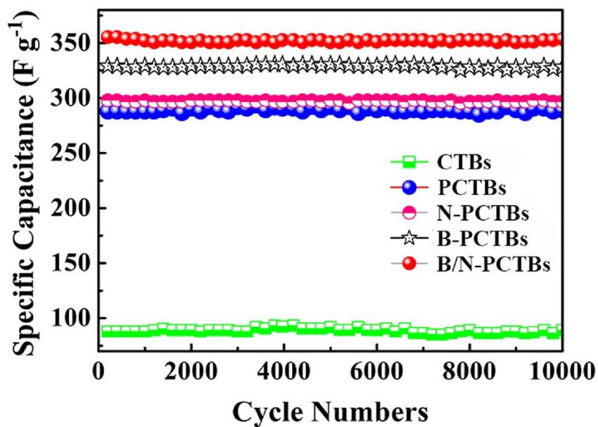
**Figure S7.** Cycling performance of the CTBs, PCTBs, N-PCTBs, B-PCTBs and B/N-PCTBs electrodes at a 1 A g<sup>-1</sup> for 10,000 cycles.
