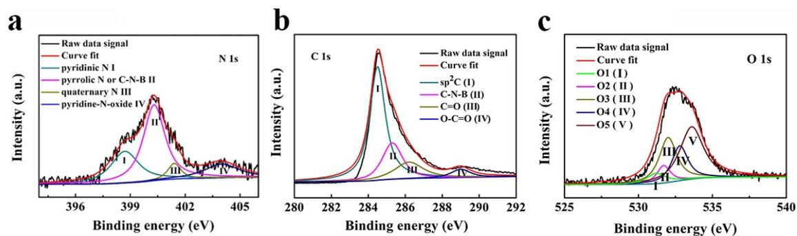
**Figure S3.** (a) High-resolution N1s and its fitting peaks of the N-PCTBs. (b) High-resolution C1s and its fitting peaks of the B/N-PCTBs. (c) High-resolution O1s and its fitting peaks of the B/N-PCTBs.
