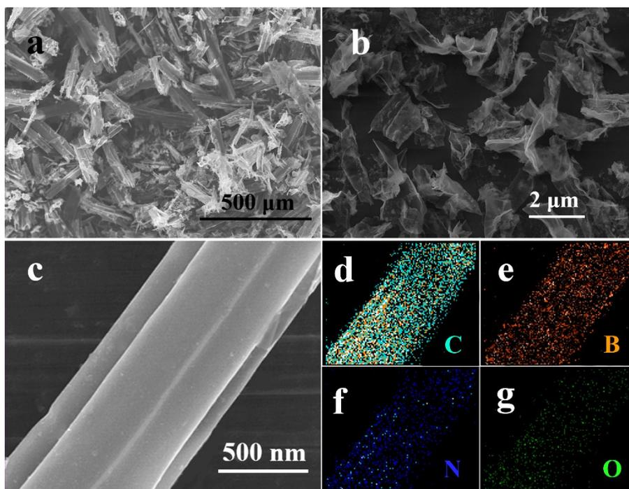
**Figure S1.** (a, b) SEM images of the PCTBs1-2. The SEM images demonstrate the morphology of the carbon tube bundle is destroyed by the KOH. (c-g) SEM image and corresponding C, B, N and O elemental mappings of the B/N-PCTBs, demonstrating the uniform distributions of B, N and O atoms.
