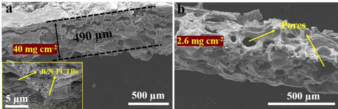
**Figure S11.** (a) SEM image showing the cross-section of the B/N-PCTBs electrode with a mass loading of  $40 \text{ mg cm}^{-2}$ . The enlarged SEM showing the B/N-PCTBs interconnect with each other (inset). (b) SEM image showing the cross-section of the B/N-PCTBs electrode with a mass loading of  $2.6 \text{ mg cm}^{-2}$ . There are many pores without filled with active materials.
