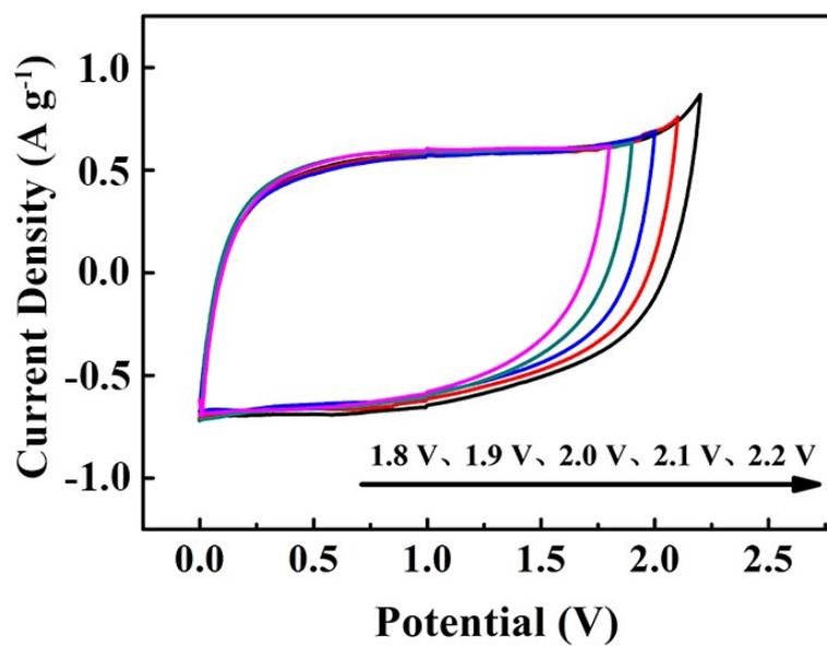
**Figure S10.** CV curves of the symmetric cell with a total active material mass loading of 80 mg cm<sup>-2</sup> within different voltage ranges at 20 mV s<sup>-1</sup>. The potential of 1.8 V was adopted as the operating voltage in this work.
