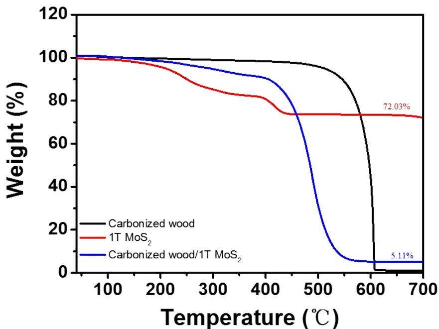
**Figure S4:** TGA curves of carbonized wood, 1T MoS<sub>2</sub> and CW/1T MoS<sub>2</sub> at a heating speed of 10°C/min in air. The weight percentage of 1T MoS<sub>2</sub> in the CW/1T MoS<sub>2</sub> was presumed to be  $x$ . Assuming the carbonized wood was completely removed after combustion,  $0.7203x=0.0511$ , therefore  $x=7.1\%$ .
