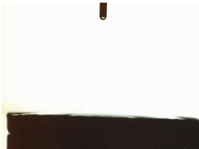
**Supplementary Video 3:** Snapshot from the video of contact angle measurement showing the wettability of CW/1T MoS<sub>2</sub>.
