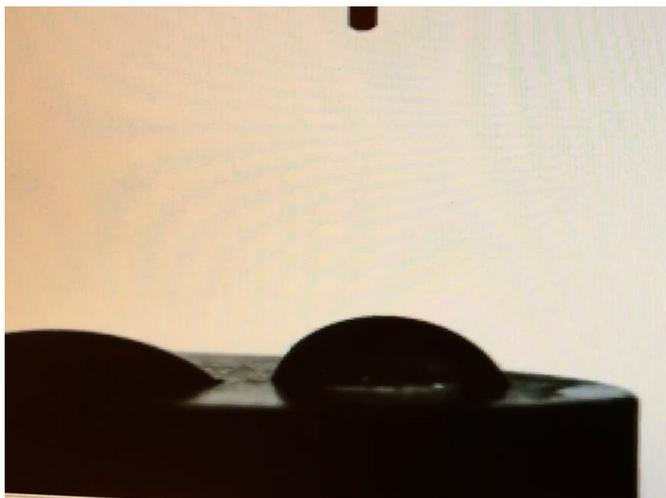
**Supplementary Video 4:** Snapshot from the video of contact angle measurement showing the wettability of the rotating disk electrode coated with 1T MoS<sub>2</sub>.
