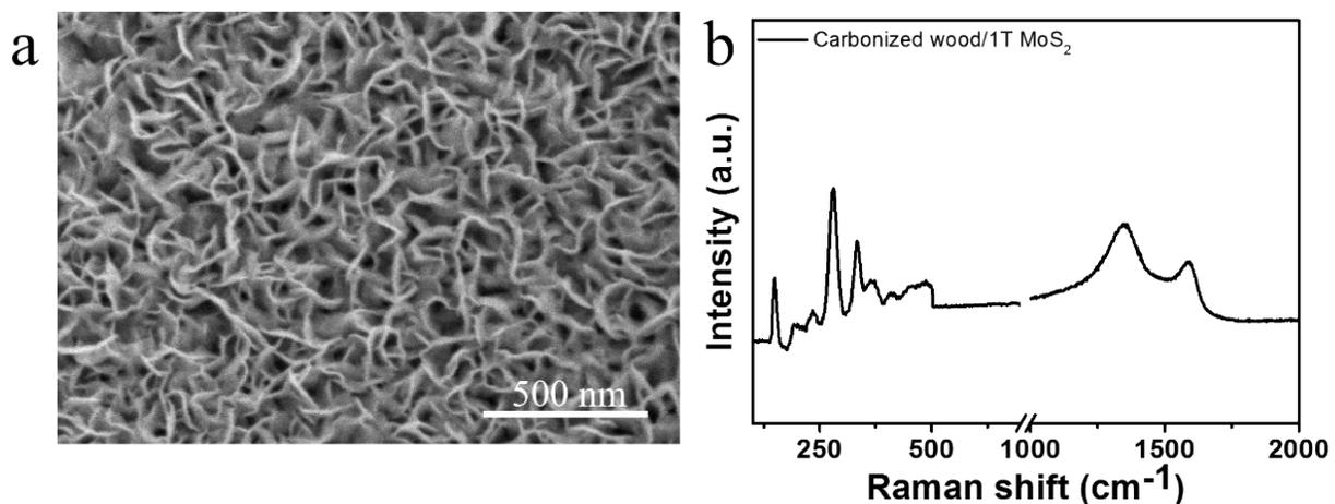
**Figure S6:** SEM images of (a) CW/1T MoS<sub>2</sub> after HER test. (b) Raman spectra of CW/1T MoS<sub>2</sub> after HER test.
