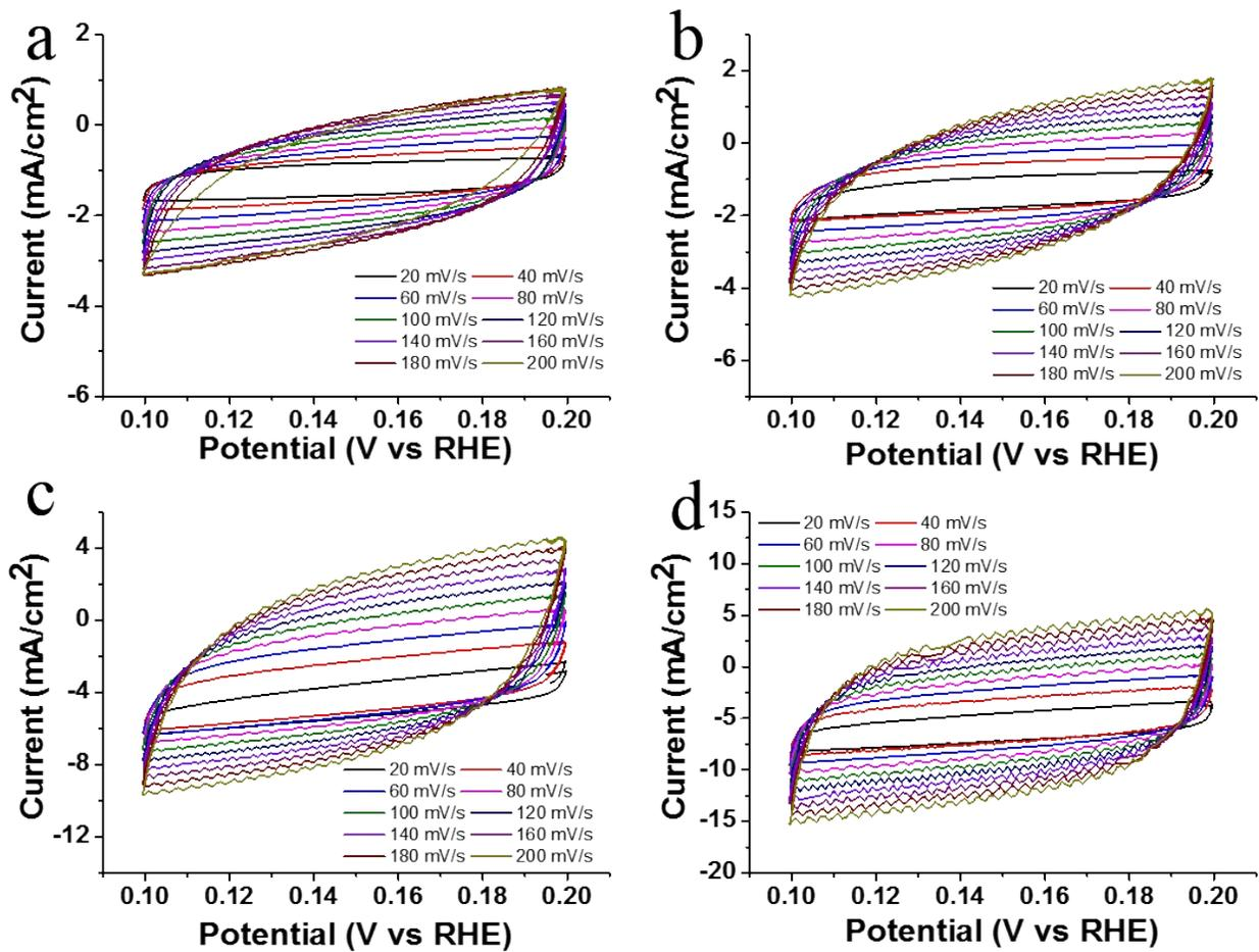
**Figure S8:** Cyclic voltammogram (CV) curves in the region of 0.1-0.2 V vs. RHE for (a) 2H MoS<sub>2</sub> (b) 1T MoS<sub>2</sub> (c) CW/2H MoS<sub>2</sub> (d) CW/1T MoS<sub>2</sub>.
