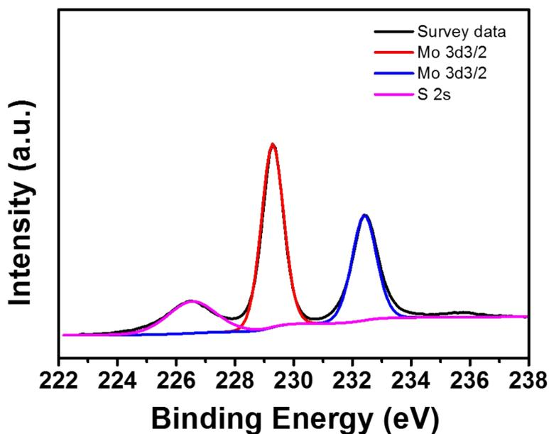
**Figure S5:** High-resolution XPS spectra of the Mo element in pure 1T MoS<sub>2</sub>.
