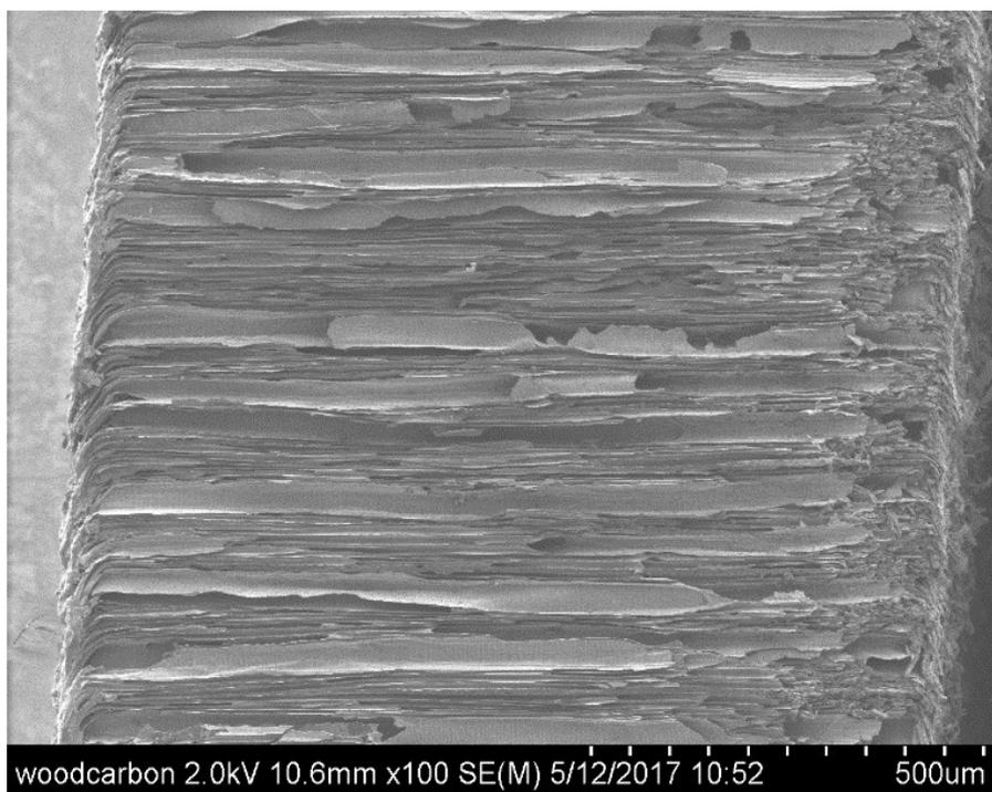
**Figure S1:** SEM image of CW/IT MoS<sub>2</sub> for measurement of the thickness ~1000 μm.
