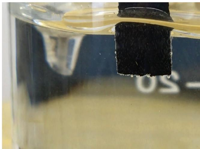
**Supplementary Video 1:** Snapshot from the video of the HER test using the freestanding CW/1T MoS<sub>2</sub> as the working electrode, where the H<sub>2</sub> bubbles were easily released from the surface of the working electrode benefiting H<sub>2</sub> production.
