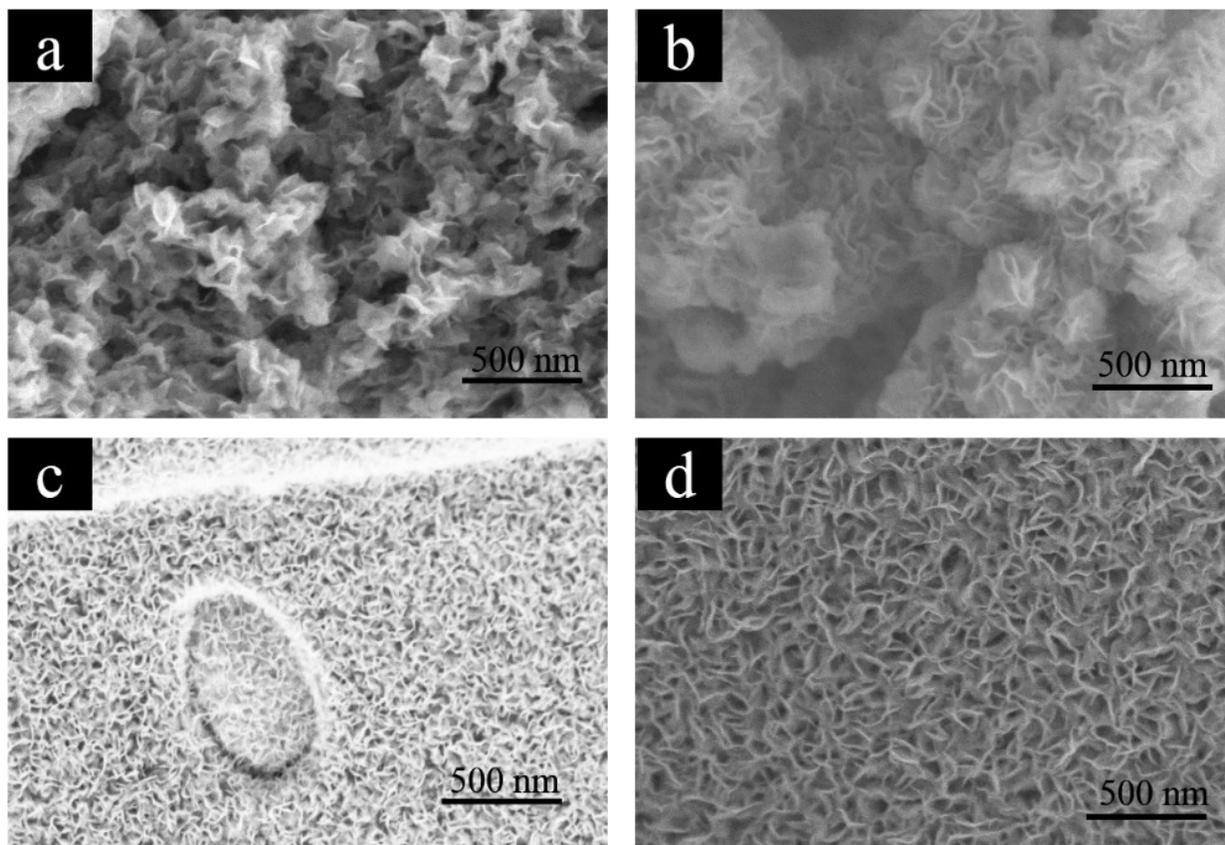
**Figure S7:** SEM images of (a) 2H MoS<sub>2</sub> after coating on glassy carbon, displaying the apparent aggregation of MoS<sub>2</sub> nanosheets. (b) 1T MoS<sub>2</sub> after coating on glassy carbon displaying nano-flower like morphology. SEM image of the unique arrangement of the 1T MoS<sub>2</sub> nanosheets perpendicular array on the (c) carbonized wood channel with a pit hole on the channel wall. (d) carbonized wood surface.
