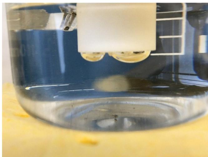
**Supplementary Video 2:** Snapshot from the video of the HER test using 1T MoS<sub>2</sub> coated on the glassy carbon as the working electrode showing huge H<sub>2</sub> bubbles strongly adsorbed on the surface of the glassy carbon hindering the interaction between active sites and electrolyte.
