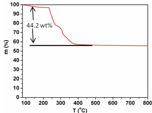
SI 1 TGA curves of GC-Co nanocages in air.
