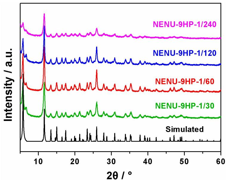
**Fig. S4** PXRD patterns of simulated NENU-9 and NENU-9HP-1/V.
