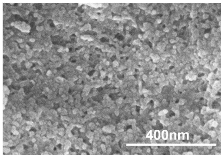
**Fig. S11** SEM image of hierarchically porous MIL-53(Al).
