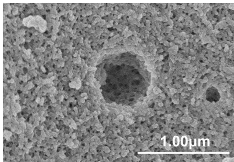
**Fig. S19** SEM image of NENU-9HP-1/120 after recycling for 5 times.
