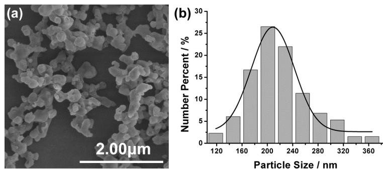
**Fig. S1** (a) SEM image and (b) particle analysis of sample synthesized in mix solvent of ethanol and water.
