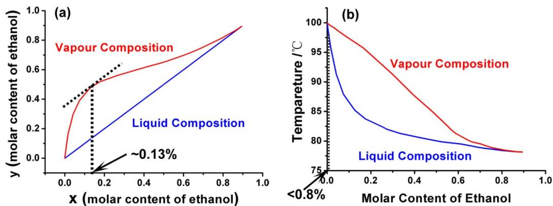
**Fig. S3** (a) x-y phase diagram and (b) T-x-y phase diagram of ethanol and water.
