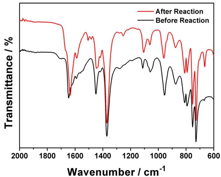
**Fig. S18** FTIR spectra of NENU-9HP-1/120 before and after recycling for 5 times.
