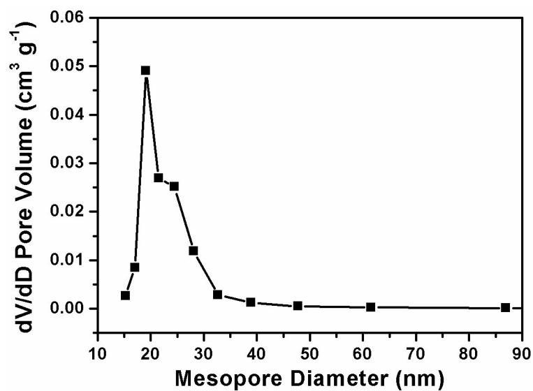
**Fig. S13** Mesopore size distribution of hierarchically porous MIL-53(Al).
