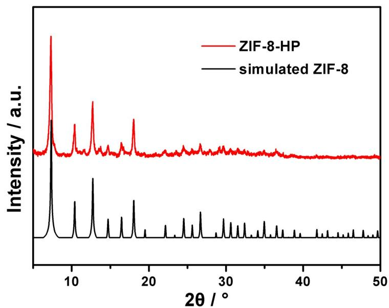
**Fig. S6** PXRD patterns of hierarchically porous and simulated ZIF-8.
