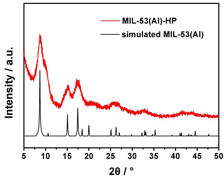
**Fig. S10** PXRD patterns of hierarchically porous and simulated MIL-53(Al).
