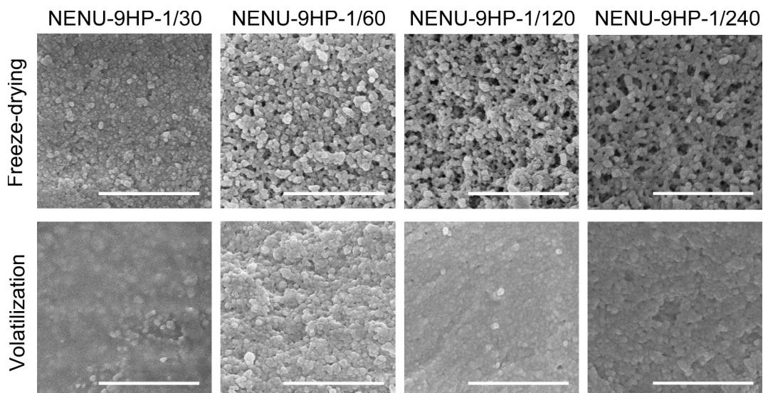
**Fig. S2** The comparison of samples prepared by freeze-drying and volatilization. The scale bars are all 1 μm.
