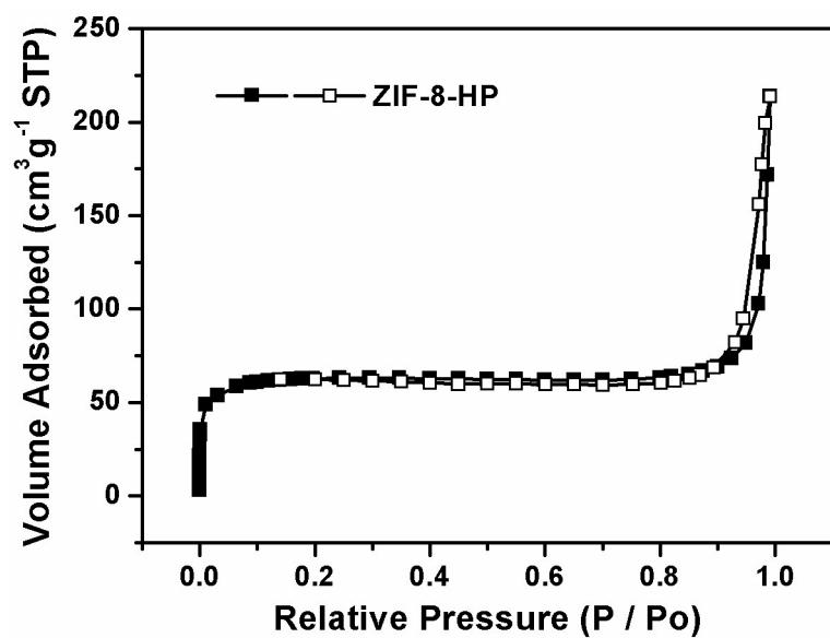
**Fig. S8**  $\text{N}_2$  sorption isotherm of hierarchically porous ZIF-8.
