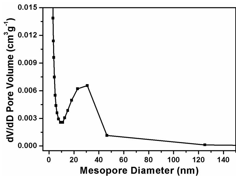
**Fig. S23** Mesopore size distribution of NENU-9HP-1/120 sonicated in ethanol.
