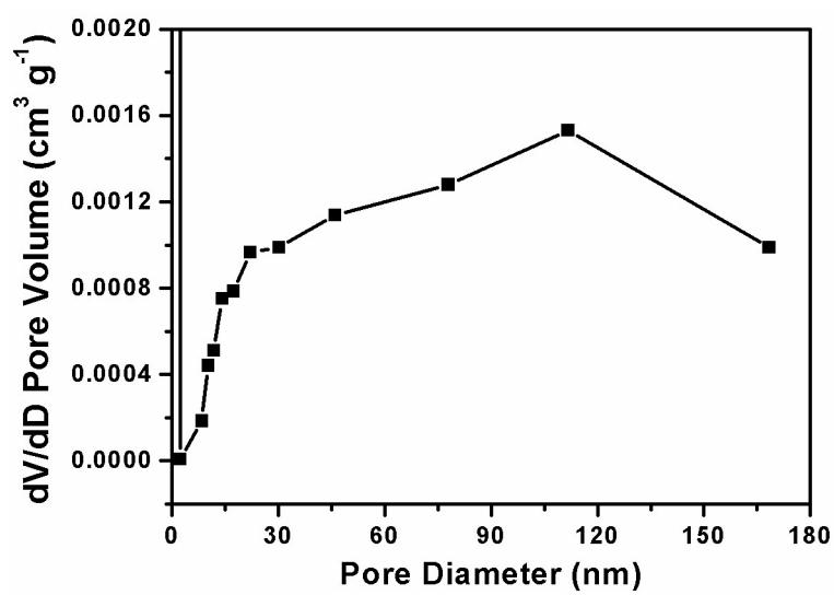
**Fig. S9** Mesopore size distribution of hierarchically porous ZIF-8.
