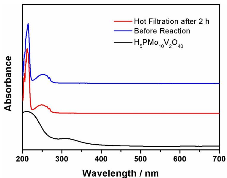
**Fig. S17** UV-Vis spectra of  $\text{H}_5\text{PV}_2\text{Mo}_{10}\text{O}_{40}$ , solution before reaction and filtrate after 2 h of reaction.
