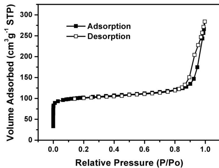
**Fig. S20** N<sub>2</sub> sorption isotherm of NENU-9HP-1/120 after recycling for 5 times.
