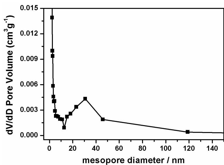
**Fig. S21** Mesopore size distribution of NENU-9HP-1/120 after recycling for 5 times.
