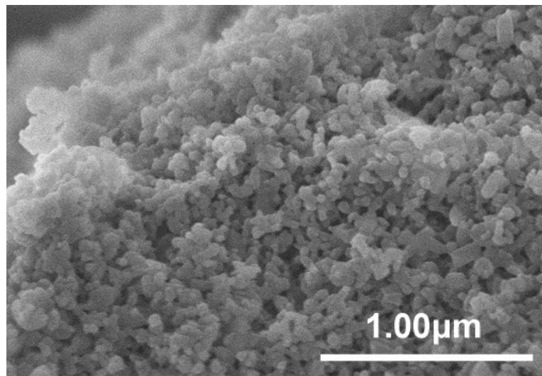
**Fig. S7** SEM image of hierarchically porous ZIF-8.
