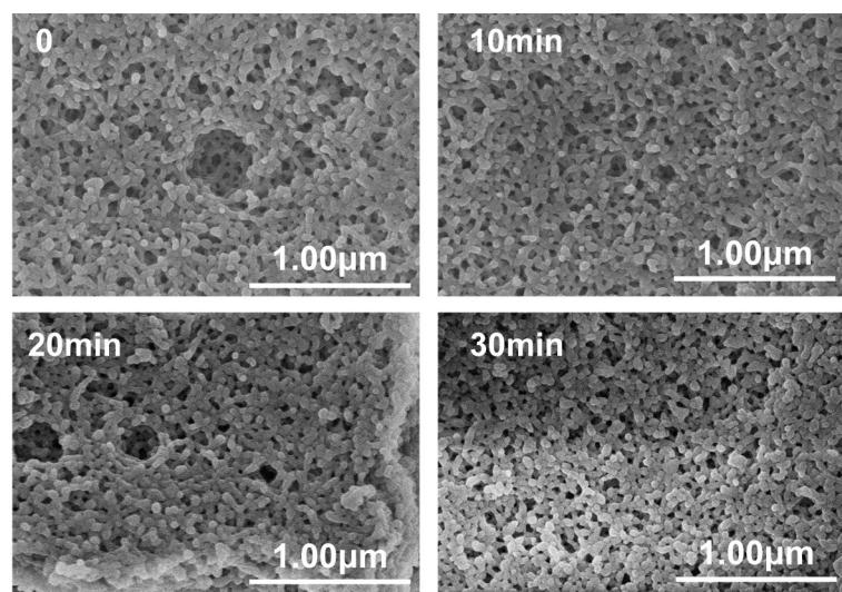
**Fig. S22** SEM images of NENU-9HP-1/120 sonicated in ethanol.
