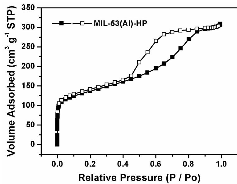
**Fig. S12** N<sub>2</sub> sorption isotherm of hierarchically porous MIL-53(Al).
