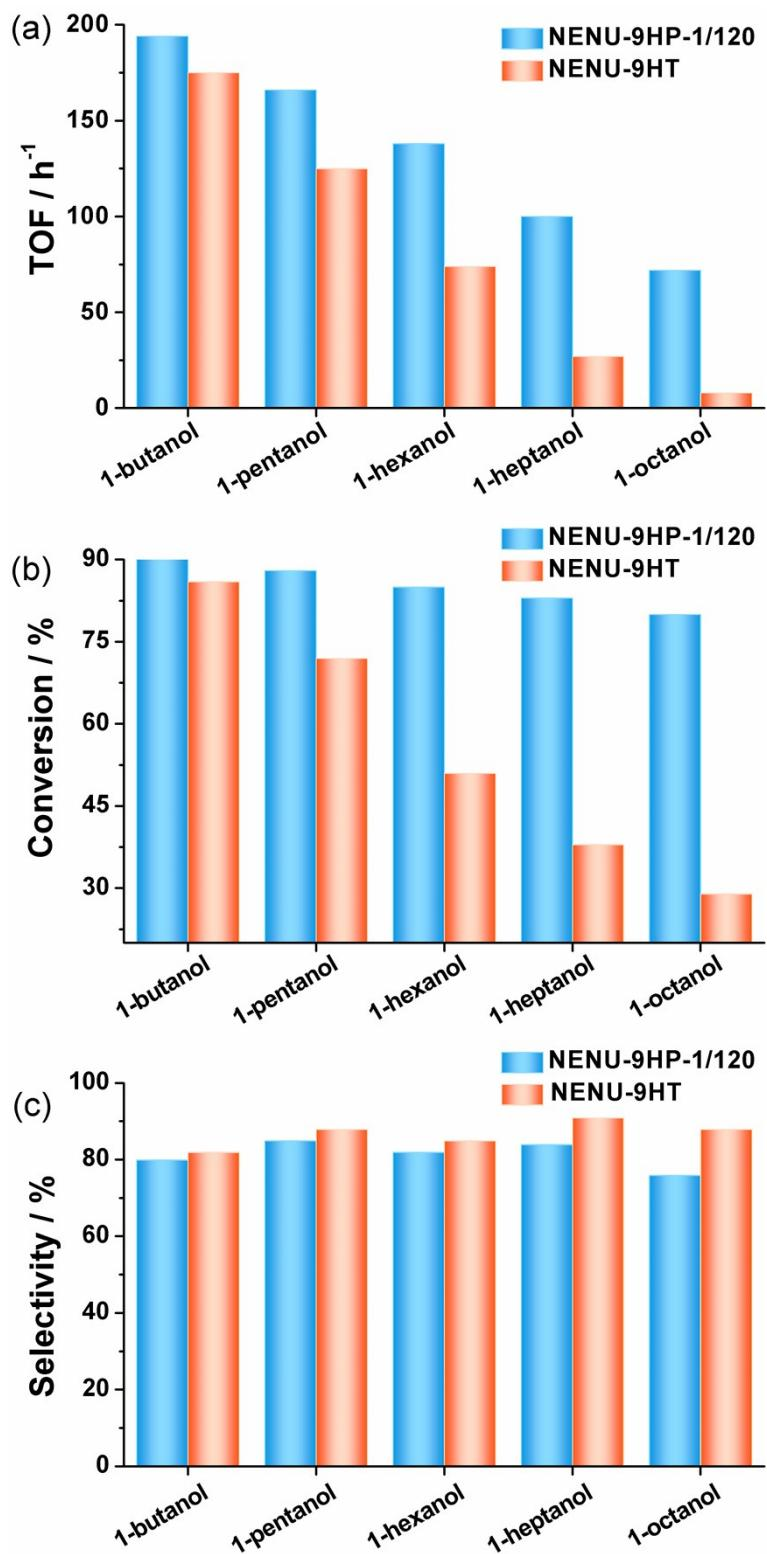
**Fig. S16** (a) TOF values evaluated on the basis of the moles of the whole catalyst and reactive moles of substrates in 20 min, (b) conversions after 24 h of different primary fatty alcohols and (c) selectivity towards corresponding aldehydes catalyzed by NENU-9HP-1/120 and NENU-9HT.
