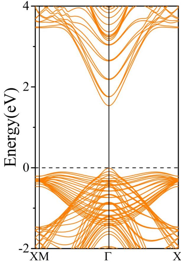
**Fig. S5.** Band structure of Cd-Se bonds at the edge for zigzag configuration. The value of bandgap at PBE level is 1.54 eV which is equal to the interface jointed by Zn-S bonds configuration. It's have a direct bandgap for both VBM and CBM are all located at  $\Gamma$  point. For these two structures, the binding energy are -4.879 eV and -4.883 eV, respectively.
