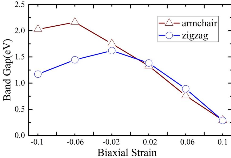
**Fig. S2.** The varization of band gaps of a-CdS/ZnSe and z-CdS/ZnSe as a function of biaxial strain. Blue and wine lines represent linear fitting of zigzag and armchair configurations, respectively.
