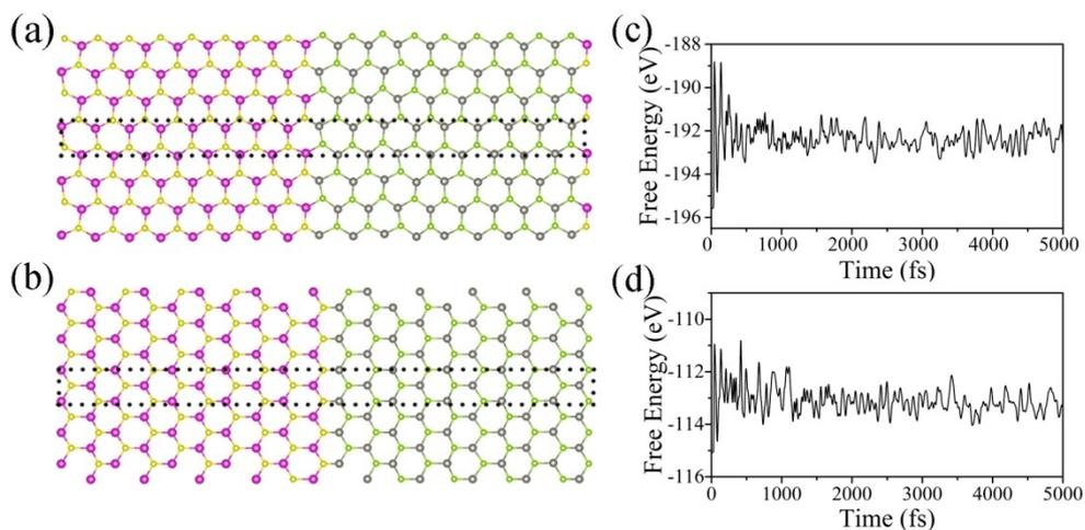
**Fig. S1.** Top views of the snapshots taken from the end of the AIMD simulations at the temperature of 500 K for (a) a-CdS/ZnSe and (b) z-CdS/ZnSe. The variation of the free energies for (a) a-CdS/ZnSe and (b) z-CdS/ZnSe in the AIMD simulations at 500 K during the timescale of 5 ps.
