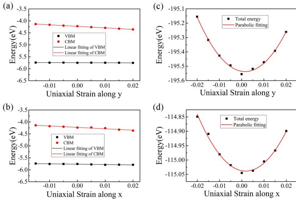
**Fig. S3.** Band edge positions and total energy as a function of the uniaxial strain for (a, c) a-
