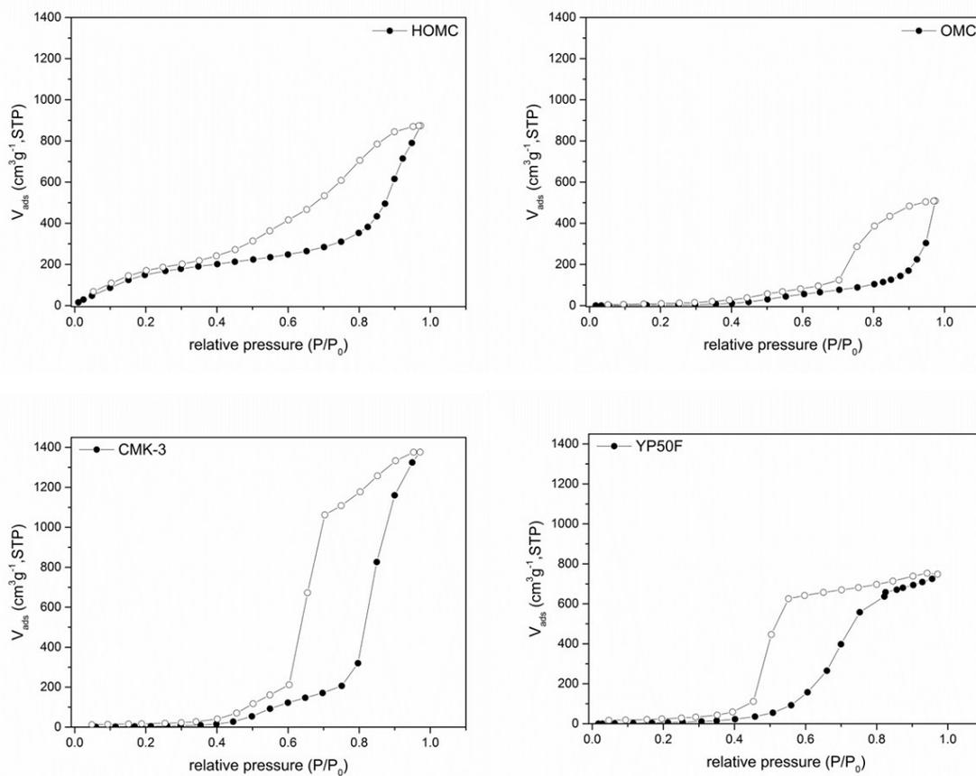
**Figure S13.** Water adsorption isotherm for the HOMC and the reference materials OMC, CMK-3 and YP50F.
