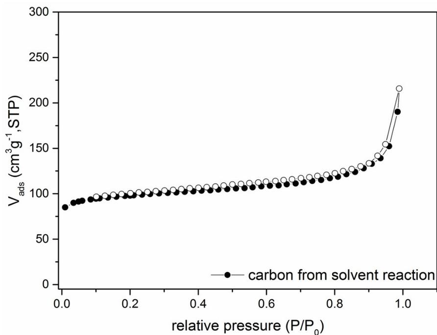
**Figure S2** N<sub>2</sub> physisorption at 77K for the carbon material that obtained by a solvent reaction process. In this process, the coordination polymer was obtained by firstly mixing the BPY and silica in DMF and then adding the in DMF dissolved CuCl<sub>2</sub>, after 0.5h the polymer was collected. The collected polymer underwent the same post-treatment like the HOMC did.
