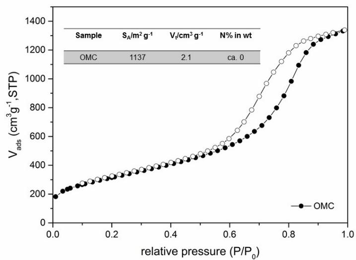
**Figure S10.** N<sub>2</sub> adsorption isotherm for N-free ordered mesoporous carbon OMC and the pore information (inset).
