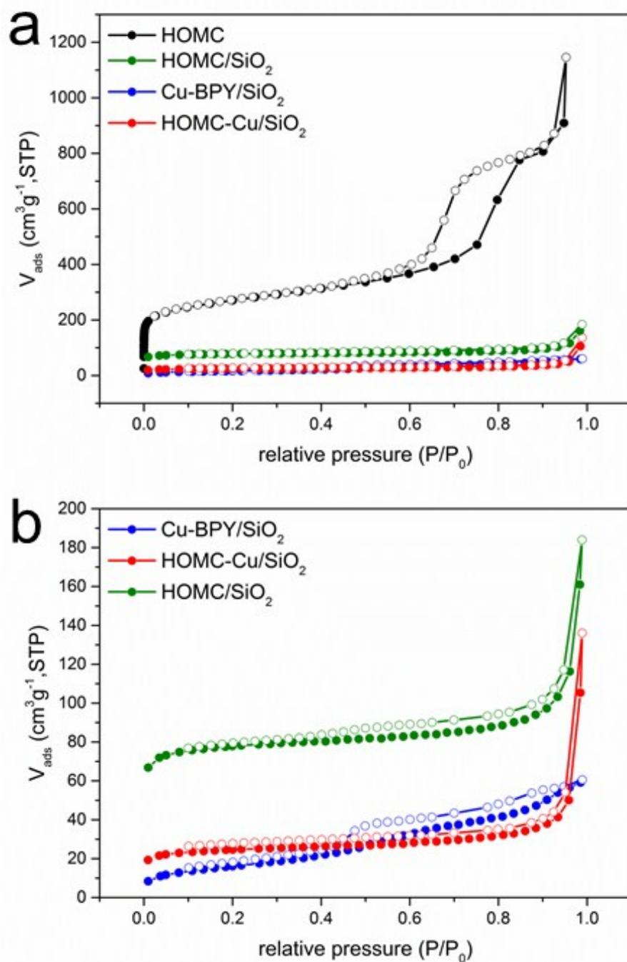
**Figure S6.** (a) N<sub>2</sub> physisorption of HOMC and (b) the corresponding intermediates along the preparation steps.
