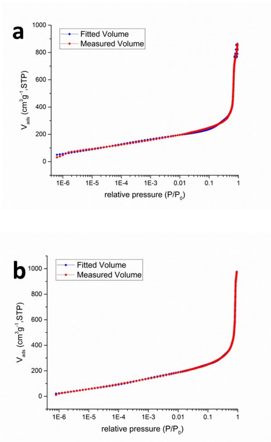
**Figure S7** QSDFT fitting of the theoretical isotherm based on the slit/cylindrical adsorption branch kernel and the measured isotherm for  $N_2$  adsorption at 77 K (a) and QSDFT fitting of
