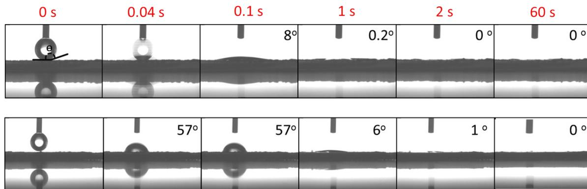
**Figure S11.** Dynamic contact angle: Comparison between HOMC (top) and PCC (bottom), which has only micropores. Both of the carbon materials have the same carbon and nitrogen precursor.
