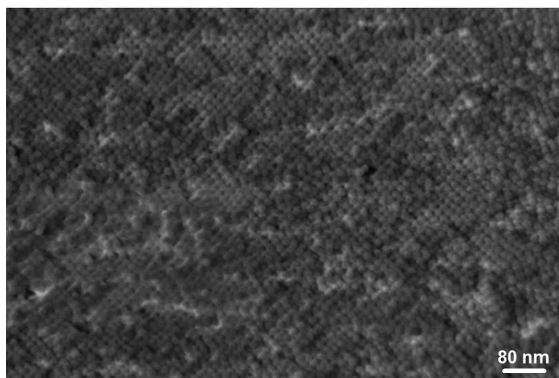
**Figure S5.** SEM images of silica spheres. Stacking faults can be found randomly in the images.
