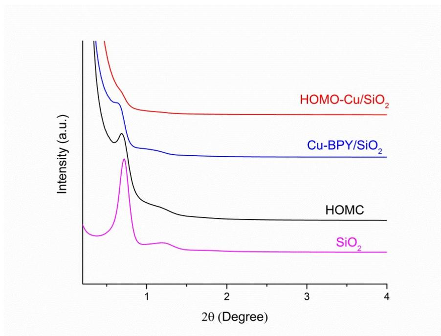
**Figure S4.** Small Angle X-Ray Scattering of the silica template, hydrophilic ordered mesoporous carbon HOMO-C, the obtained polymer/silica mixture Cu-BPY/SiO<sub>2</sub> and the obtained HOMO-Cu/SiO<sub>2</sub> composite after pyrolysis. They show distinguishable but poorly-resolved diffraction peaks, indicating that the inherited ordering from silica template is attenuated by the surrounded coordination polymer or carbon.
