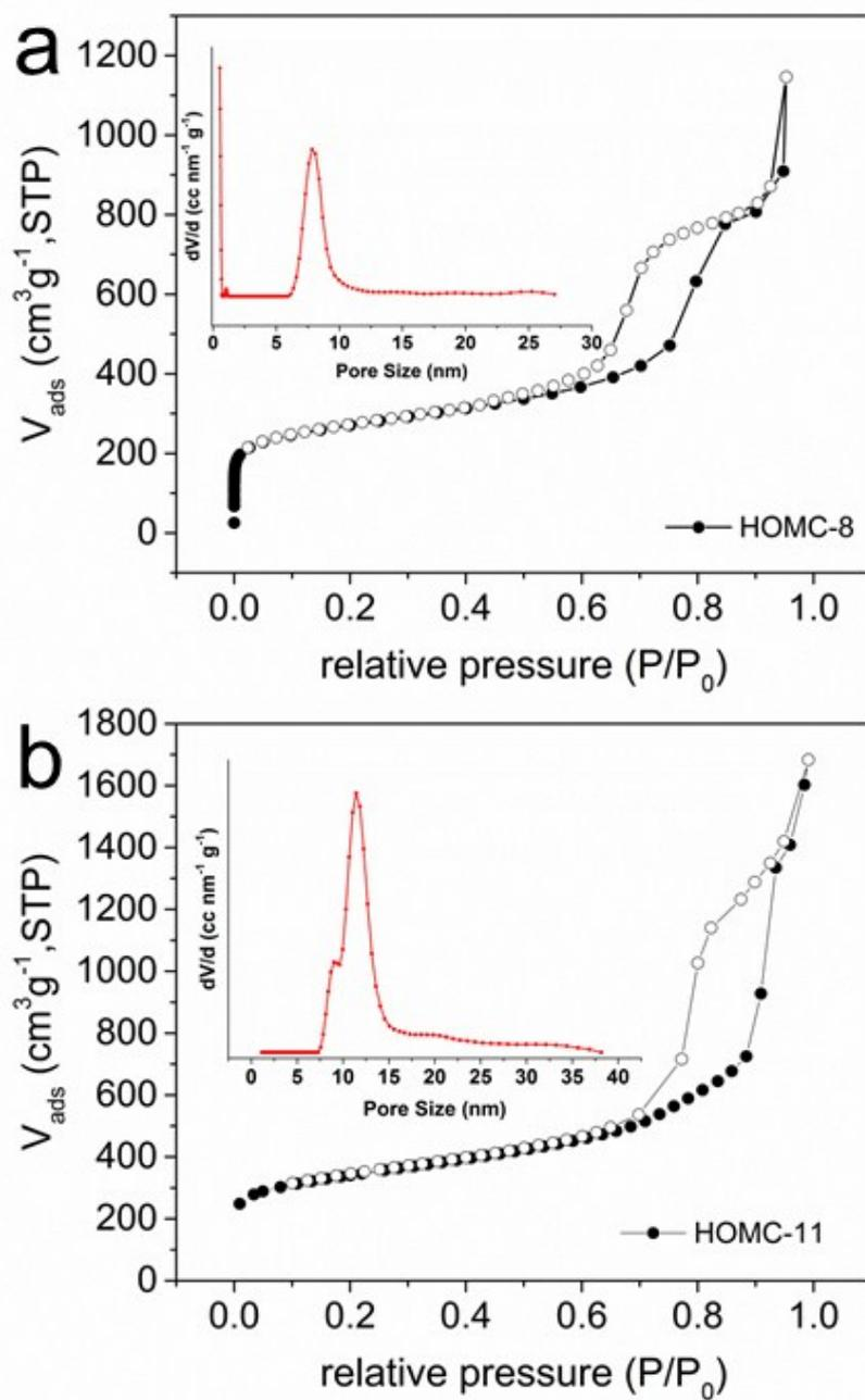
**Figure S9.**  $N_2$  adsorption isotherm of HOMC (top) and HOMC-11nm (bottom) with larger silica template. Inset: the pore size distribution.
