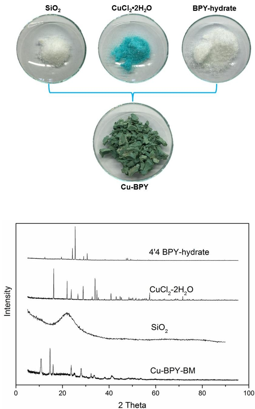
**Figure S1** The precursor and the product of the coordination polymer (a) and the corresponding XRD patterns (b). An obvious color change can be observed. From the XRD patterns we can see a phase formed after the ball milling, i.e. the Cu-BPY coordination polymer.
