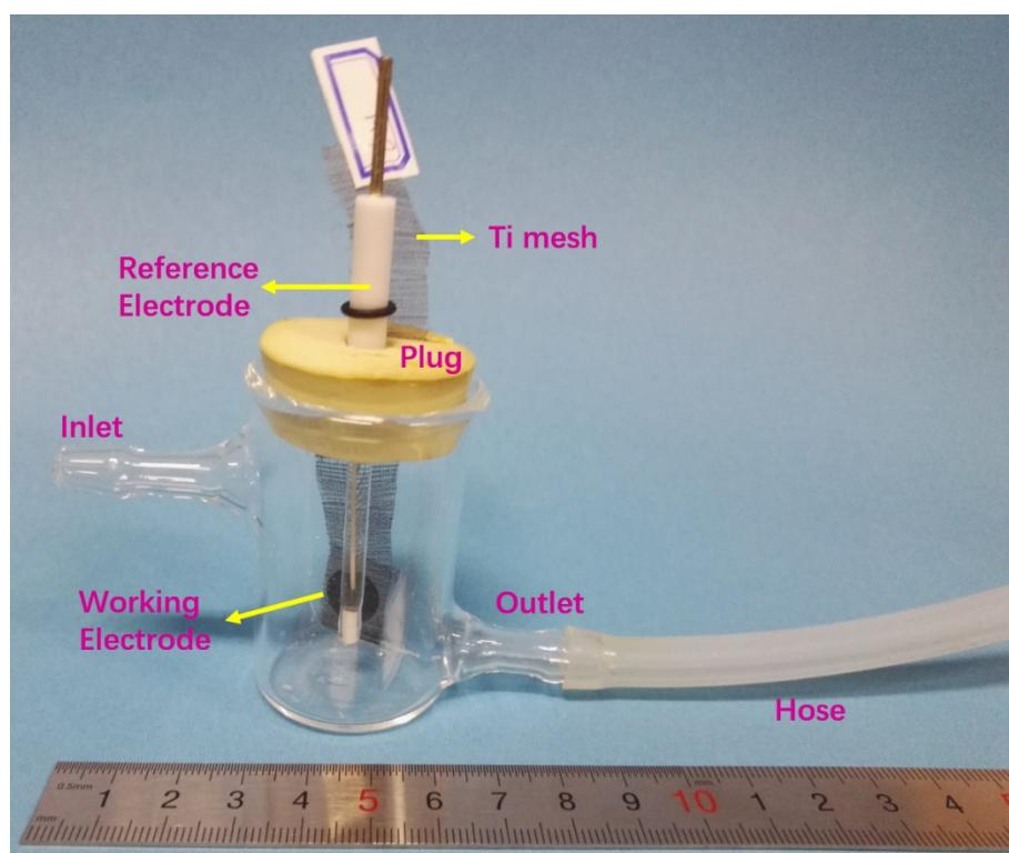
**Fig. S1** Photograph of the device for OCP measurements. The HC and LC solutions alternately flow into and out of the tank via the inlet and outlet, respectively. The working electrode and the Ag/AgCl reference electrode are in the tank. The hose connected with the outlet can be used to adjust the height of the liquid level by changing the height of its tail end.
