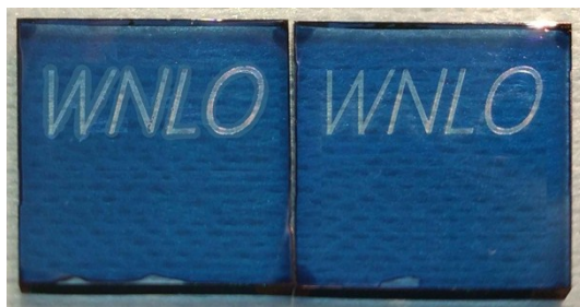
Figure S6. Patching trace of PVA on deliberately created defects (WNLO shape) on the PBDB-T:ITIC films (the left is patched, and the right is not patched).
