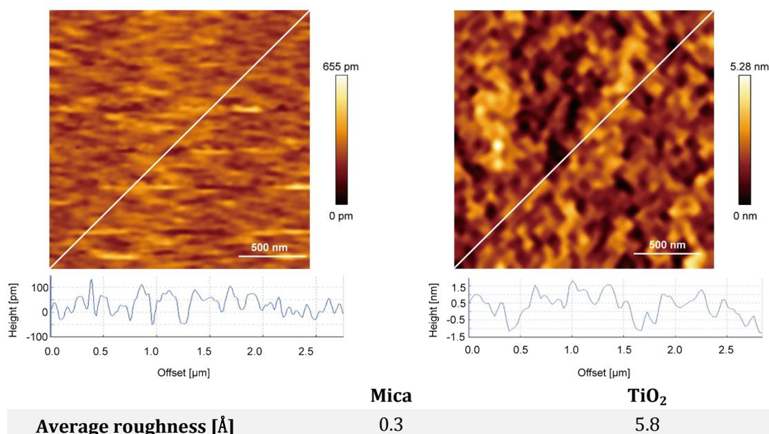
**Figure S5. Surface roughness of Mica (left) and TiO<sub>2</sub> (right) evaluated by AFM imaging.** The images were obtained at room temperature by a NanoWizard II AFM (JPK, Germany) operating in intermittent contact mode. Surface roughness of the two substrates were automatically evaluated by a commercial
