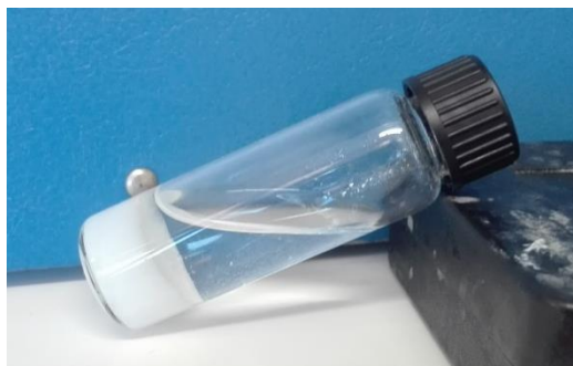
Figure S13. Experimental systems used to determine kinetic of CPT release from gel matrix: a) hybrid gel; b) pure gel.
