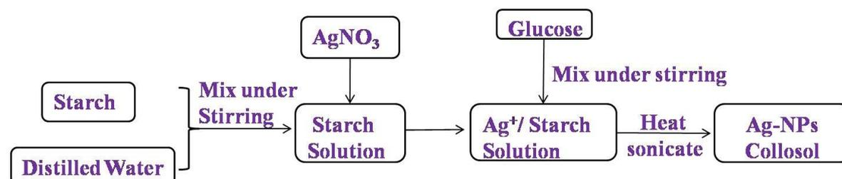
**Figure S1:** The schematic diagram of the green preparation process of small sized Ag-NPs collosol.
