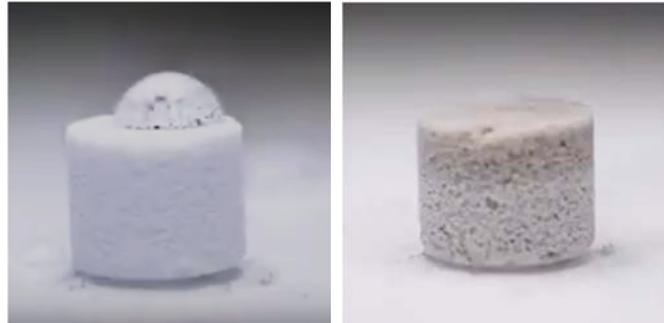
**Figure S5.** A water droplet deposited on bare (left) and ND treated ChronOS (right). In the case of ChronOS+ND the water droplets are immediately uptaken by the scaffold material (darker shade in the upper third of the scaffold sample).
