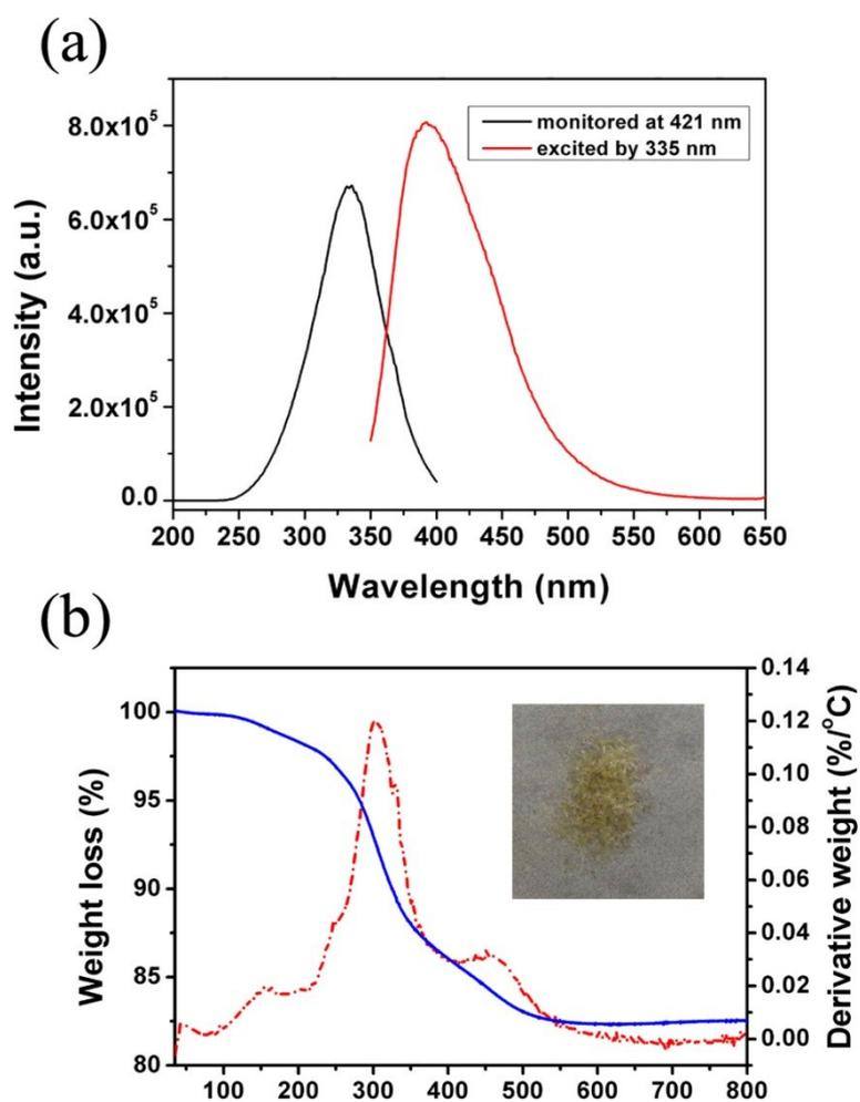
Figure S7. (a) PL excitation spectrum (monitored at 421 nm) and PL emission spectrum (excited by 335 nm) of the carbon black and amorphous silica derived sample; (b) TG and DTG curves of the carbon black and amorphous silica derived sample; the inset of (b) shows the optical photograph of the obtained control sample.
