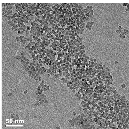
Figure S2. TEM image of the as-obtained Silica-C NPs in a relatively low magnification to verify their uniform morphology.
