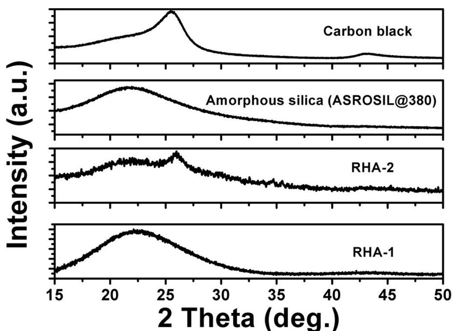
Figure S6. XRD patterns of the carbon black, amorphous silica, and RHA (1: obtained by treating RHs in a mixed gas of air and N<sub>2</sub>; 2: obtained by treating RHs in N<sub>2</sub>).
