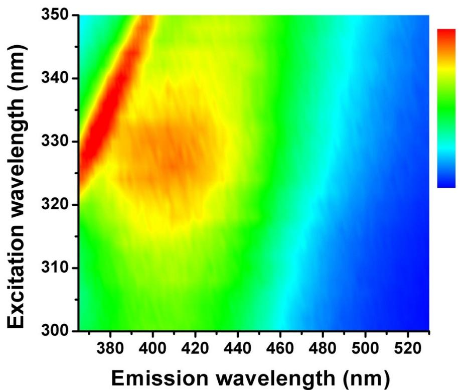
Figure S3. PL mapping image of the RH derived carbon QDs measured at 25 °C. The carbon QDs were prepared under the same experimental conditions as those of Silica-C NPs, except changing the RHA to RH carbon (RHC) extracted from RHs.
