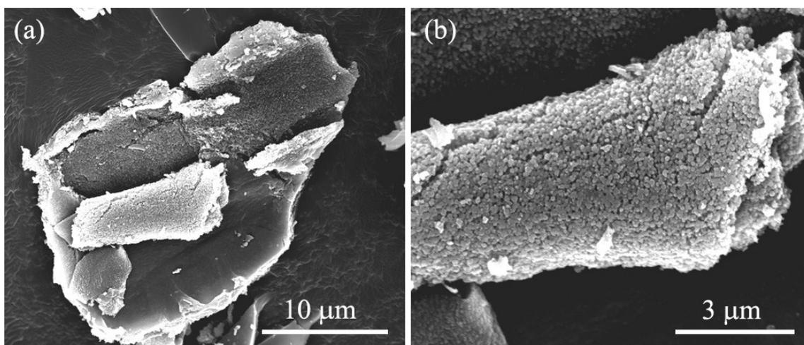
Figure S1. SEM images of RHA in low magnifications.
