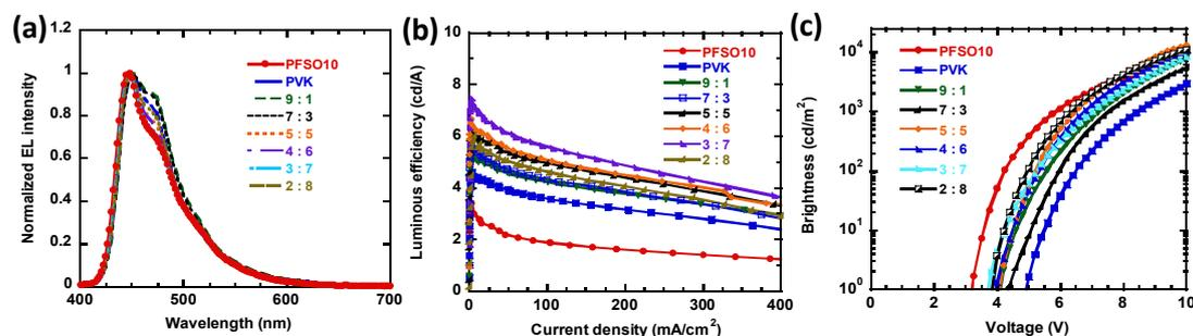
**Figure S2.** The electroluminescent spectra (a), luminous efficiency–current density (b) and luminance–voltage (c) characteristics of devices.
