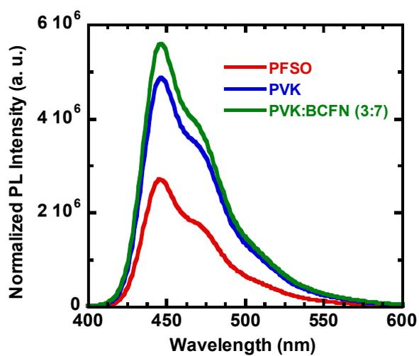
**Figure S3.** The PL spectra of PFSO (80 nm) films processed on quartz/PEDOT:PSS with or without 20 nm PVK or PVK:BCFN = 3:7 as hole transport layer.
