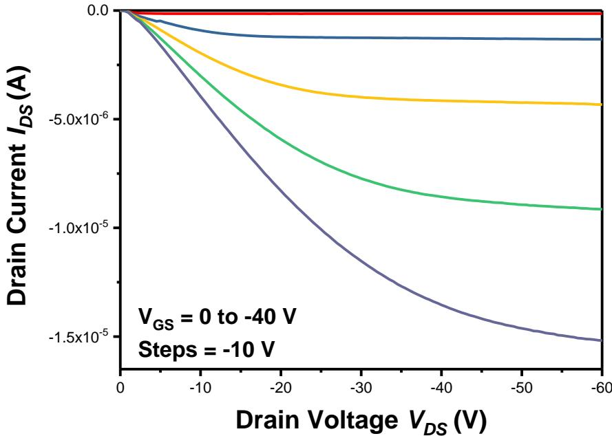
**Figure S6.** Output characteristics of rubrene single crystal transistor.
