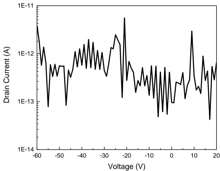
**Figure S7.** Transfer characteristics of **rubrene-Ox2** device.
