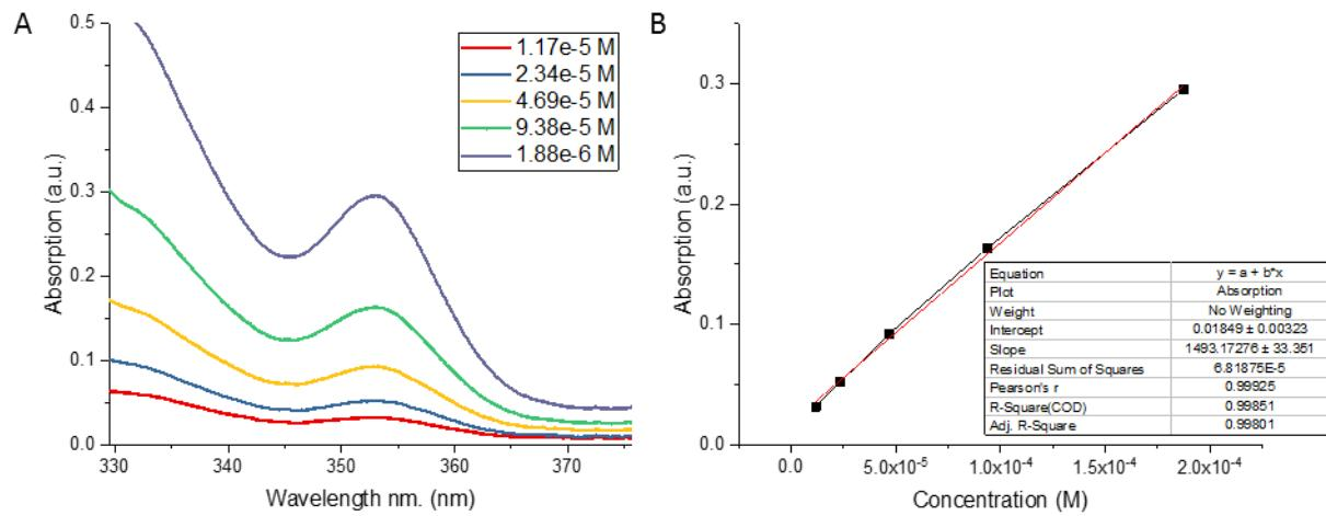
**Figure S4.** A) Rubrene-Ox2 concentration absorption sweep and B) Absorption coefficient of rubrene-Ox2 determined at 353 nm.
