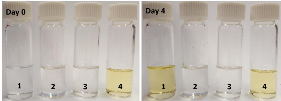
**Figure S1.** 5 mg of Rubrene-Ox1 were mixed dissolved in (1) chloroform, (2) toluene, (3)  $\text{Na}_2\text{CO}_3$  treated chloroform, and (4)  $\text{Na}_2\text{CO}_3$  treated choroform with Methanesulfonic acid.
