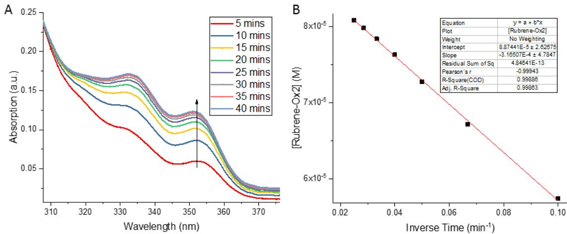
**Figure S5.** A) UV-Vis of rubrene-Ox1 to rubrene-Ox2 reaction with equimolar amounts of external acid and B) rubrene-Ox2 plotted against inverse time.
