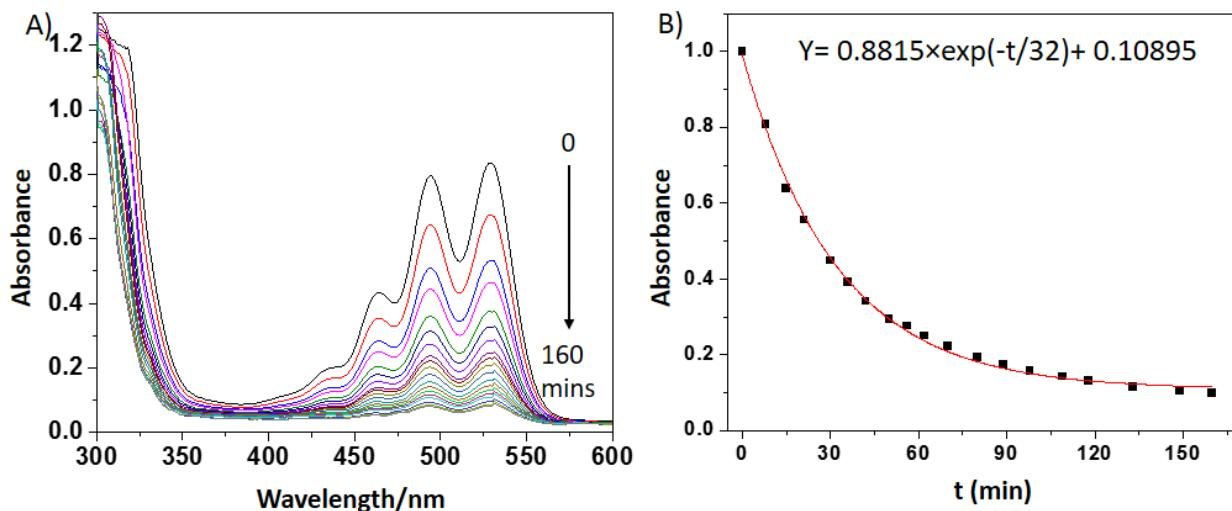
**Figure S3.** A)UV-vis spectra of rubrene in  $\text{CHCl}_3$  recorded at regular interval (10 mins) during exposure to light, B) The absorbance intensity vs exposure time.
