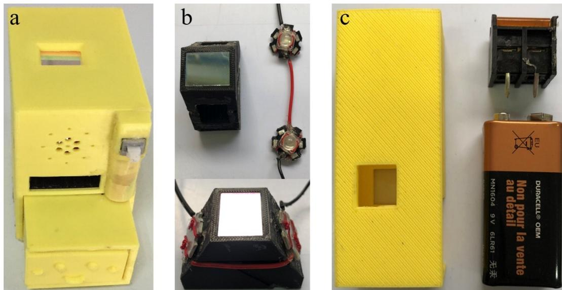
**Figure S1.** Schematic illustrations demonstrating (a) Scheme of 3D-printed read-out platform; (b) The composed of core component, included two LED lights and an optical filter; (c) The battery case consisted of lithium ion and a switch.
