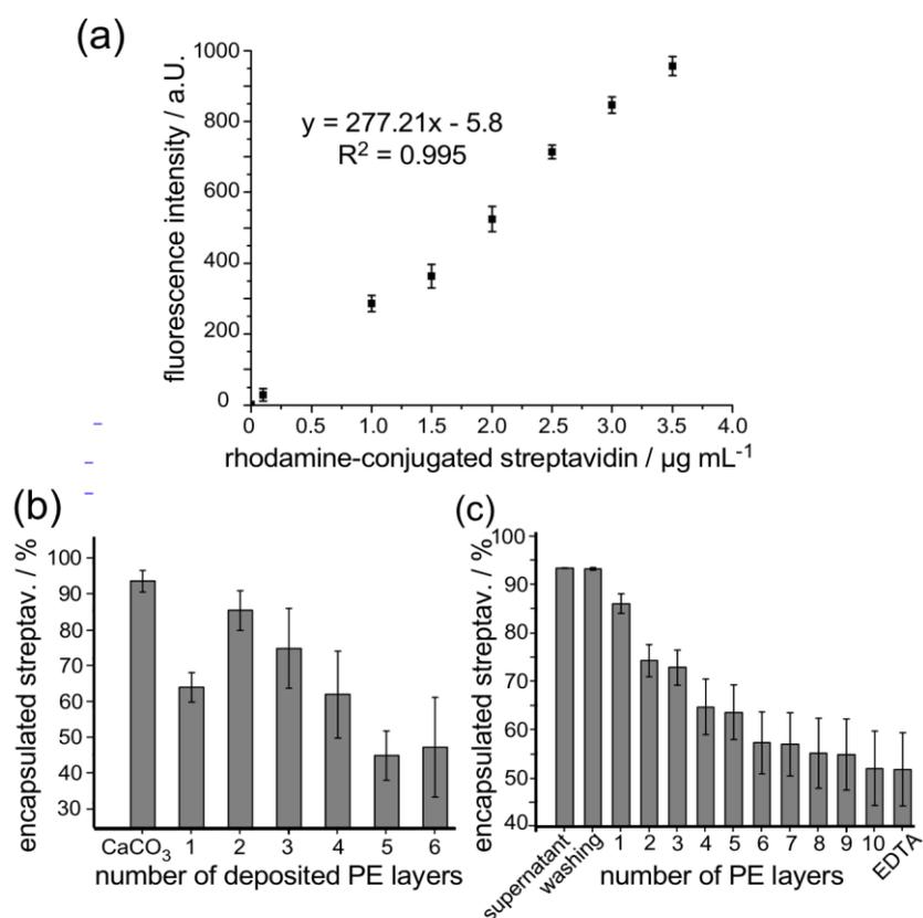
**Figure S-3.4** (a) Calibration curve for rhodamine-conjugated streptavidin. Encapsulation efficiency (in %) of fluorescent streptavidin was measured (b) directly from the particle suspension, or (c) by the amount of streptavidin released into PE, washing and EDTA solutions during the LbL process.
