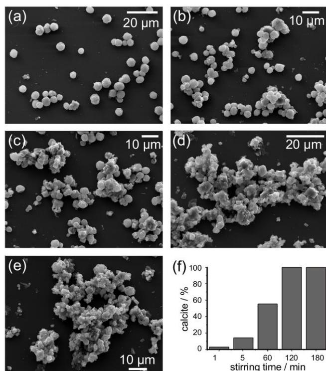
**Figure S-2.1** SEM images of  $\text{CaCO}_3$  microparticles obtained after different stirring periods during the synthesis process. (a) Spherical particles (vaterite) crystals obtained after mixing for 1 and (b) 5 min; (c) a mixture of spherical particles (vaterite) and rhombohedral microcrystals (calcite) obtained after stirring for 1 h; (d) rhombohedral microcrystals (calcite) obtained when stirring for 2 h and (e) 3 h. (f) Calcite microcrystal amount (%) as a function of stirring time.
