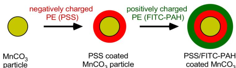
**Figure S1.1** Schematic of the coating of  $\text{MnCO}_3$  particles with alternating PE assembly of FITC-PAH and PSS. The  $\text{MnCO}_3$  particles were exposed to a fluorescently-labelled, positively charged PE (FITC PAH) to deposit the first PE layer. The excess PE was removed by the cycles of centrifugation and washing steps before the second layer of negatively charged PEs (PSS) was added.
