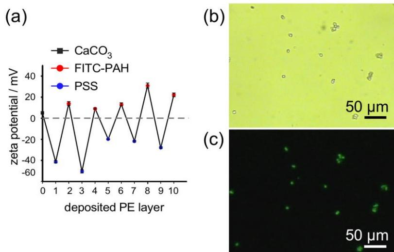
**Figure S-2.3** LbL deposition of PE (PSS/FITC-PAH)<sub>5</sub> on  $\text{CaCO}_3$  microparticles. (a) The particles zeta potential alternates as a function of the number PE layers deposited ( $n=3$ ). (b) Bright field image and (c) fluorescence microscope image of  $\text{CaCO}_3$  microparticles coated with 10 layers of FITC-PAH/PSS polyelectrolyte.
