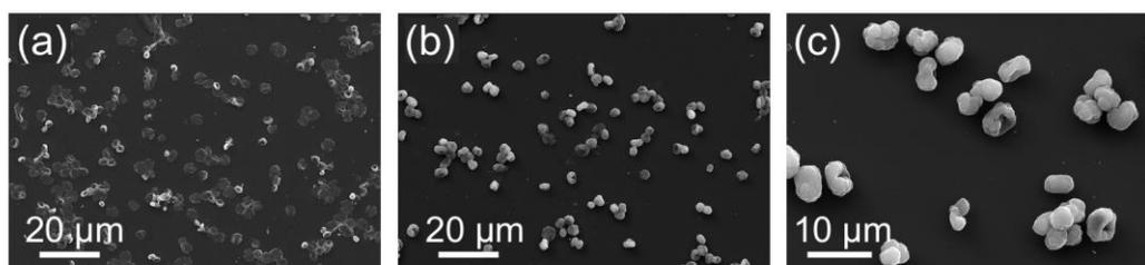
**Figure S-2.4** SEM images of LbL formed PE microcapsules with particles core dissolved by EDTA solution. (a) Two-bilayered PE microcapsules forming a thinner shell. (b) Six-bilayer PE microcapsules with a thicker shell. (c) Ten-bilayer PE  $\text{CaCO}_3$  particles with the majority of  $\text{CaCO}_3$  cores not dissolved.
