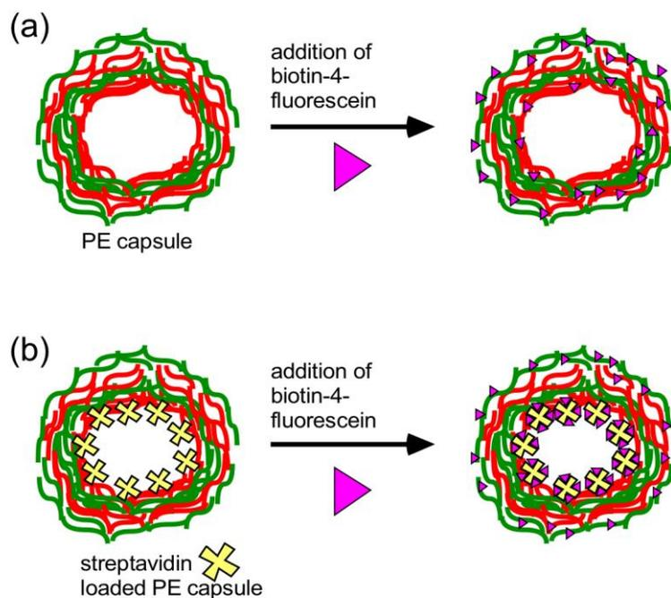
**Figure S-4.1** Concept of streptavidin-biotin assay in LbL capsules templated from  $\text{MnCO}_3$  and  $\text{CaCO}_3$  microparticles. (a) Biotin-4-fluorescein solution was added to capsules not containing streptavidin as a control and (b) to PE capsules filled with streptavidin.
