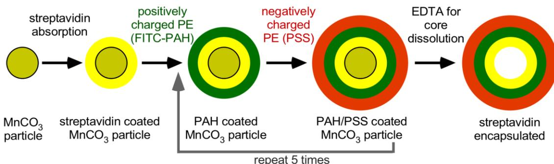
**Figure S-3.1** Streptavidin was loaded directly onto the  $\text{MnCO}_3$  microparticles, followed by deposition of alternating layers of polyelectrolytes, namely the cationic PAH and the anionic PSS. Five bilayers were deposited.
