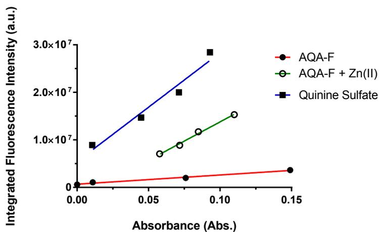
**Figure S 2:** Plot of absorbance against integrated fluorescence intensity for **AQA-F**, **AQA-F + 1 equivalent Zn(II)Cl<sub>2</sub>**, and quinine sulfate ( $\lambda_{ex}=320$  nm).
