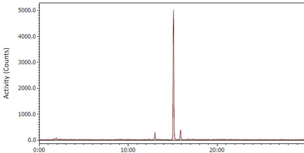
**Figure S 12:** Radio-HPLC chromatogram for crude radiolabelling mixture of **8** incubated with  $[^{18}\text{F}]\text{F}^-$  prior to addition of TFA radiochemical conversion = 82.6%
