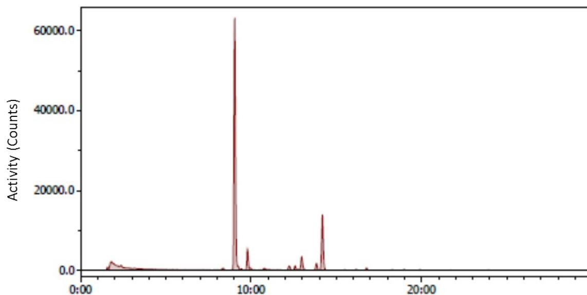
**Figure S 13:** Radio-HPLC chromatogram for crude radiolabelling mixture of **8** incubated with  $[^{18}\text{F}]\text{F}^-$  15 minutes after addition of TFA radiochemical conversion = 54.3%
