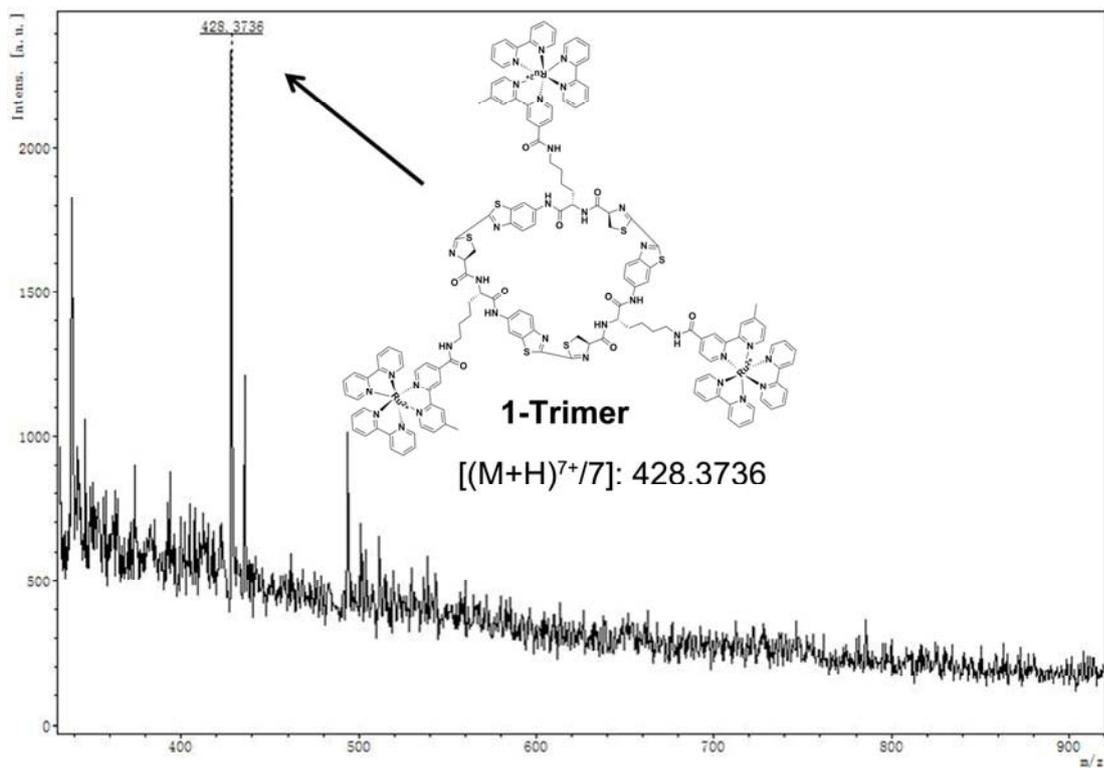
**Figure S9.** HR-MALDI-TOF/MS spectrum of HPLC peaks at 27.1 min (**1-Trimer**) in Figure 2D.
