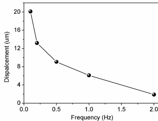
Fig. S2 Actuation displacement as a function of frequency of the catheter.
