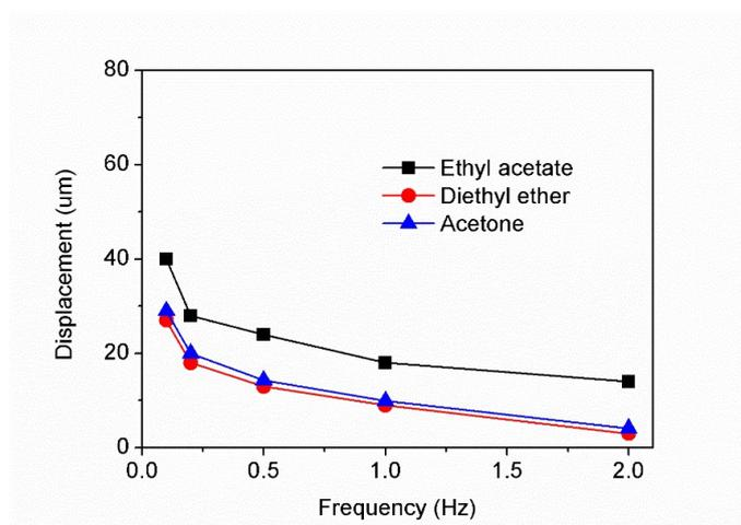
Fig. S6 Actuation displacement as a function of frequency of catheters regulated by diethyl ether, ethyl acetate and acetone, respectively.
