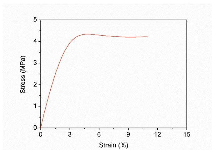
Fig. S7 Stress-strain curve of Nafion treated with pure water under the same condition.
