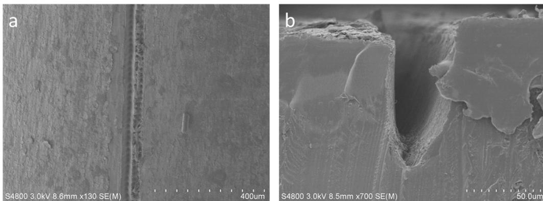
Fig. S1 Surface and cross-sectional SEM images of the electrode incision caused by laser micro-dissection.
