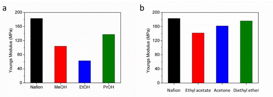
Fig. S4 a) Young's Modulus of Nafion tubes regulated by methanol, ethanol and propanol, respectively. b) Young's Modulus of Nafion tubes regulated by diethyl ether, ethyl acetate and acetone, respectively.
