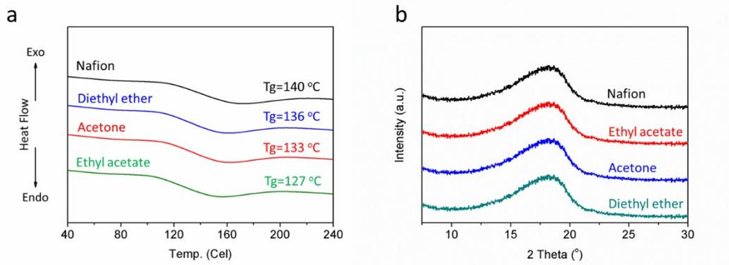
Fig. S3 a) DSC traces and b) XRD patterns of Nafion tubes regulated by diethyl ether, ethyl acetate and acetone, respectively.
