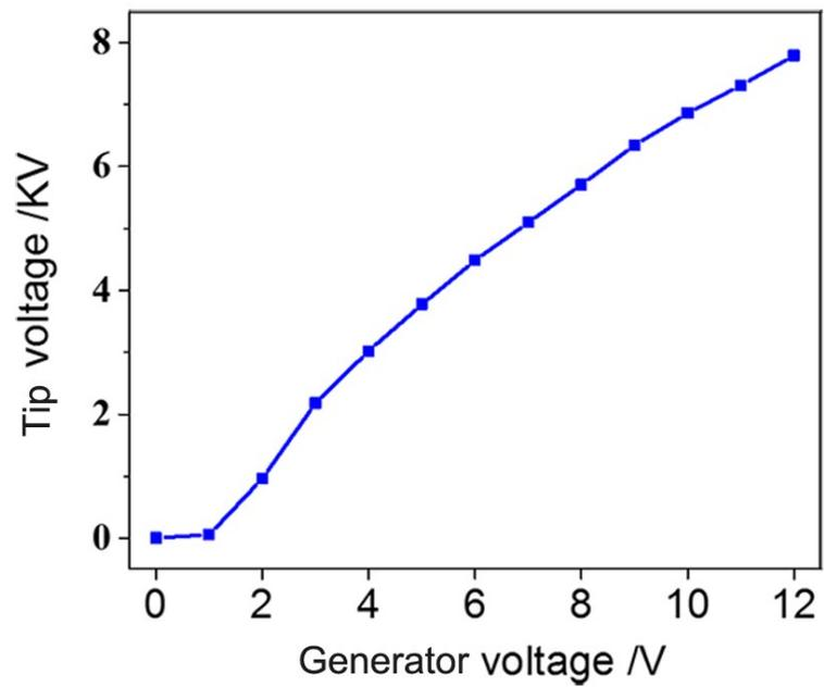
**Figure S2** Characterization of the tungsten-tip voltage (absolute voltage) versus the output voltage from NAIs generator.
