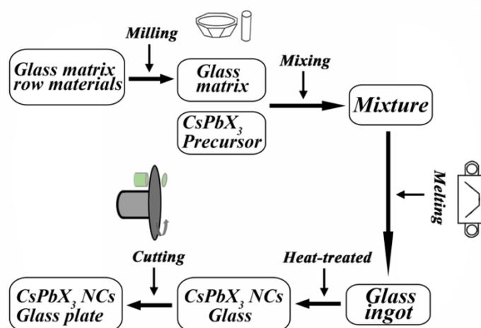
Fig. S1. Schematic of fabrication of the  $\text{CsPbX}_3$  NCs glasses.
