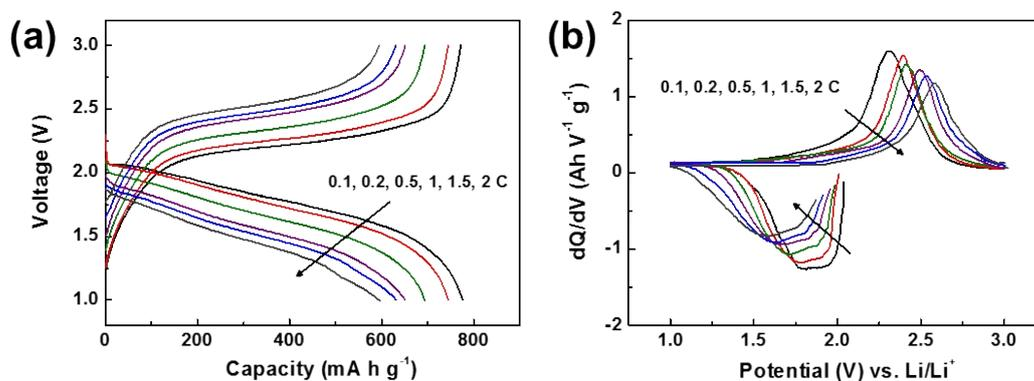
Fig. S5 Discharge/charge curves of SPANI cathode at different rates and the corresponding differential capacity plots.
