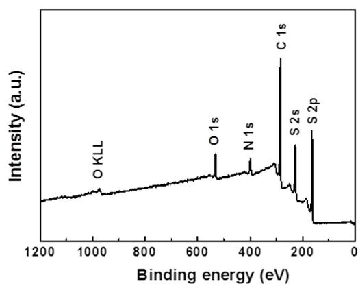
Fig. S2 Overall XPS spectrum of the SPANI sample, which shows the elements of carbon, oxygen, nitrogen and sulfur.
