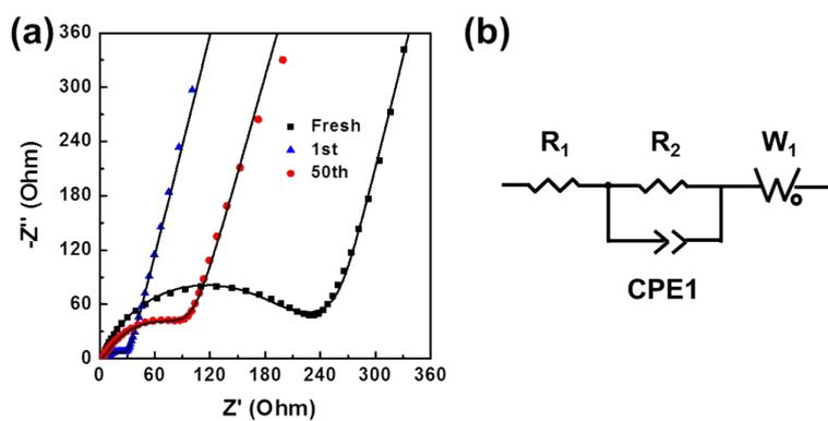
Fig. S7 (a) EIS plots of SPANI cathode after different cycles at 1 C. Solid lines in (a) are fitted to the equivalent circuit (b).
