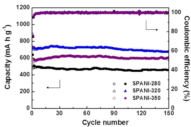
Fig. S4 Cycling test of SPANI samples prepared at different temperatures at 0.25 C (0.1 C for the 1st cycle).
