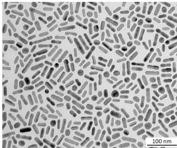
**Figure. S5** TEM image of AuCu<sub>3</sub> nanorods.
