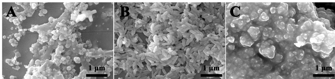
Figure S1. SEM images of (A) Fe<sub>2</sub>O<sub>3</sub> nanoparticles, (B) spindle-like Sn-doped Fe<sub>2</sub>O<sub>3</sub> nanoclusters and (C) bare SnO<sub>2</sub> after 50 discharge/charge cycles.
