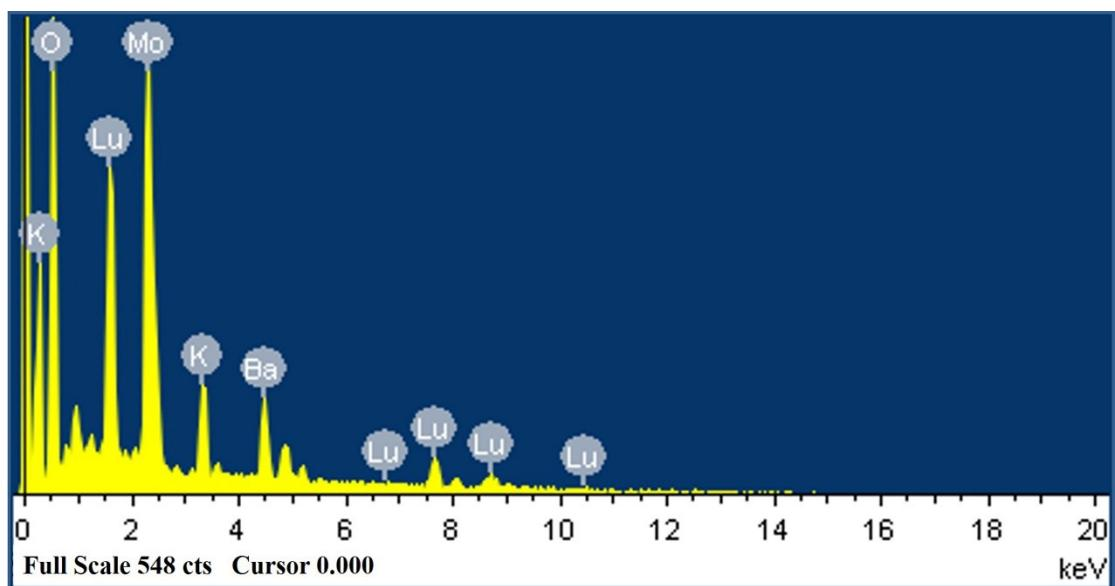
Fig. S1. EDX spectrum of  $\text{KBaLu}(\text{MoO}_4)_3$  crystal.
