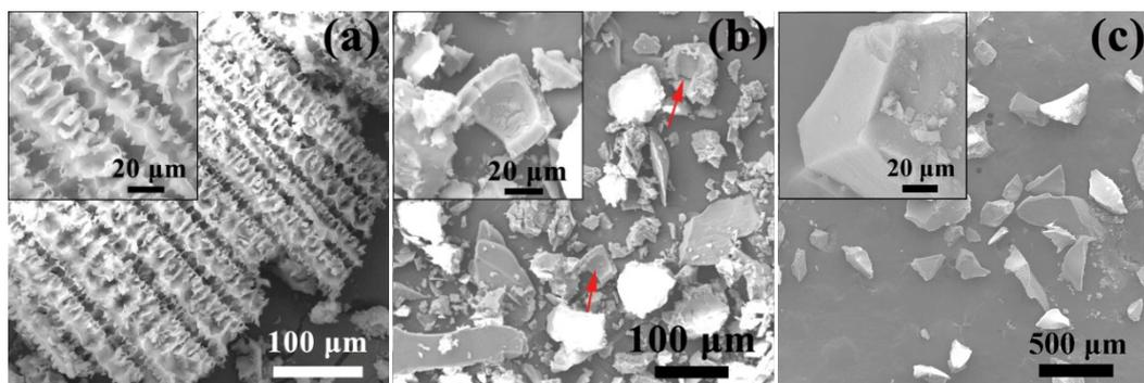
**Figure S5.** SEM images of froze samples dried by (a) supercritical CO<sub>2</sub> or (b) solvent evaporation at room temperature, (c) SEM image of sample dried by supercritical CO<sub>2</sub> directly without freezing.
