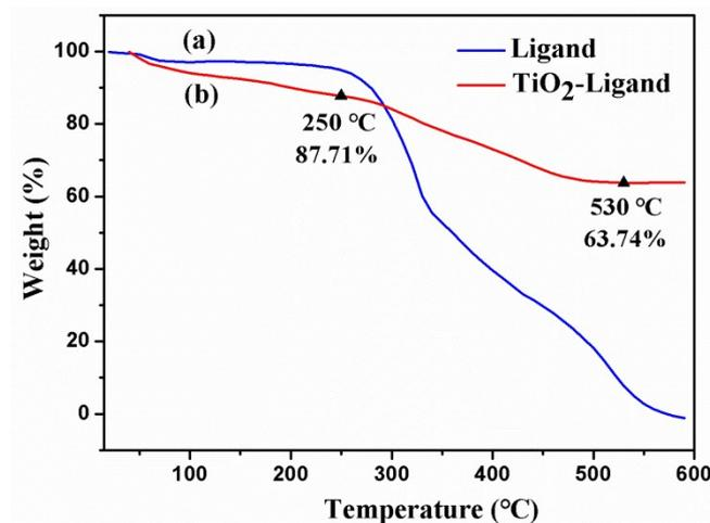
**Figure S3.** TGA curve of (a) ligand and (b) TiO<sub>2</sub>-ligand nanoparticles.
