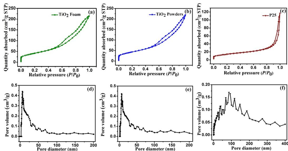
**Figure S7.** Nitrogen physisorption isotherms and the corresponding pore-size distributions for TiO<sub>2</sub> foam (a) (d), TiO<sub>2</sub> Powders (b) (e), and P25 (c) (f).
