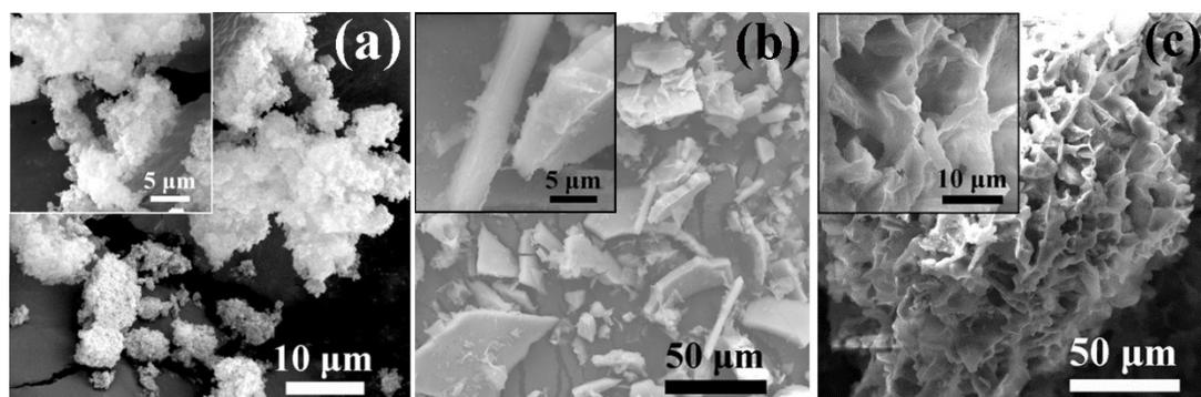
**Figure S6.** SEM images of samples obtained by centrifuging and freeze drying of suspension of (a) naked TiO<sub>2</sub> particles and (b, c) 2-bromo-N-(3, 4-dihydroxyphenethyl)-2-methylpropanamide-grafted TiO<sub>2</sub> in benzene.
