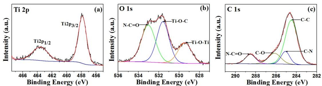
Figure S2. High-resolution XPS spectra of elements of TiO<sub>2</sub> nanoparticles: (a) Ti 2p, (b) O 1s, (c) C 1s.
