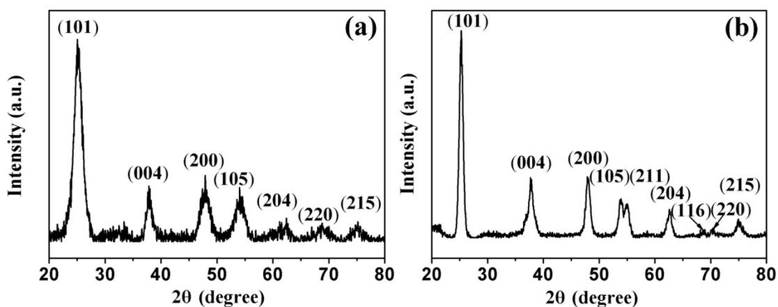
Figure S1. XRD pattern of TiO<sub>2</sub> NPs (a) before and (b) after annealing.
