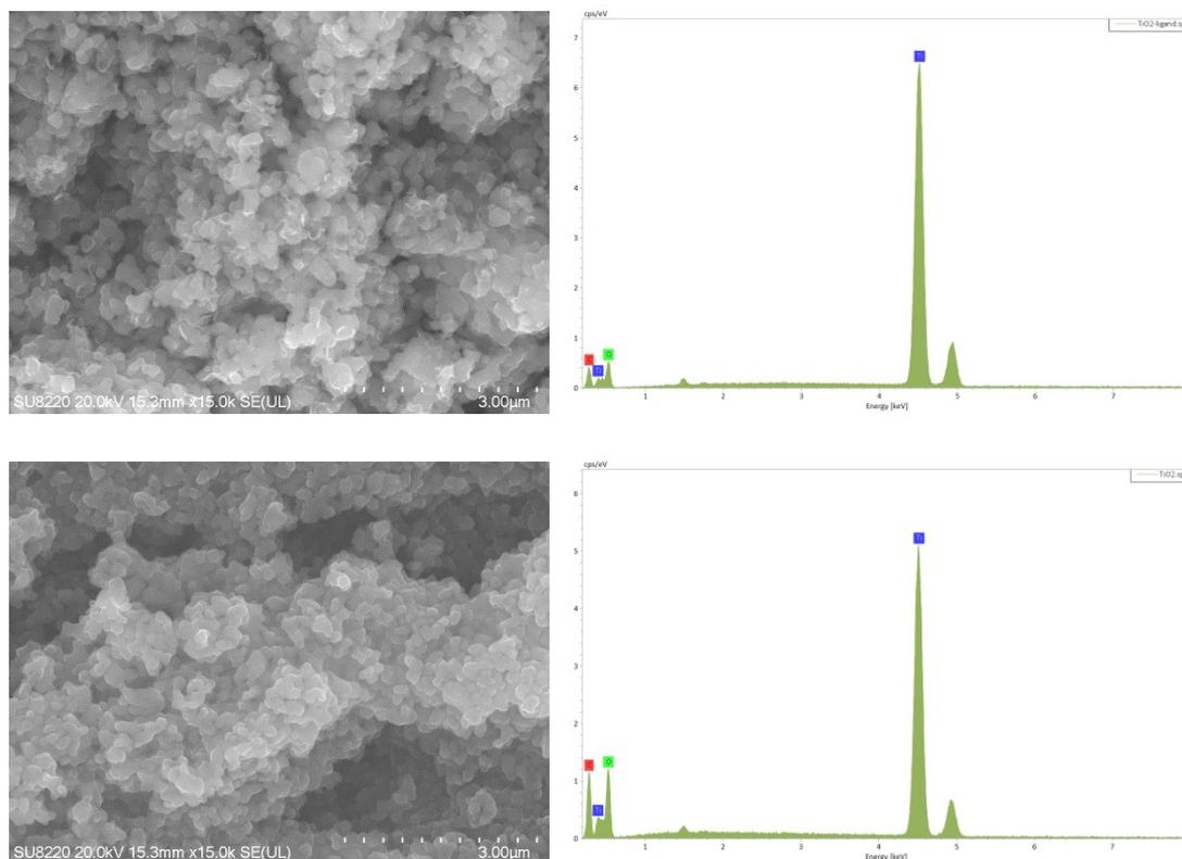
**Figure S4.** FESEM images and EDX spectra of backbone of TiO<sub>2</sub> foam before (up) and after (down) annealing.
