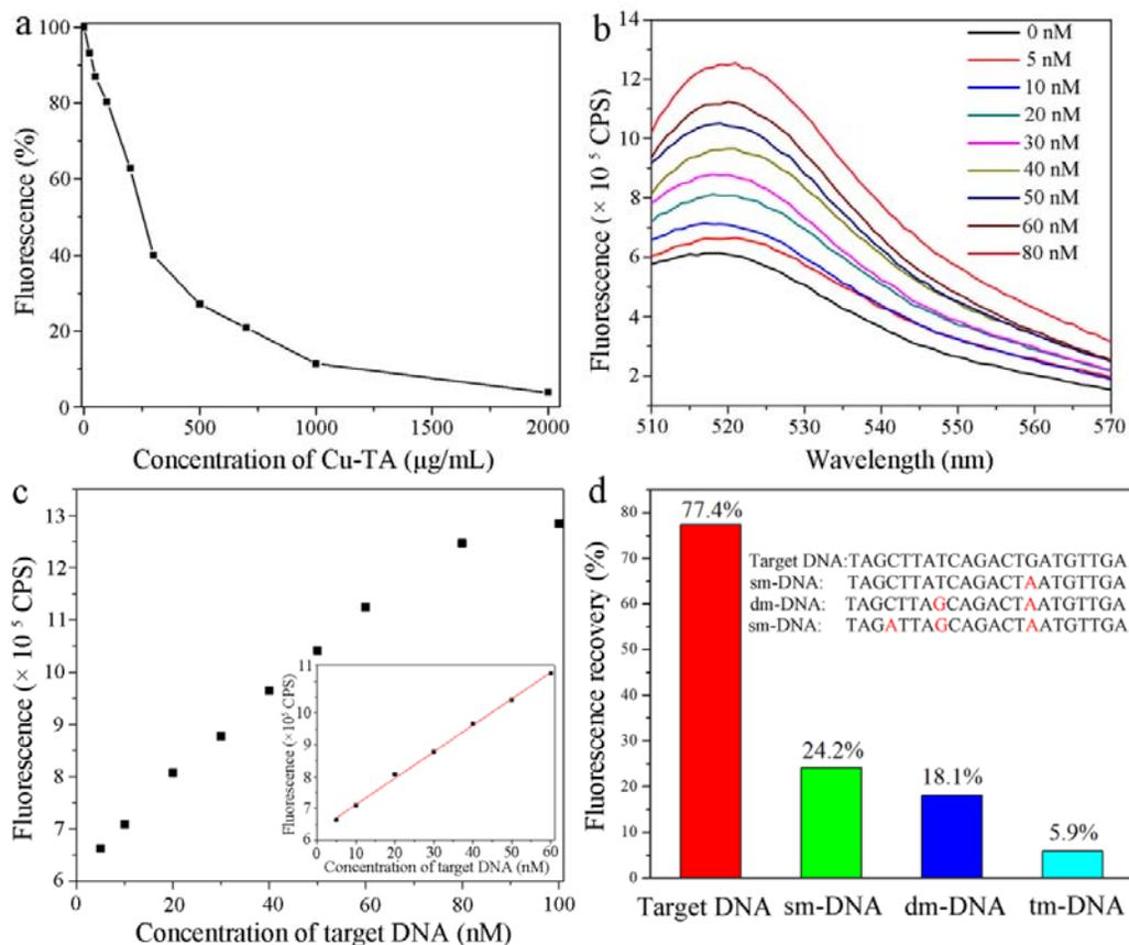
**Figure S5** (a) Fluorescence intensities of probe DNA at 520 nm versus different concentrations of shuttle-like Cu-TA crystals. (b) Fluorescent recovery in different concentrations of target DNA solution (0-80.0 nM). (c) Fluorescence intensities versus different concentrations of target DNA (0.5-100 nM). Insets are corresponding calibration curve for target DNA detection. (d) Selectivity for the detection of DNA.
