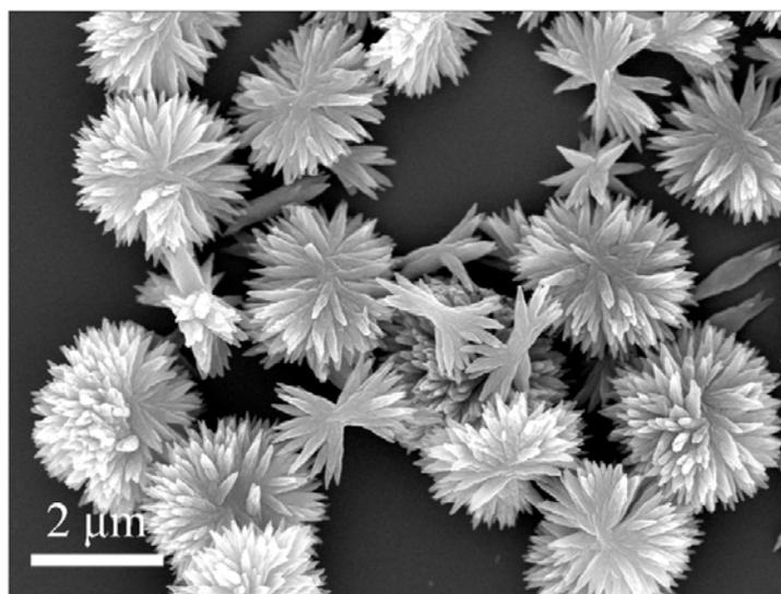
**Figure S1** SEM image for urchin-like Cu-TA synthesized when the amounts of ammonia is 0.8 mL.
