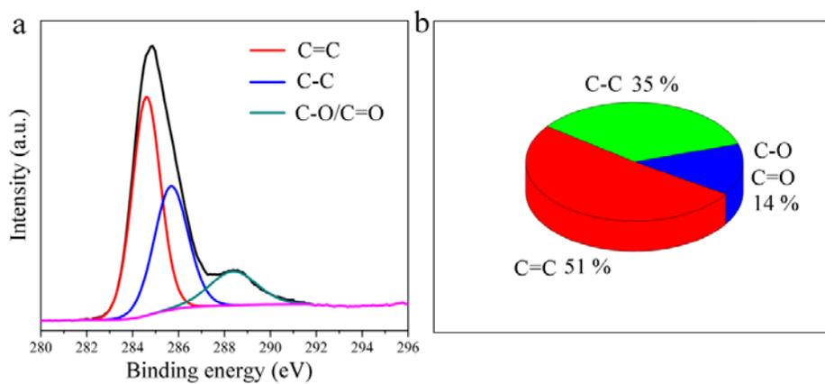
**Figure S4** (a) High resolution XPS spectra for C 1s. (b) The content (at %) of different kinds of carbon atoms.
