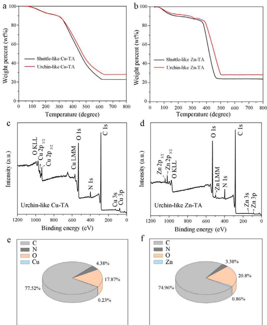
**Figure S3** TG curves for (a) Cu-TA crystals and (b) Zn-TA crystals. XPS spectra for (c) urchin-like Cu-TA and (d) Zn-TA crystals. The element contents in (e) urchin-like Cu-TA and (f) Zn-TA crystals calculated from XPS results.
