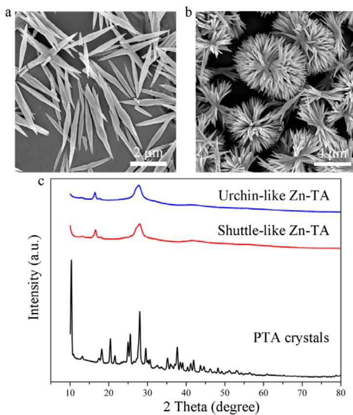
**Figure S2** SEM images for (a) shuttle-like and (b) urchin-like Zn-TA crystals. (c) XRD patterns of shuttle-like, urchin-like Zn-TA crystals, and PTA crystals synthesized without using any metal ions.
