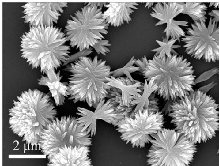
**Figure S1** SEM image for urchin-like Cu-TA synthesized when the amounts of ammonia is 0.8 mL.
