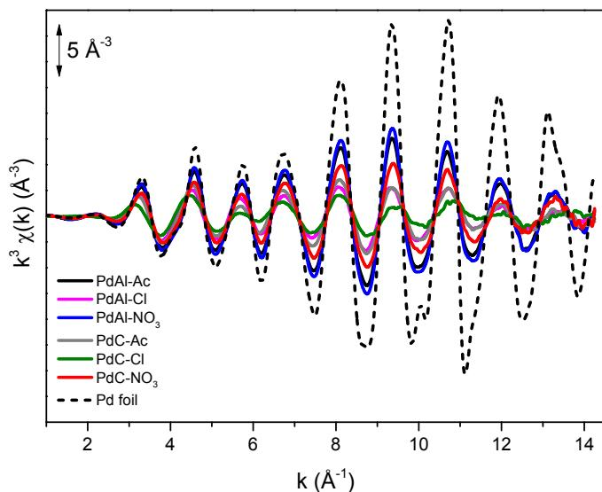
**Fig. S3.**  $k^3$ -weighted, phase-uncorrected  $\chi(k)$  functions of Pd-based catalysts during reduction in  $\text{H}_2$  at  $200^\circ\text{C}$ .
