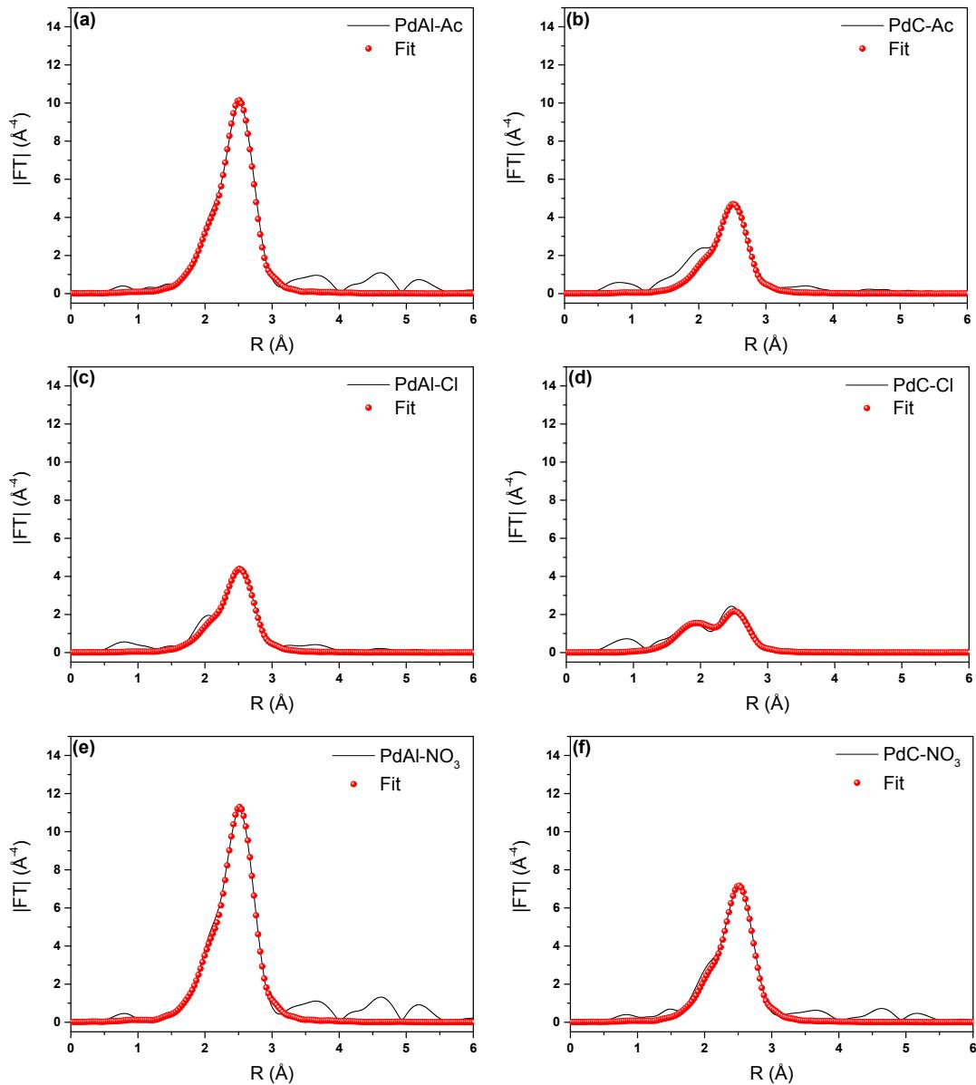
**Fig. S5.**  $|\text{FT}|$  of the  $k^3$ -weighted  $\chi(k)$  functions of catalysts during reduction in  $\text{H}_2$  at 200  $^{\circ}\text{C}$ : (a) PdAl-Ac (b) PdC-Ac (c) PdAl-Cl (d) PdC-Cl (e) PdAl- $\text{NO}_3$  (f) PdC- $\text{NO}_3$ .
