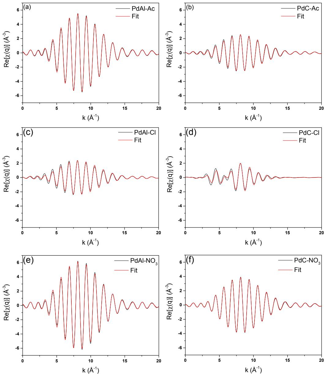
**Fig. S4.**  $k^3$ -weighted,  $\chi(q)$  functions ( $q$ -range = 2.2-3.0  $\text{\AA}$ ) of Pd-based catalysts during reduction in  $\text{H}_2$  at 200  $^\circ\text{C}$ : (a) PdAl-Ac (b) PdC-Ac (c) PdAl-Cl (d) PdC-Cl ( $q$ -range = 1.4-3.0  $\text{\AA}$ ) (e) PdAl- $\text{NO}_3$  (f) PdC- $\text{NO}_3$ .
