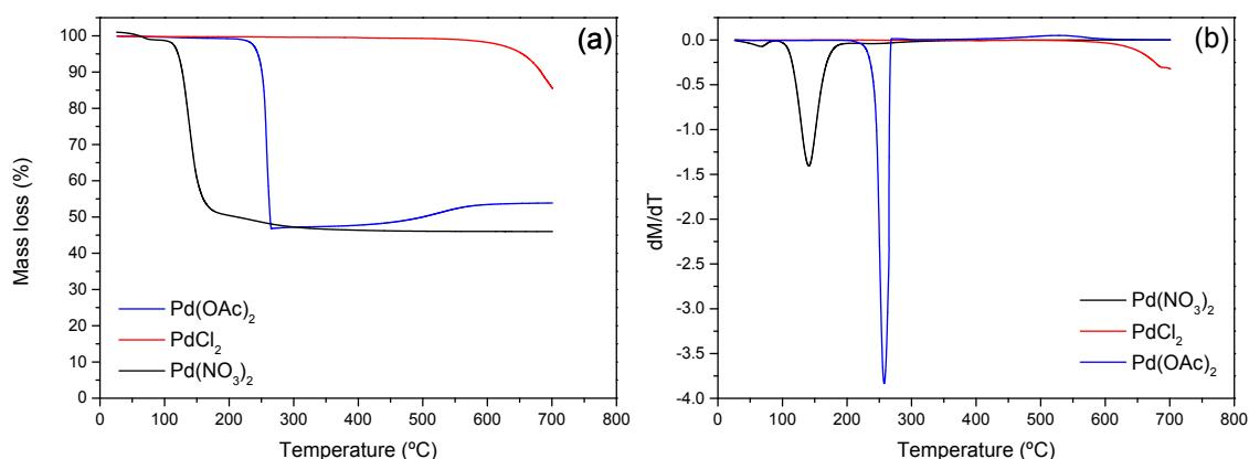
**Fig. S2.** Thermogravimetric analysis (a) and respective derivative (b) of Pd(OAc)<sub>2</sub>, PdCl<sub>2</sub> and Pd(NO<sub>3</sub>)<sub>2</sub> precursors.
