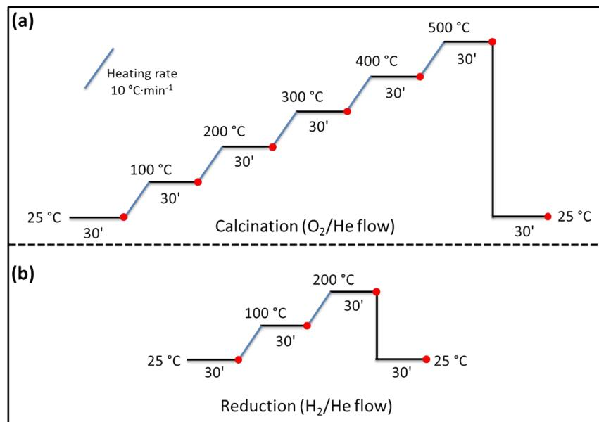
**Fig. S1.** Experimental steps used in the XAS study of Pd-based catalysts: (a) calcination under O<sub>2</sub>/He flow and (b) reduction under H<sub>2</sub>/He flow. Every red dot represents a set of 3 measurements.
