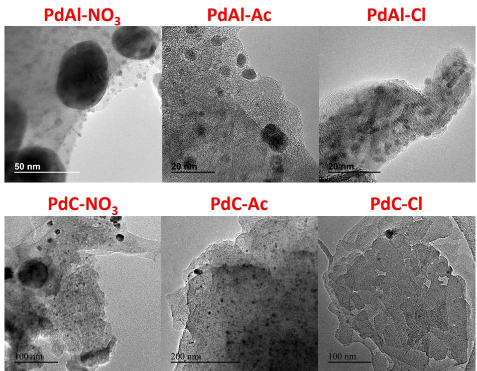
**Fig. S6.** TEM images of as-reduced Pd/Al<sub>2</sub>O<sub>3</sub> (top) and Pd/C (bottom) catalysts according the scheme reported in Fig.S1b.
