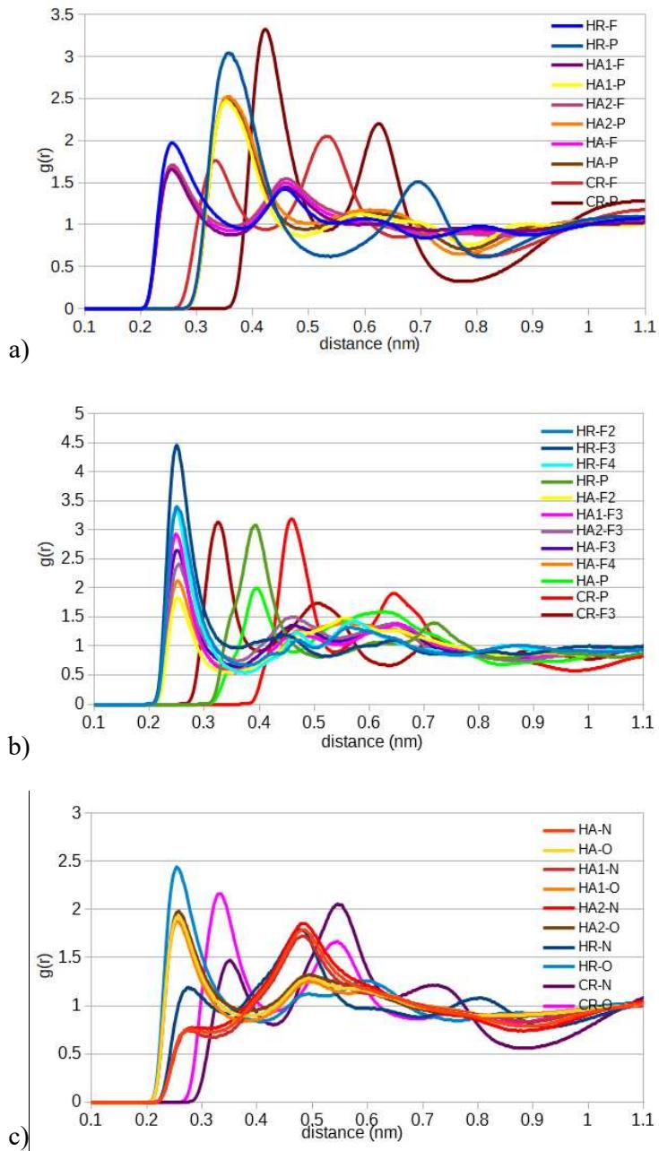
Figure S3. Atom-atom RDFs for between the most important sites of cation and anion  $[PF_6]^-$  (a),  $[FAP]^-$  (b) and  $[NTf_2]^-$  (c). As it can be seen, RDFs, involving atoms HA1 and HA2 are not distinguishable. Therefore, for further analysis the sites HA, HR, CR, as well as P and F for  $[PF_6]^-$ , O for  $[NTf_2]^-$ , and P and F3 for  $[FAP]^-$  were chosen.
