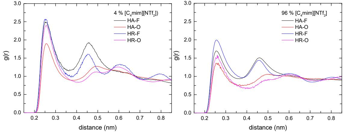
Figure S7. Radial distribution functions, HX-F and HX-O, for the  $[\text{C}_4\text{mim}][\text{PF}_6]/[\text{C}_4\text{mim}][\text{NTf}_2]$  mixture with a mole fraction of  $[\text{C}_4\text{mim}][\text{NTf}_2]$  of 4 % (a) and 96 % (b), derived from molecular dynamics simulation at 303 K.
