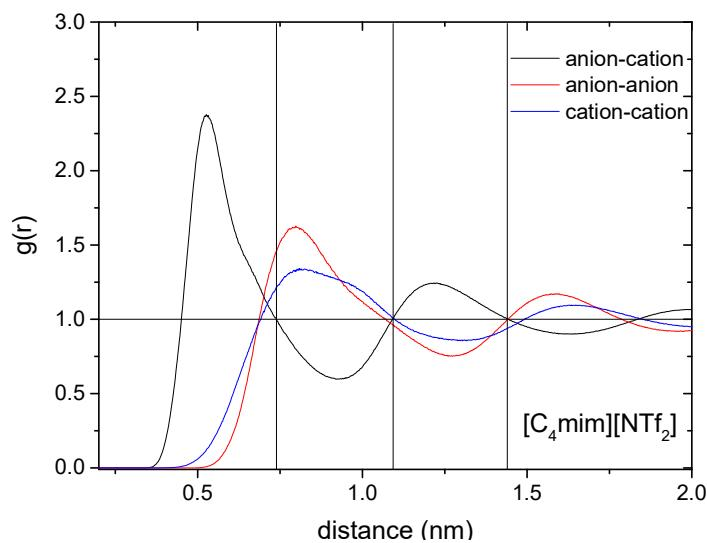
Figure S1. Period estimation – intersection with asymptote on the example of ionic liquid  $[C_4\text{mim}][\text{NTf}_2]$
