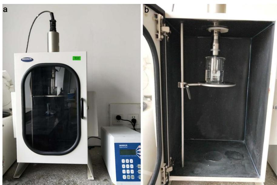
**Figure S1** a) The image; b) The internal structure of Ultrasonic cell Disruption System .
