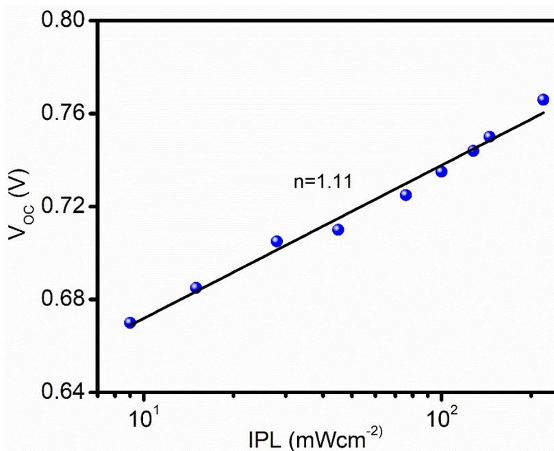
**Figure S2:** Shockley model; fit (solid lines) of the experimental data from Fig. 2a (symbols) by an Shockley diode model (For the comparison with charge transport model fitting plotted as in Fig 2a)
