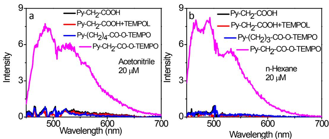
**Fig. S3** Fluorescence emissions spectra of Py-CH<sub>2</sub>-COOH, Py-CH<sub>2</sub>-COOH+TEMPOL, Py-(CH<sub>2</sub>)<sub>3</sub>-CO-O-TEMPO and Py-CH<sub>2</sub>-CO-O-TEMPO, recorded at  $\lambda_{\text{ex}} = 450$  nm, in acetonitrile (a) and *n*-hexane (b), after subtraction of Raman lines. Concentration: 20 μM.
