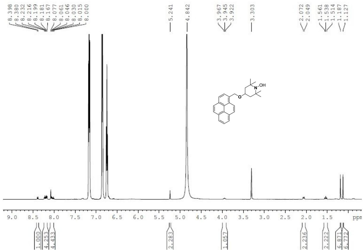
**Fig. S12** 600 MHz <sup>1</sup>H NMR spectrum of Py-CH<sub>2</sub>-O-TEMPOH after reduction of Py-CH<sub>2</sub>-O-TEMPO (**5**) by phenyl hydrazine in CD<sub>3</sub>OD.
