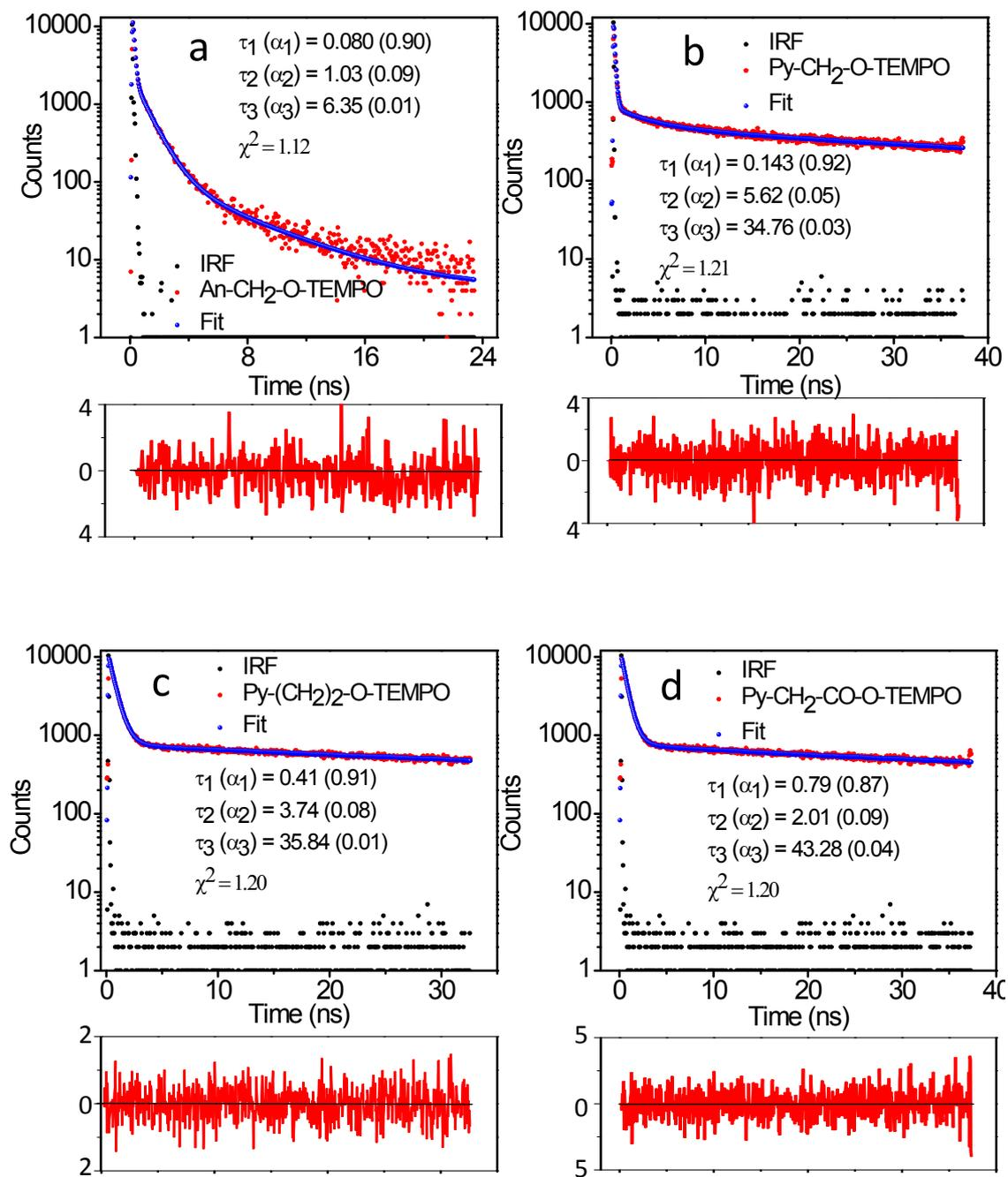
**Fig. S7** Representative time-resolved fluorescence signals and their fits to a sum of multiexponentials. Plots of weighted residuals are shown below each panel. An-CH<sub>2</sub>-O-TEMPO (a), Py-CH<sub>2</sub>-O-TEMPO (b), Py-(CH<sub>2</sub>)<sub>2</sub>-O-TEMPO (c) and Py-CH<sub>2</sub>-CO-O-TEMPO (d) in nitrogen-saturated *n*-hexane at room temperature. Concentration: 20  $\mu$ M.
