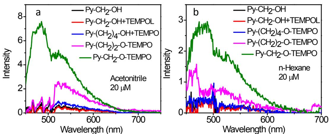
**Fig. S2** Fluorescence emissions spectra of Py-CH<sub>2</sub>-OH, Py-CH<sub>2</sub>-OH+TEMPOL, Py-(CH<sub>2</sub>)<sub>4</sub>-O-TEMPO, Py-(CH<sub>2</sub>)<sub>2</sub>-O-TEMPO and Py-CH<sub>2</sub>-O-TEMPO at  $\lambda_{\text{ex}} = 450$  nm (a) in acetonitrile (a) and *n*-hexane (b), after subtraction of Raman lines. Concentration: 20 μM.
