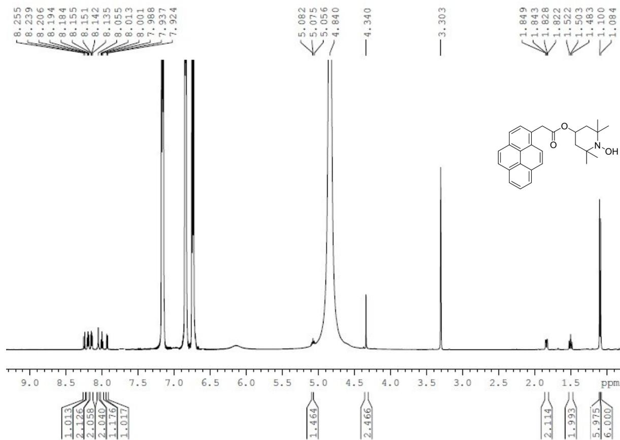
**Fig. S17** 600 MHz <sup>1</sup>H NMR) spectrum of Py-CH<sub>2</sub>-CO-O-TEMPOH after reduction of Py-CH<sub>2</sub>-CO-O-TEMPO (**10**) by phenyl hydrazine in CD<sub>3</sub>OD.
