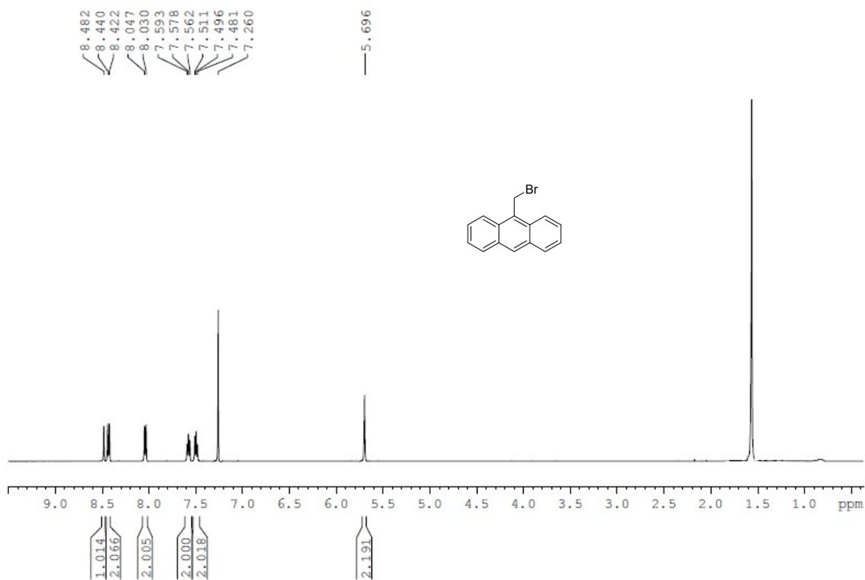
**Fig. S8** 600 MHz <sup>1</sup>H NMR spectrum of An-CH<sub>2</sub>-Br (**1**) in CDCl<sub>3</sub>.
