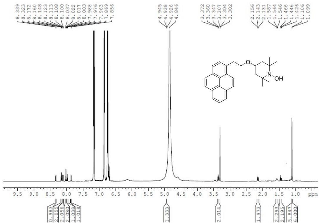
**Fig. S16** 600 MHz <sup>1</sup>H NMR spectrum of Py-(CH<sub>2</sub>)<sub>2</sub>-O-TEMPOH after reduction of Py-(CH<sub>2</sub>)<sub>2</sub>-O-TEMPO (**9**) by phenyl hydrazine in CD<sub>3</sub>OD.
