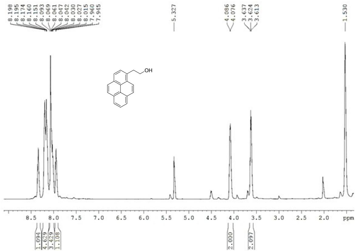
**Fig. S14** 500 MHz <sup>1</sup>H NMR spectrum of Py-(CH<sub>2</sub>)<sub>2</sub>-OH (7) in CD<sub>2</sub>Cl<sub>2</sub>.
