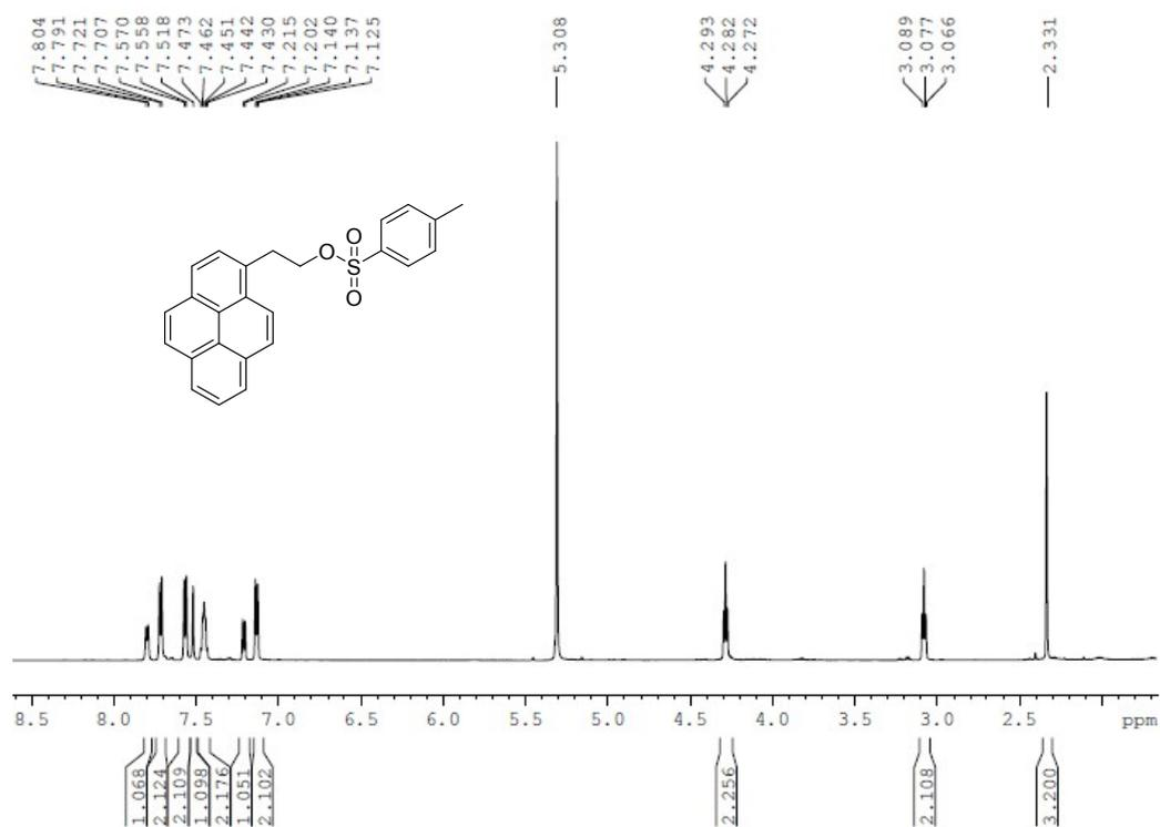
**Fig. S15** 600 MHz <sup>1</sup>H NMR spectrum of Py-(CH<sub>2</sub>)<sub>2</sub>-OTs (**8**) in CD<sub>2</sub>Cl<sub>2</sub>.
