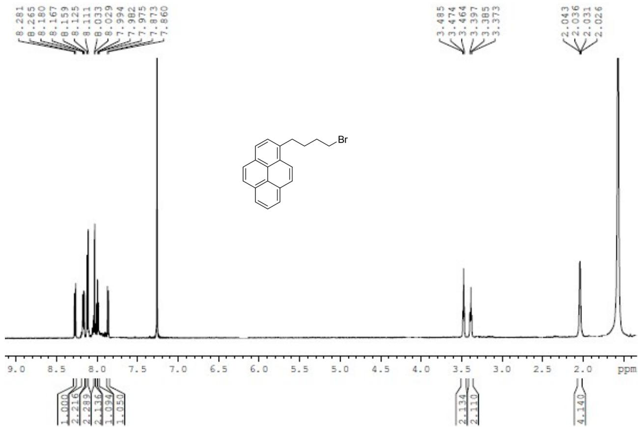
**Fig. S11** 600 MHz <sup>1</sup>H NMR spectrum of Py-(CH<sub>2</sub>)<sub>4</sub>-Br (**4**) in CDCl<sub>3</sub>.
