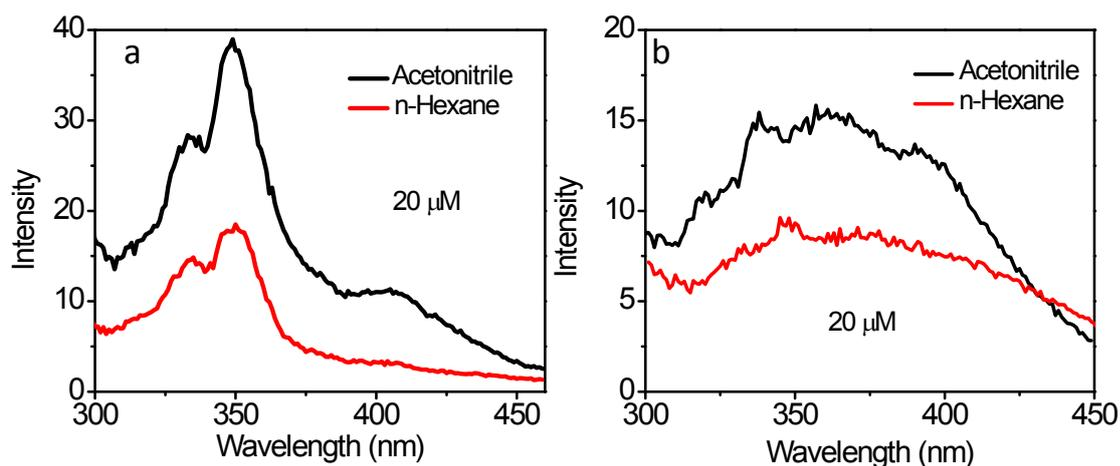
**Fig. S4** Fluorescence excitation spectra of Py-CH<sub>2</sub>-O-TEMPO (a) and Py-CH<sub>2</sub>-CO-O-TEMPO (b), in *n*-hexane and in acetonitrile, recorded at  $\lambda_{em} = 450$  nm. Concentration: 20  $\mu$ M.
