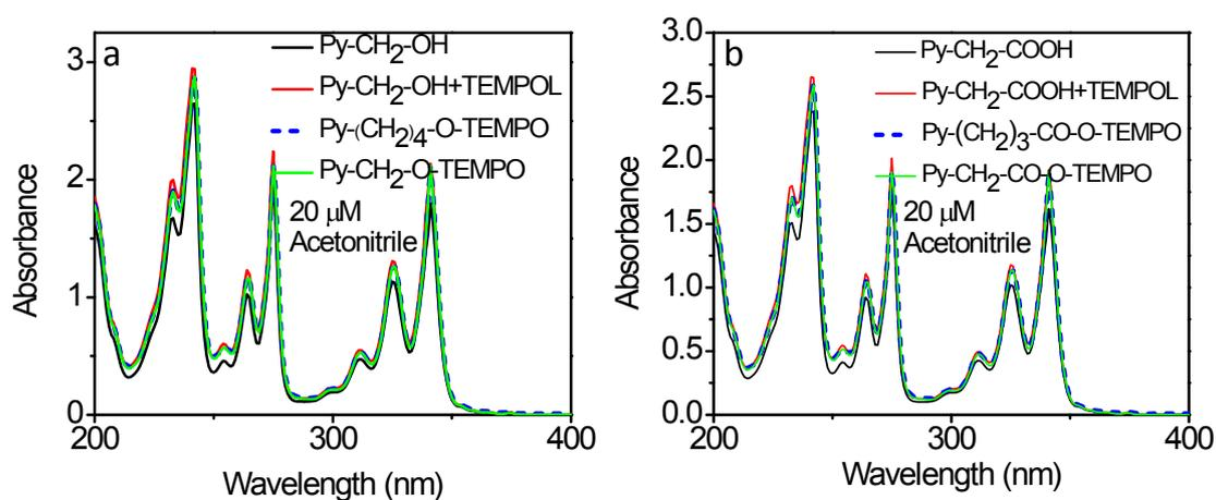
**Fig. S5** Absorption spectra of Py-CH<sub>2</sub>-OH, Py-CH<sub>2</sub>-OH+TEMPOL (1:1), Py-(CH<sub>2</sub>)<sub>4</sub>-O-TEMPO, Py-CH<sub>2</sub>-O-TEMPO (a), and Py-CH<sub>2</sub>-OOH and Py-CH<sub>2</sub>-COOH+TEMPOL (1:1), Py-(CH<sub>2</sub>)<sub>3</sub>-O-TEMPOL and Py-CH<sub>2</sub>-CO-O-TEMPOL (b) in acetonitrile. Concentration: 20  $\mu$ M.
