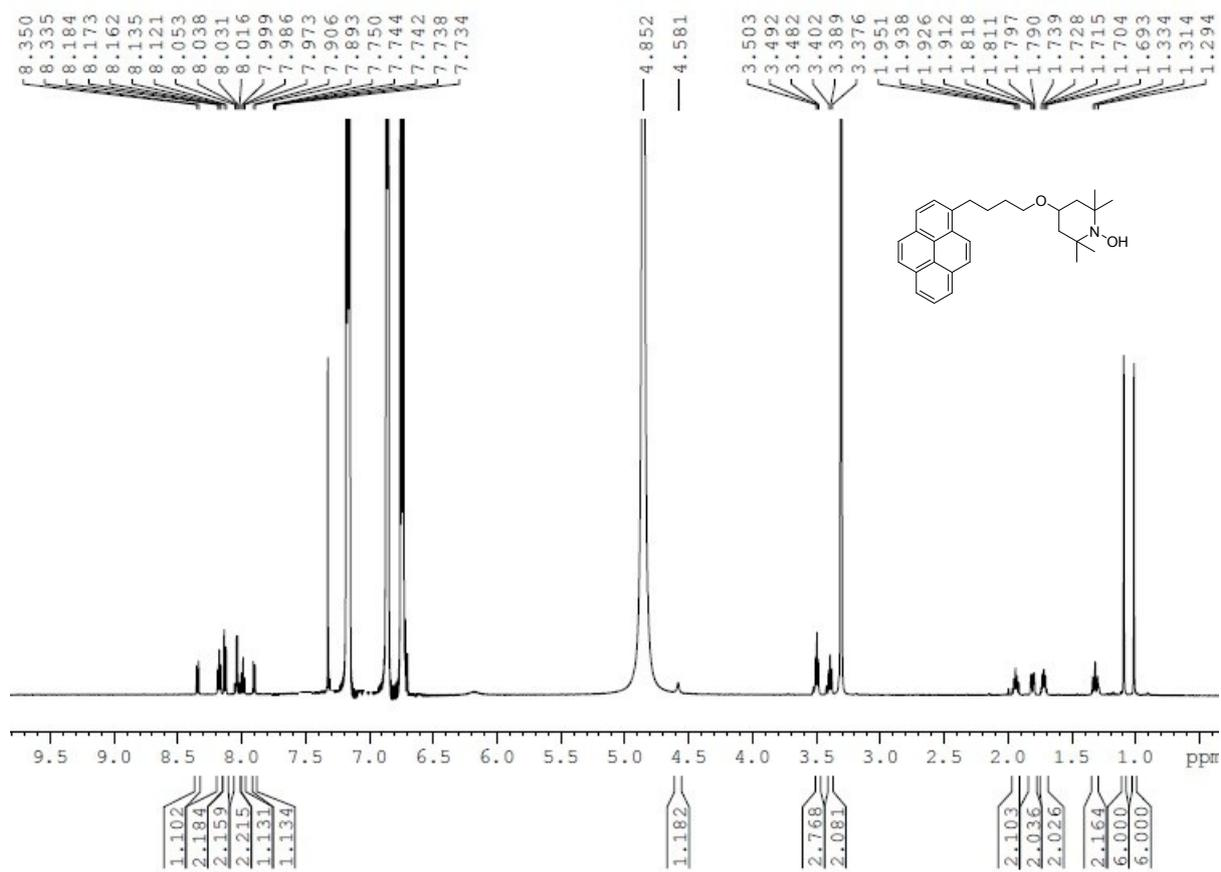
**Fig. S13** 600 MHz <sup>1</sup>H NMR spectrum of Py-(CH<sub>2</sub>)<sub>4</sub>-O-TEMPOH after reduction of Py-(CH<sub>2</sub>)<sub>4</sub>-O-TEMPO (**6**) by phenyl hydrazine in CD<sub>3</sub>OD.
