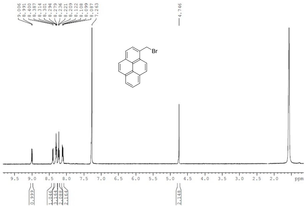
**Fig. S10** 600 MHz  $^1\text{H}$  NMR spectrum of Py-CH<sub>2</sub>-Br (**3**) in CDCl<sub>3</sub>.
