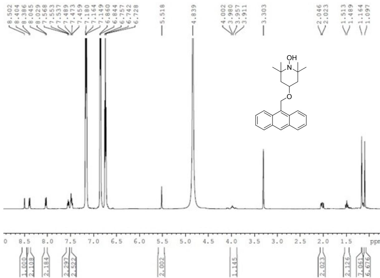
**Fig. S9** 600 MHz <sup>1</sup>H NMR spectrum of An-CH<sub>2</sub>-O-TEMPOH after reduction of An-CH<sub>2</sub>-O-TEMPO (**2**) by phenyl hydrazine in CD<sub>3</sub>OD.
