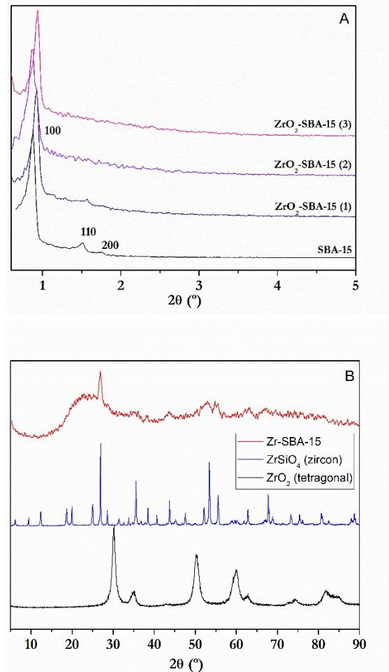
**Figure ESI-1.** (A) Low-angle, and (B) wide angle powder XRD patterns of ZrO<sub>2</sub>-SBA-15, and t-ZrO<sub>2</sub>, zircon, and Zr-SBA-15 reference materials.
