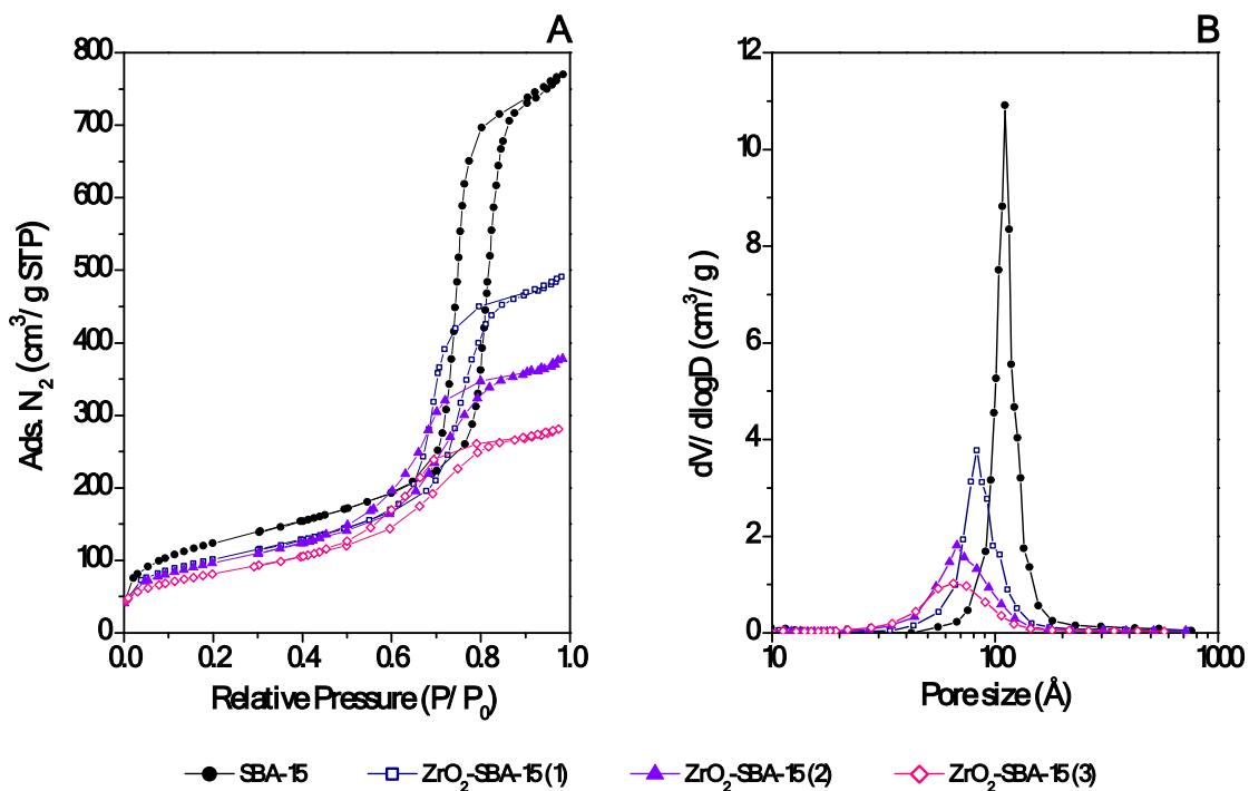
**Figure ESI-2.** (A)  $N_2$  adsorption-desorption isotherms, and (B) corresponding BJH- pore size distributions for  $ZrO_2$ -SBA-15 and parent SBA-15 materials.
