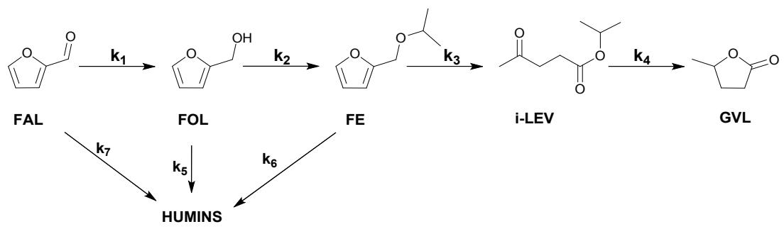
**Scheme ESI-1** Proposed reaction network for the transformation of furfural in alcohol media over  $\text{ZrO}_2$ -grafted SBA-15. FAL, furfural; FOL, furfuryl alcohol; FE, isopropyl furfuryl ether; i-LEV, isopropyl levulinate; GVL,  $\gamma$ -valerolactone; HUMINS, degradation product
