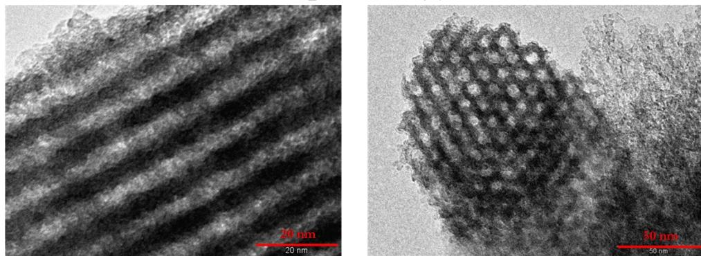
**Figure ESI-3.** TEM images of ZrO<sub>2</sub>-SBA-15 and parent SBA-15 materials.
