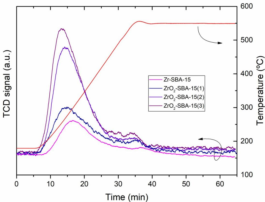
**Figure ESI-5.**  $\text{NH}_3$  TPD profiles for Zr- and  $\text{ZrO}_2$ -SBA-15 materials.
