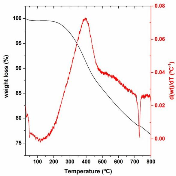
**Fig ESI-9.** TG analysis curves recorded for sample ZrO<sub>2</sub>-SBA-15 used during 3 consecutive reutilization cycles in the cascade transformation of furfural to GVL. Reaction conditions: 170 °C; 7 h; furfural:2-propanol=1:50 (by mols); furfural:catalyst=2.5:1 (by mass).
