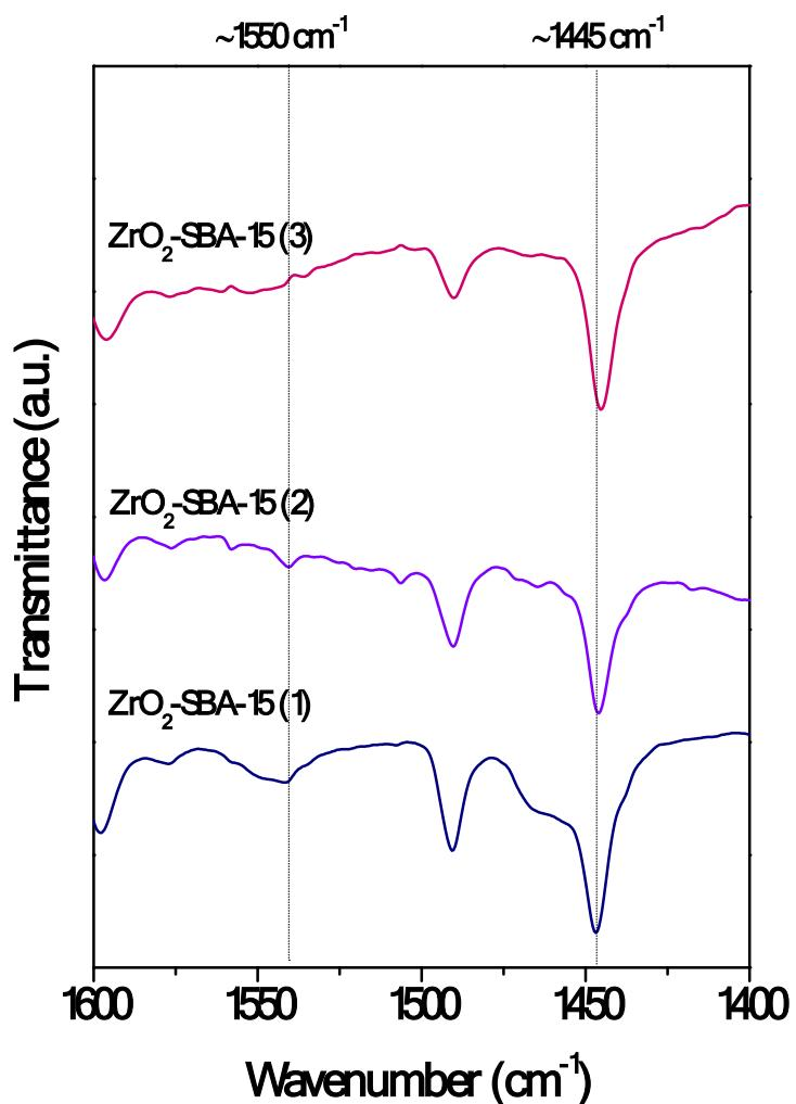
**Figure ESI-6.** DRIFT spectra of adsorbed pyridine on  $\text{ZrO}_2$ -coated SBA-15.
