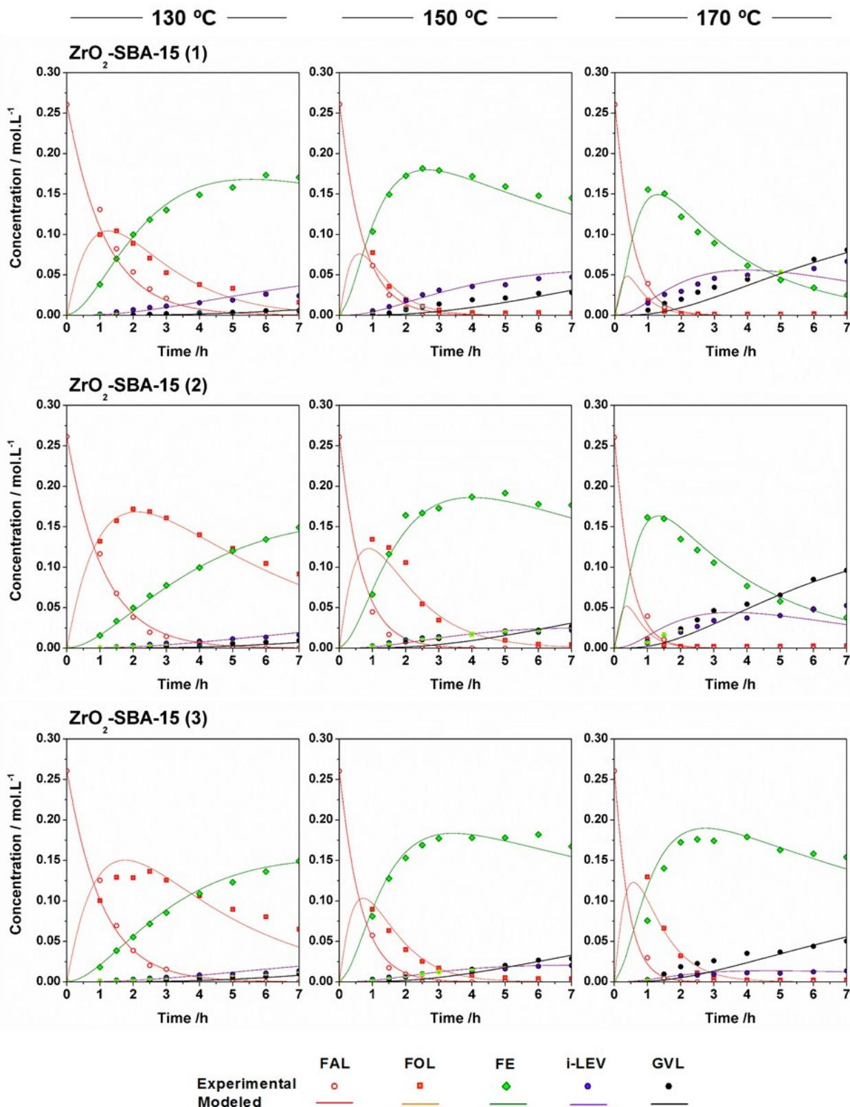
**Figure ESI-8.** Experimental (symbol) and modelled (solid lines) products concentration for furfural transformation to GVL in 2-propanol over ZrO<sub>2</sub>-SBA-15 catalysts. Reaction conditions: furfural:2-propanol=1:50 (by mols); furfural:catalyst=2.5:1 (by weight).
