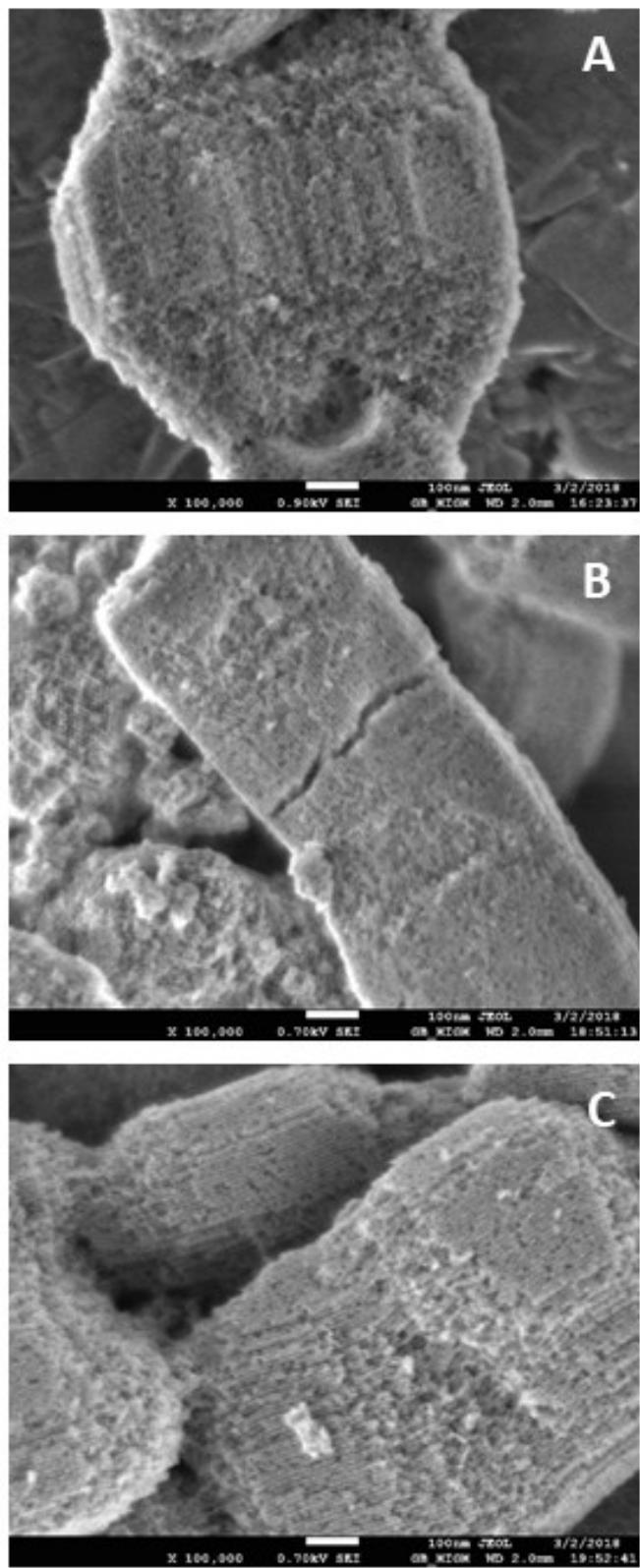
**Figure ESI-4.** SEM images of (A)  $\text{ZrO}_2$ -SBA-15(1), (B)  $\text{ZrO}_2$ -SBA-15(2), and (C)  $\text{ZrO}_2$ -SBA-15(3) materials.
