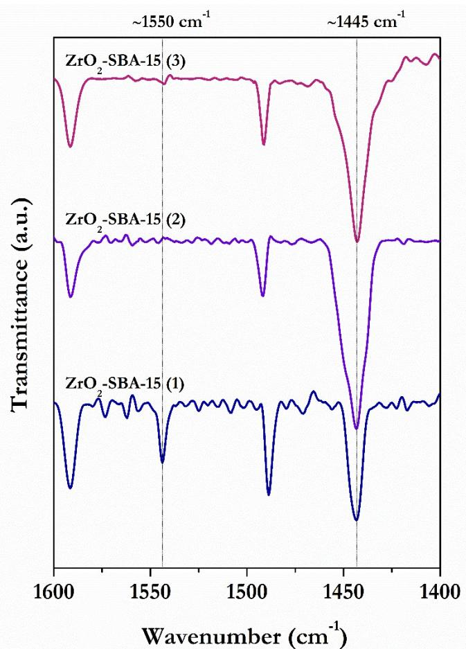
**Figure ESI-7.** ATR-IR spectra of adsorbed pyridine on  $\text{ZrO}_2$ -coated SBA-15 in i-PrOH.
